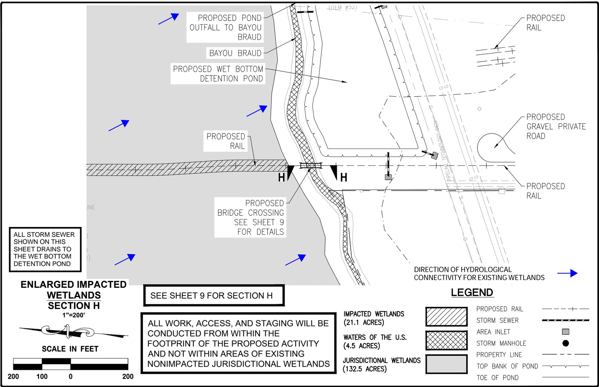
ALL STORM SEWER SHOWN ON THIS SHEET DRAINS TO THE WET BOTTOM DETENTION POND
