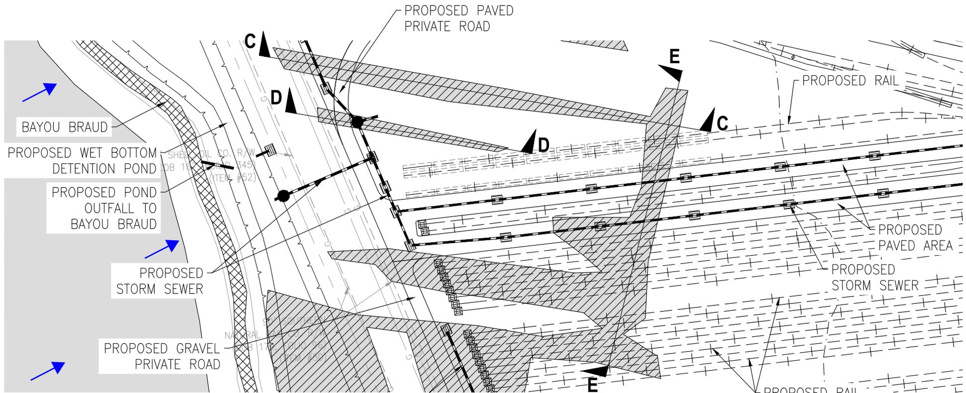
ALL STORM SEWER SHOWN ON THIS SHEET DRAINS TO THE WET BOTTOM DETENTION POND
