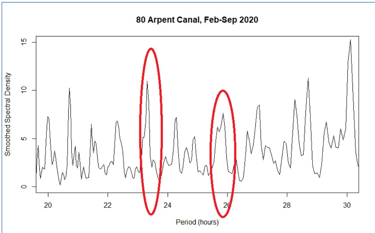
Figure 5: Water levels recorded in the 80 Arpent Canal exhibiting more prominent peaks corresponding to 24 and 26 hours
