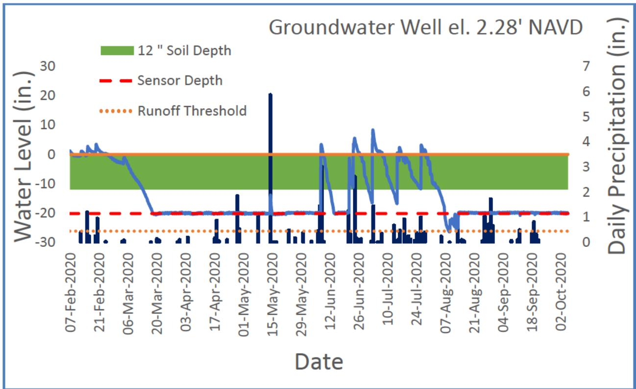
Figure 6: Groundwater well readings relative to the soil surface recorded in the project area and daily precipitation recorded at Thibodaux 4 SE.
