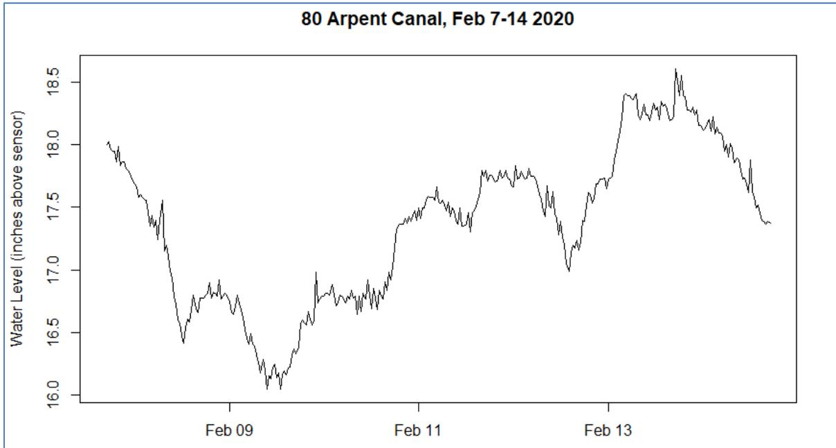
Figure 4: Water levels recorded in the 80 Arpent Canal exhibiting small daily fluctuations consistent with tidal influence.
