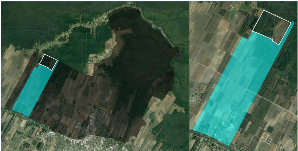
***Figure 3: The calculated watershed containing the project area is shaded black in the left image. The area assumed to contribute runoff to the project area is shaded in blue.***
