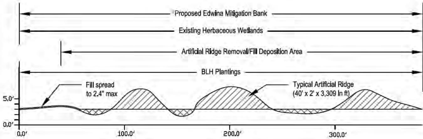
Section G-G: Existing Artificial Ridge to be Removed
