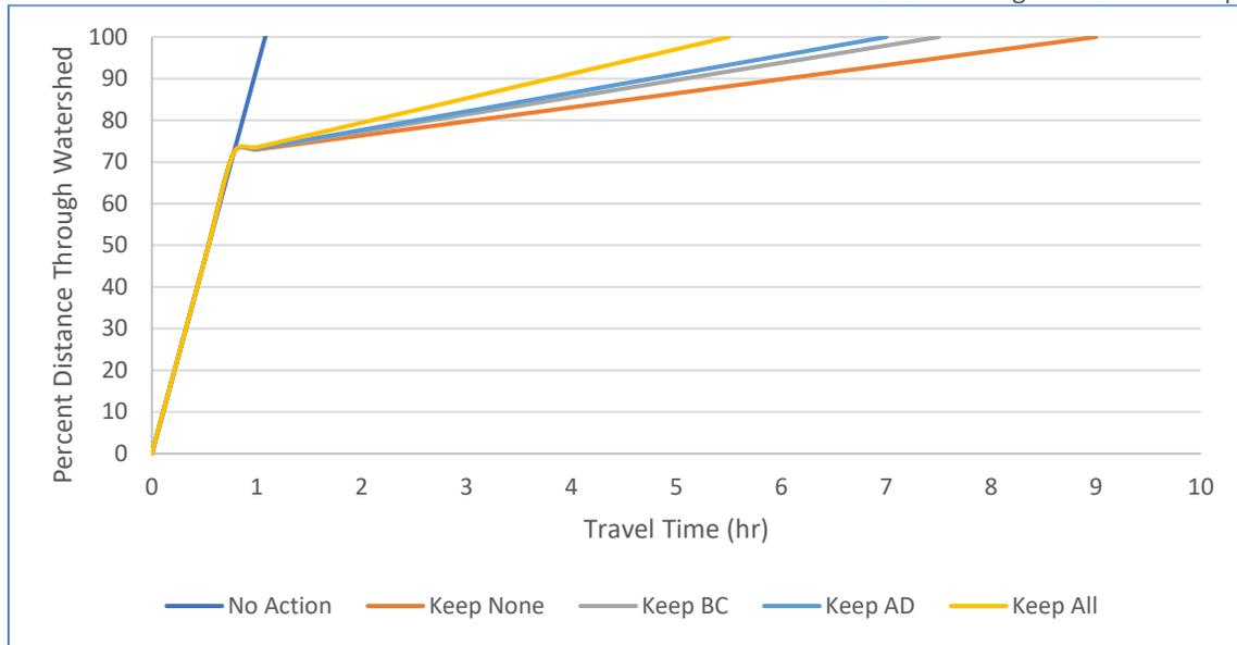
**Figure 14: Comparison of travel rates through watershed, expressed as percent distance from upslope watershed boundary to 80 Arpent Canal. Inflection point indicates property boundary.**
