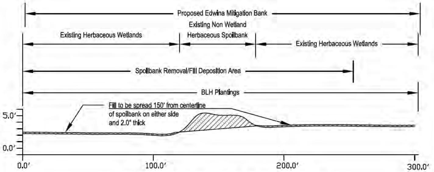
Section D-D': Existing Spoilbank within Crawfish Pond to be Removed
