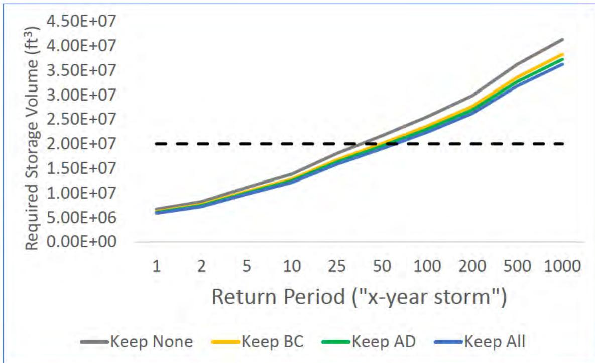
Figure 17: Calculated detention volumes required to avoid flooding after 24-hour rainfall events across return periods for all design alternatives. Horizontal dashed line indicates estimated volume of project area below 5 ft.
