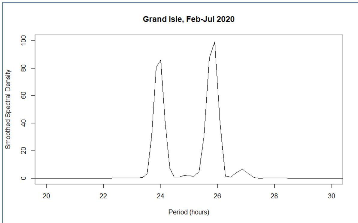
Figure 1: Periodogram for the water level recorded at Grand Isle for the period of record identical to that of the data collected at the project site.
