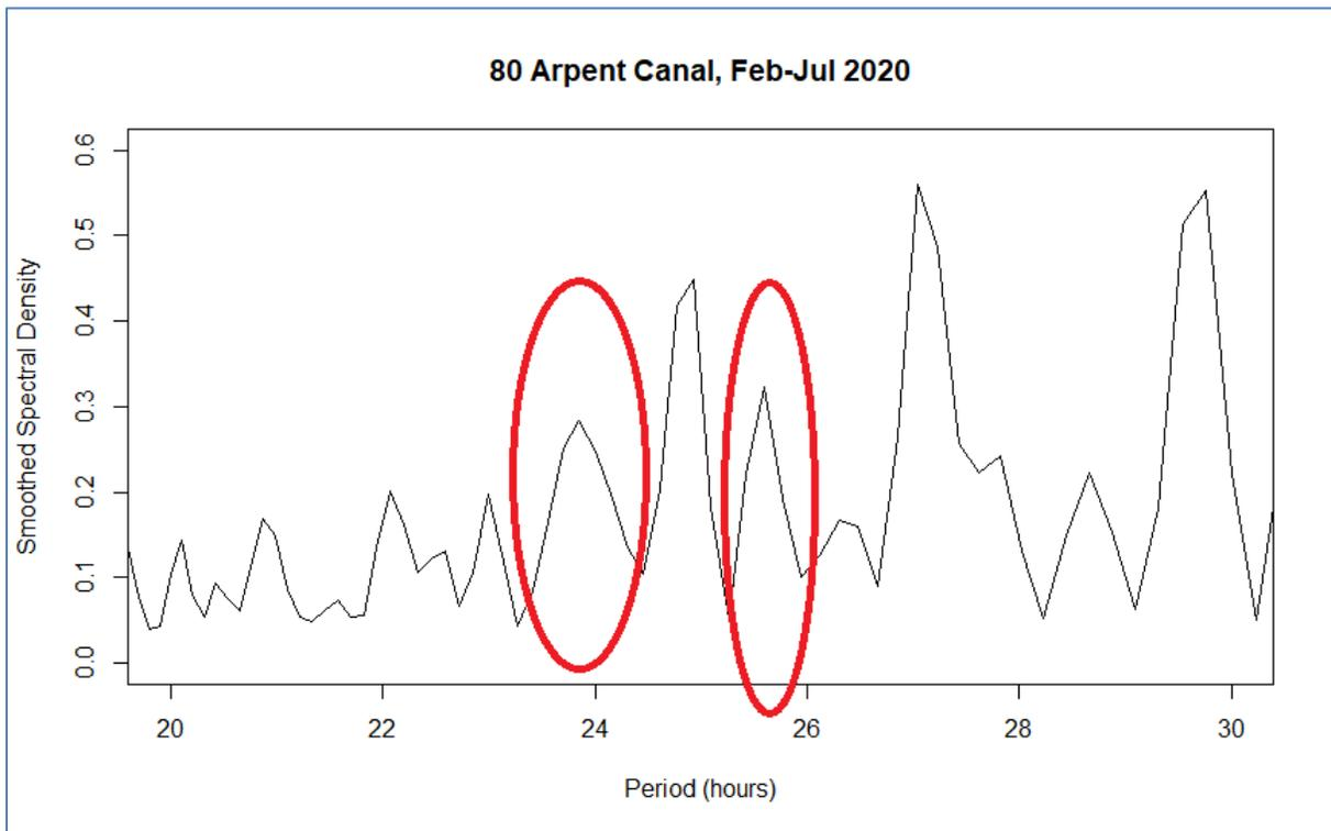
Figure 3: Water levels recorded in the 80 Arpent Canal exhibiting small peaks corresponding to 24 and 26 hours
