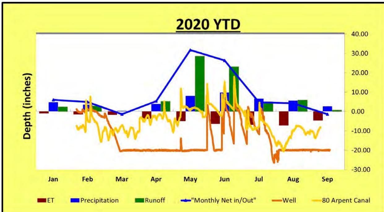
Figure 10: Calculated hydrograph for January through September 2020, and water levels recorded at project site between February-September 2020. Both sets of water levels are relative to ground level at groundwater well (elevation 2.28' NAVD 88)
