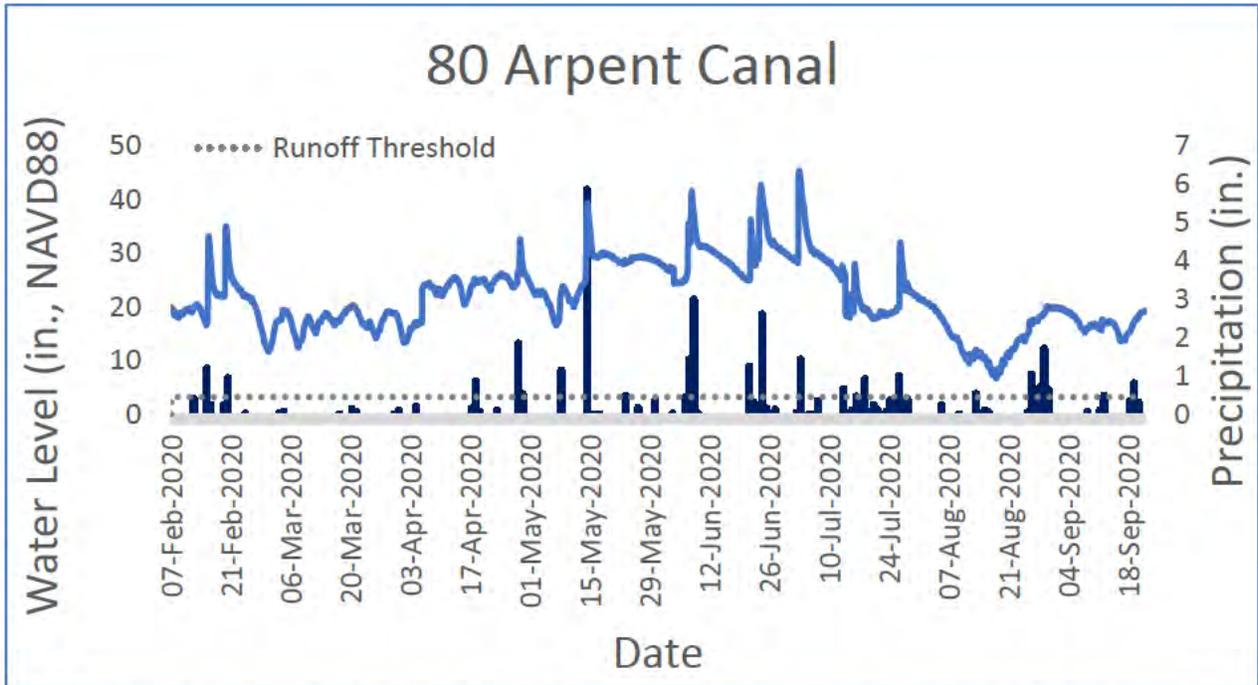
Figure 4: Water levels recorded in the 80 Arpent Canal and daily precipitation totals recorded at Thibodaux 4 SE.
