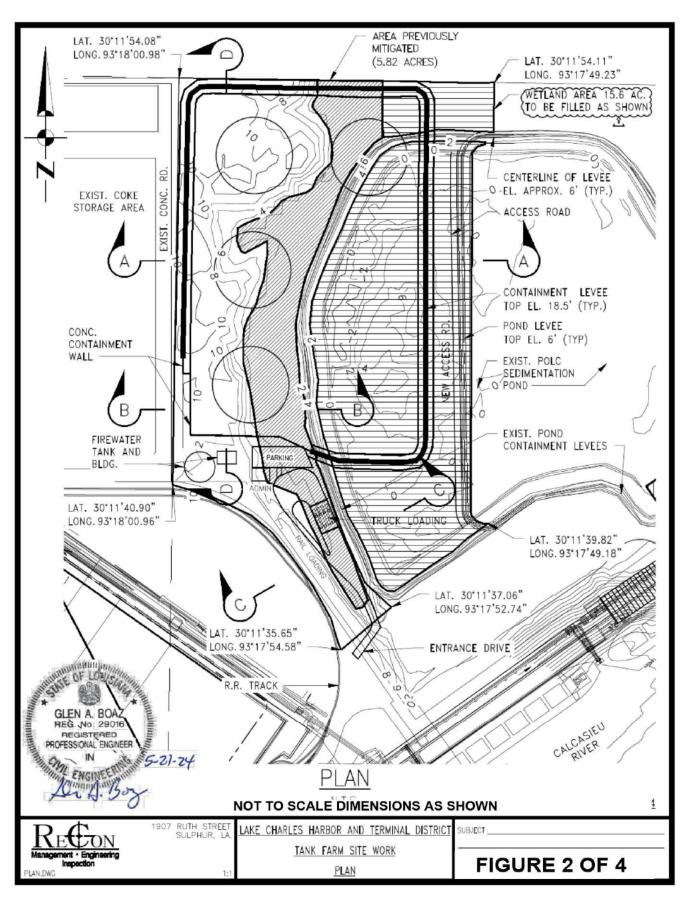
Total Earthen Fill: 248,300 cubic yds Total Concrete: 800 cubic yds
