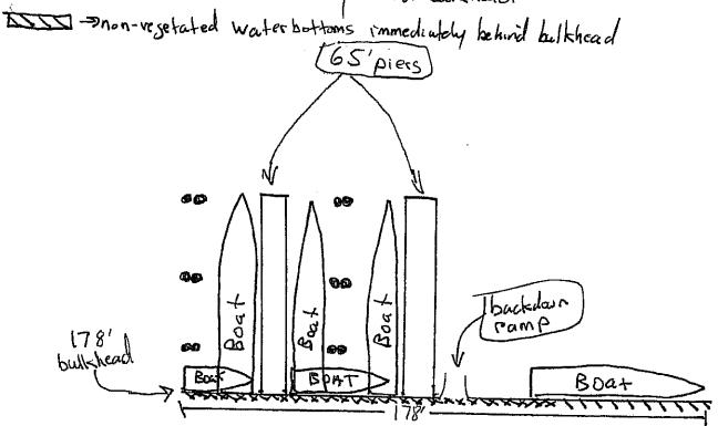
\* oyster boats will be loaded /unloaded along the entire length of the bulkhead
