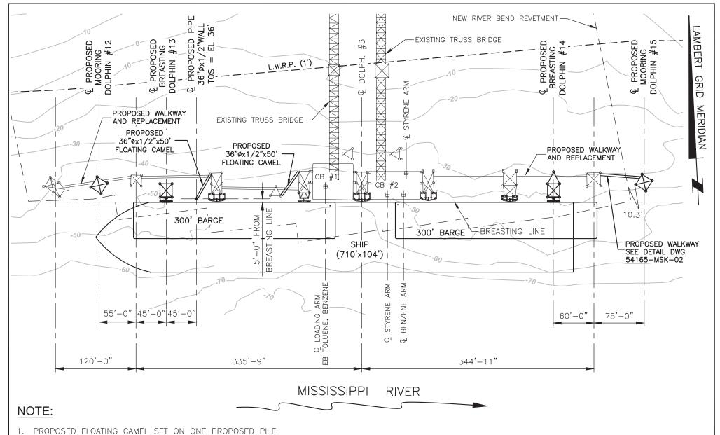
AND CONNECTED TO EXISTING PILES ON A RIDING TRACK CONNECTION. INSTALL FOR FLOATING DEBRIS DEFLECTION.
