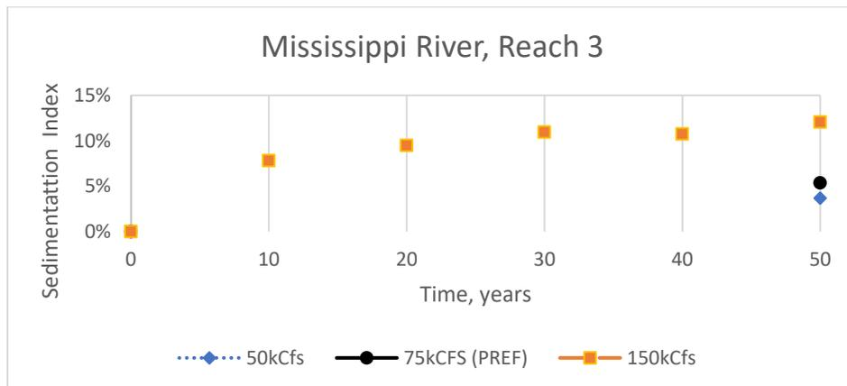
**Figure 6. Basinwide Model Sedimentation Index for Reach 3 of the Mississippi River (1 Mile Below Structure) under Three Diversion Rates.** Note the range of values on the y axis differs between figures.
