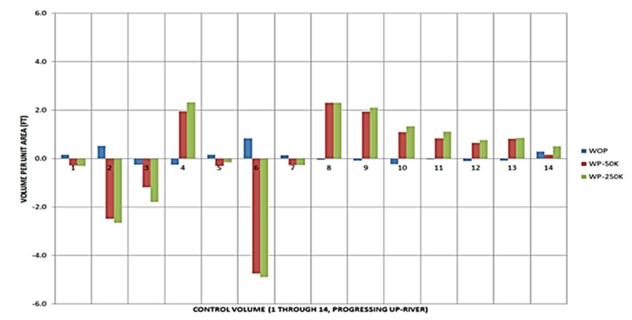
**Figure 9. LMR Bed Elevation Change by Control Volume: 2008-2010 Hydrograph, Without Future Relative Sea-level Rise.** ‘WOP’ = without diversions; ‘WP-50k’ = with upper-Breton (250,000 cfs), mid-Breton (5,000 cfs), lower-Breton (50,000 cfs), lower-Barataria (50,000 cfs) and MBSD at 50,000 cfs; ‘WP-250k’ = same as ‘WP-50k’ but with MBSD at 250,000 cfs. This is Figure 5.10 from Brown et al. (2018 draft).
