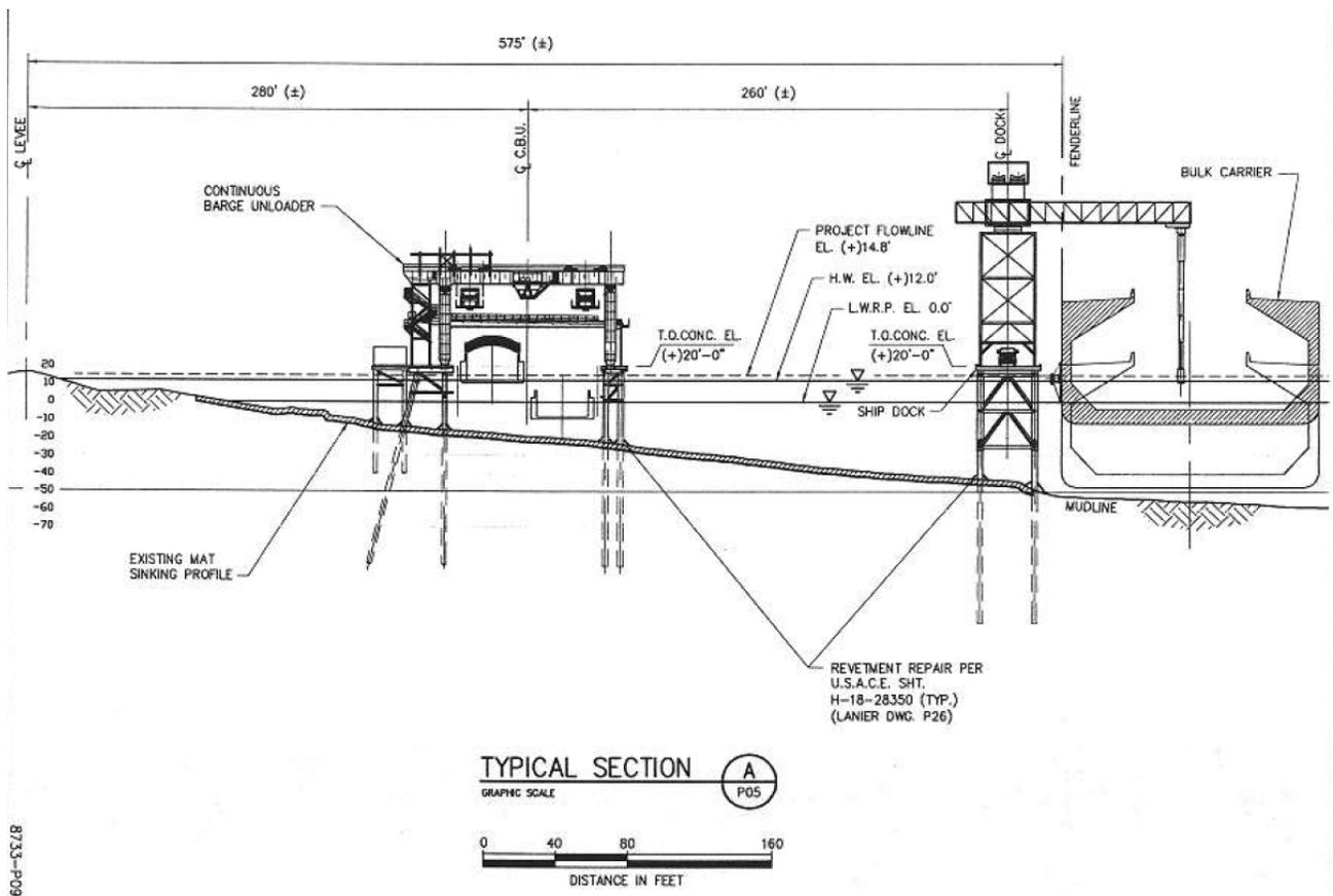
**Figure 35. Riverward Extent of the Previously Permitted Ram Coal Export Facility to the Proposed Mid-Barataria Sediment Diversion Project. Based on the estimated distance from the low water reference plane into the river, the fenderline of the dock would extend 425 ft into the river and an additional 140 ft bulk carrier beam width would result in a total of 565 ft of occupied river space.**
