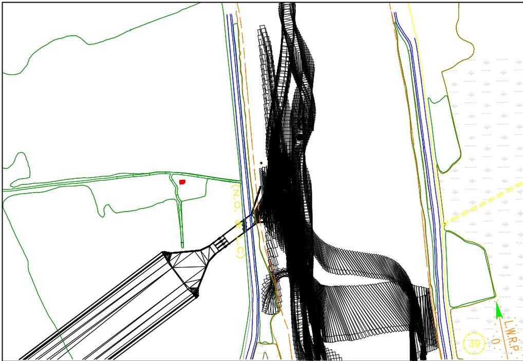
**Figure 26: Composite Trackline of Tows Passing Close to Operating Diversion Pilots Noting Effect on Tow of Operating Diversion, Closest Approach <300 ft 1,000,000 cfs River Flow, SE or ENE 20-knot Wind**
