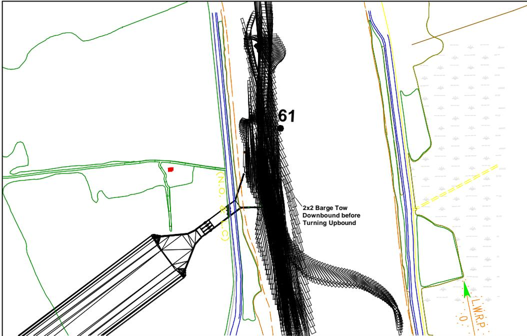
**Figure 25: Composite Trackline of Tows Passing Close to Operating Diversion Pilots Noting Effect on Tow of Operating Diversion, Closest Approach <200 ft 600,000 cfs River Flow, SE or ENE 20-knot Wind**
