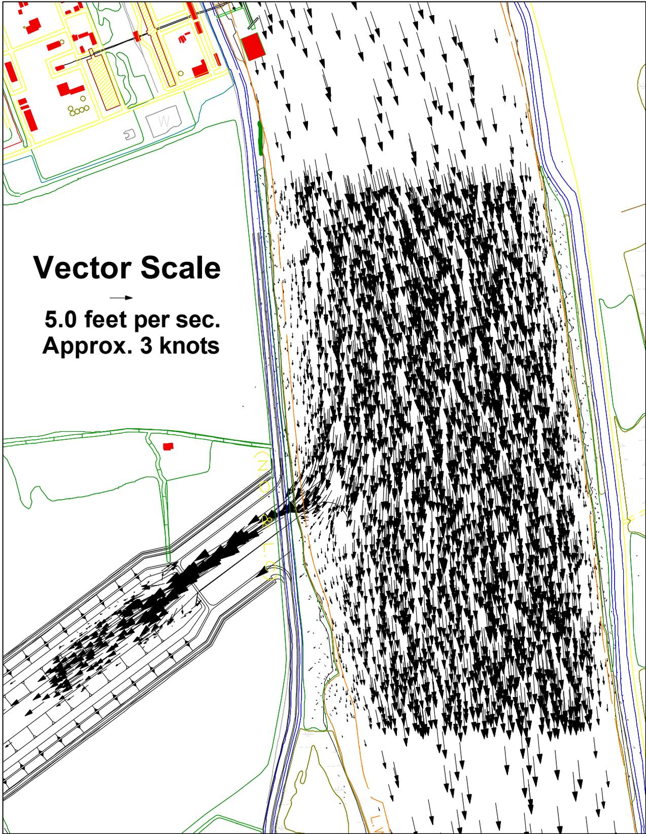
Figure 11: River Current at 975kcf Flow Rate (30ft depth-averaged) (Inset)
