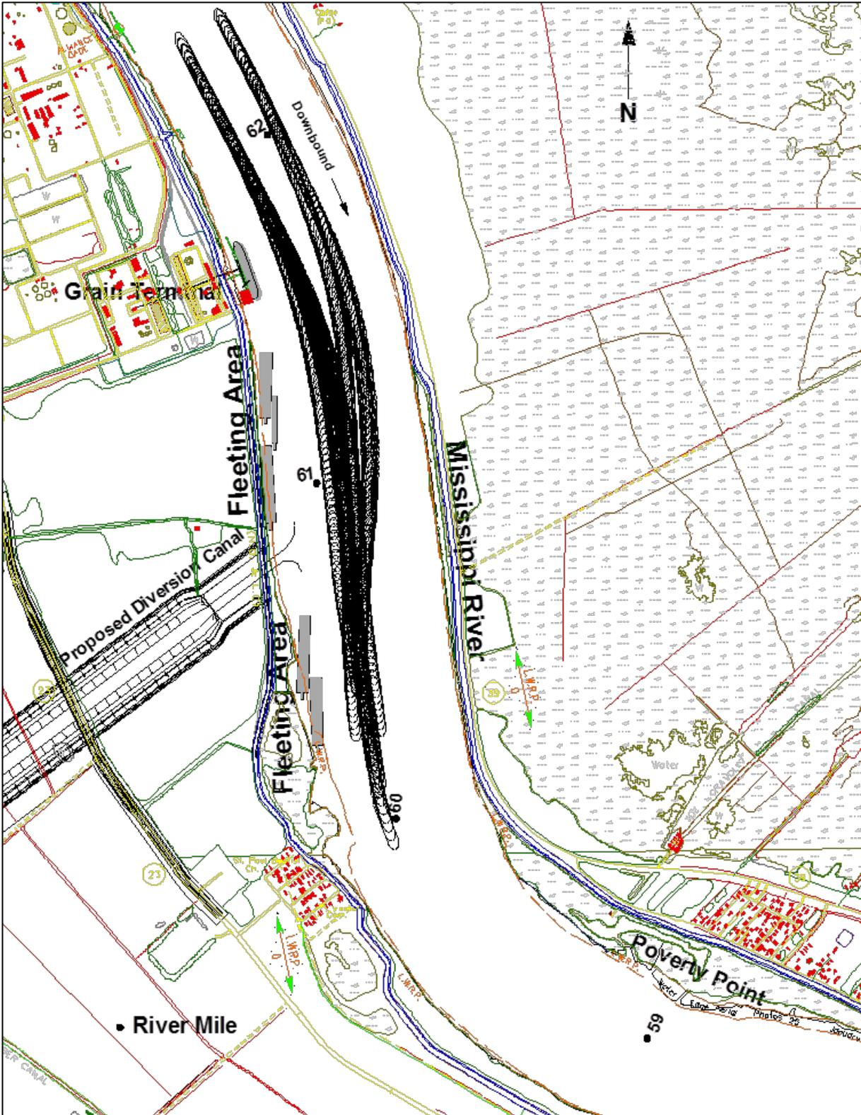
**Figure 13: Downbound Ballasted and Loaded Suezmax Tanker (919ft x 164ft x 33ft/47ft)
