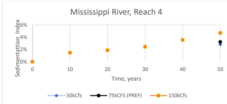
**Figure 7. Delft3D Basinwide Model Sedimentation Index for Reach 4 of the Mississippi River (From 1 Mile Below Structure to Gulf) under Three Diversion Rates.** Note the range of values on the y axis differs between figures.
