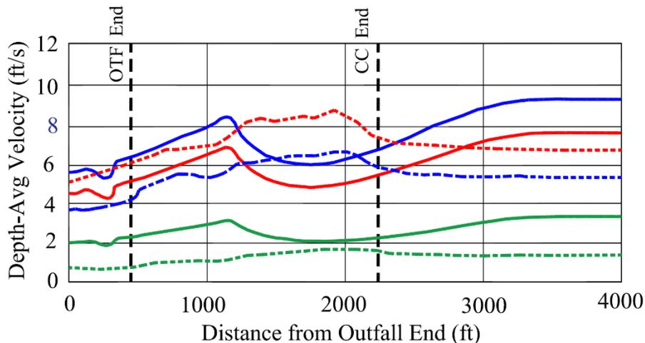
**Figure 6.6-15: Depth-Averaged Velocities in the Outfall section for various model cases**
