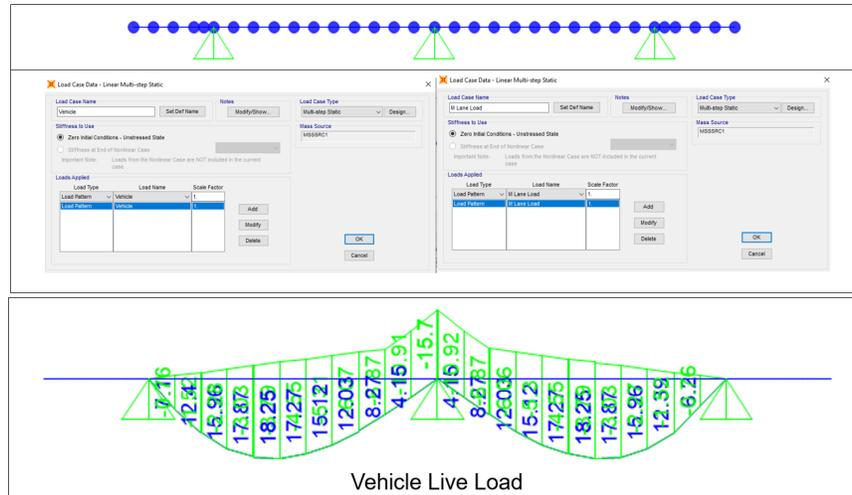
**Figure 5.4-17: An example of a SAP2000 model developed for the deck design and the envelope of the bending moment diagram for the vehicle live load**
