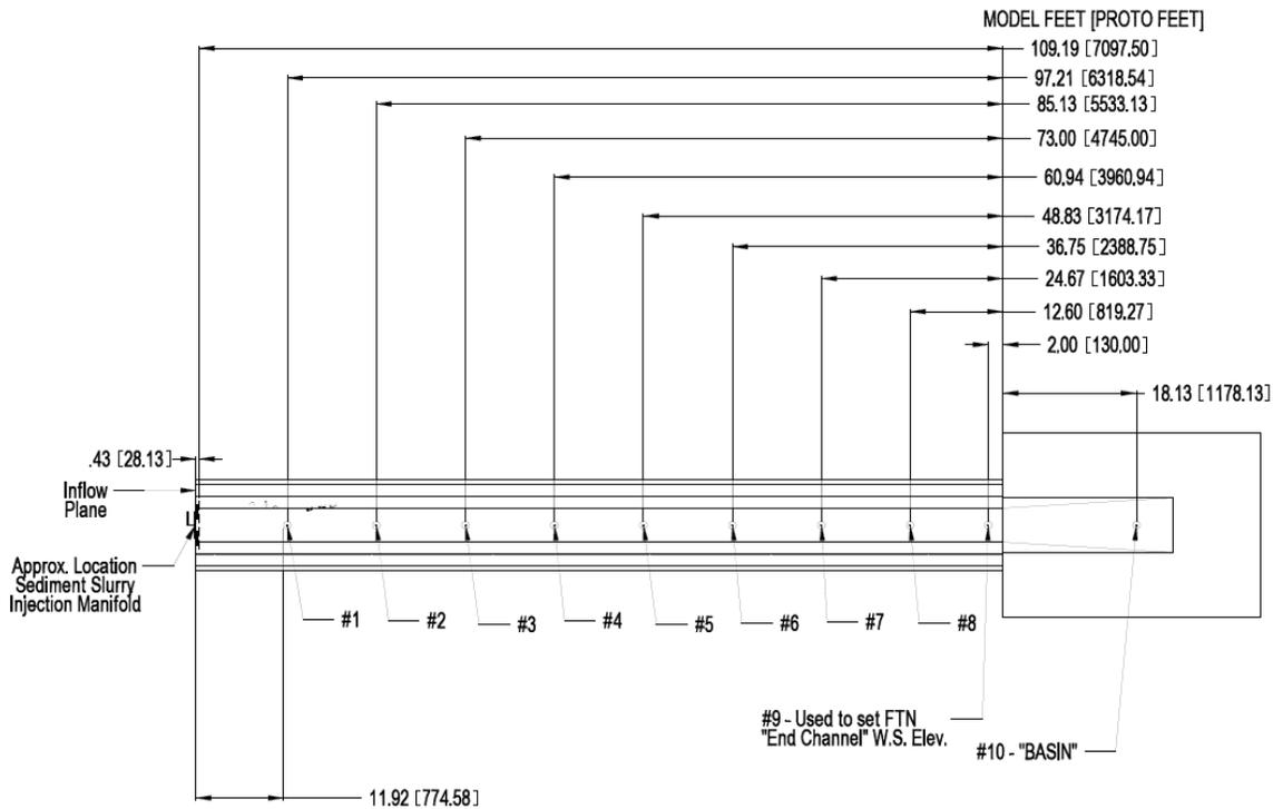
Figure 3.3-4: Location of water level measurements in conveyance channel.
