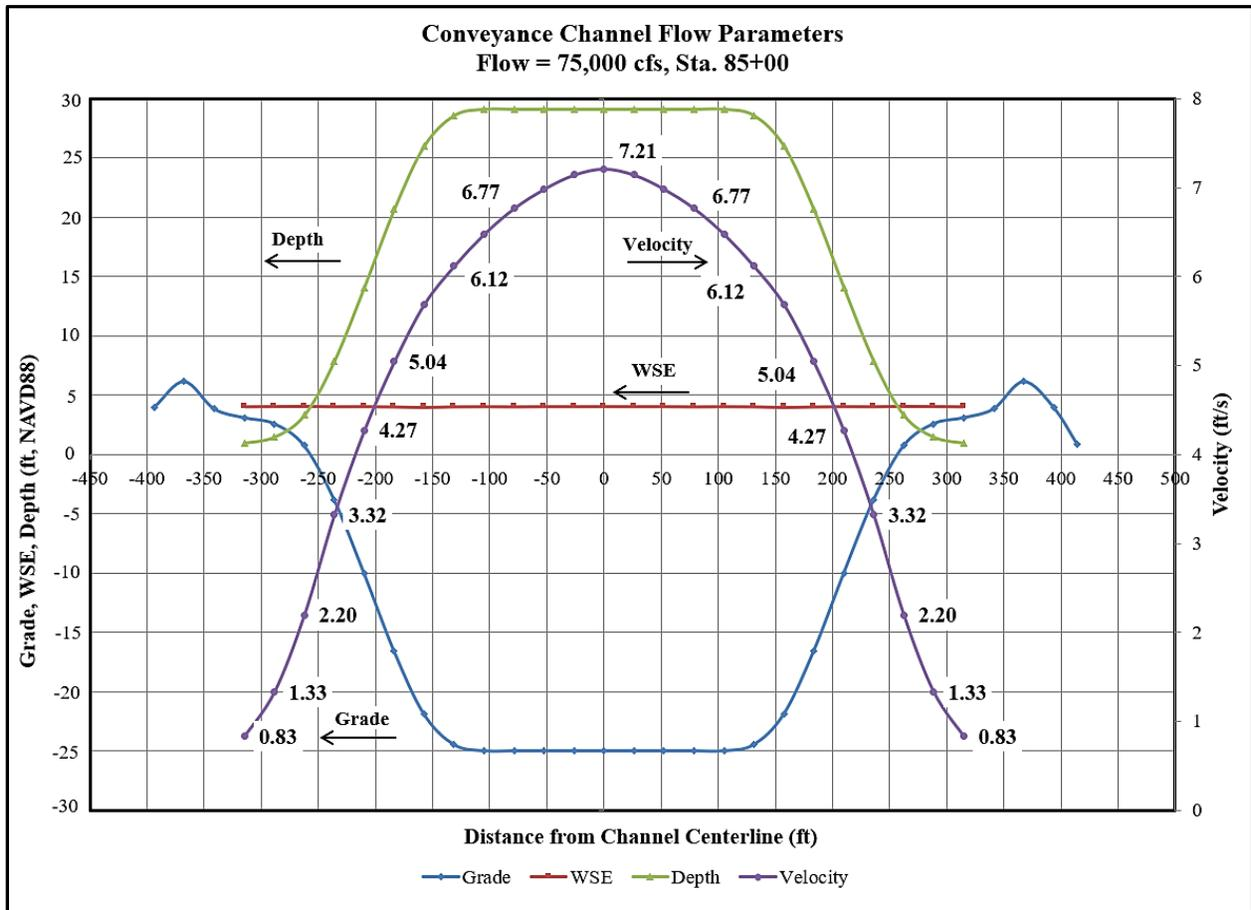
**Figure 6.6-12: Water Surface Elevation, Depth & Velocity at Mid-Channel (Sta 85+00) for Normal Flow Conditions (75,000 cfs) [Velocities are Depth-Averaged Velocities]**
