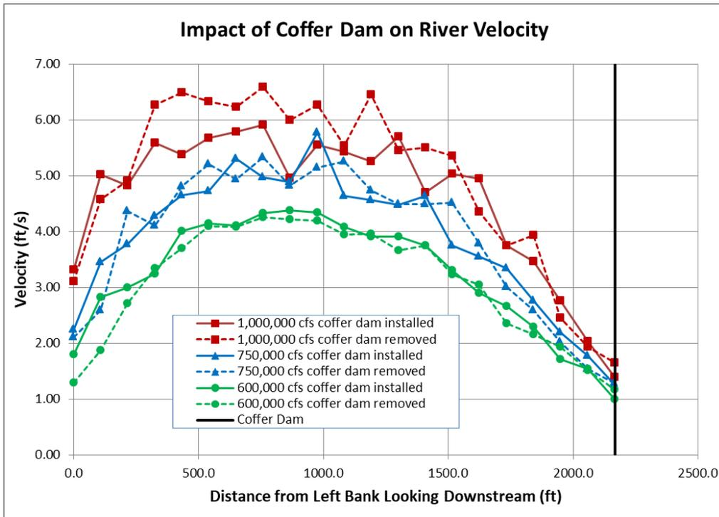
**Figure 3.3-9: Velocity profile with and without cofferdam.**
