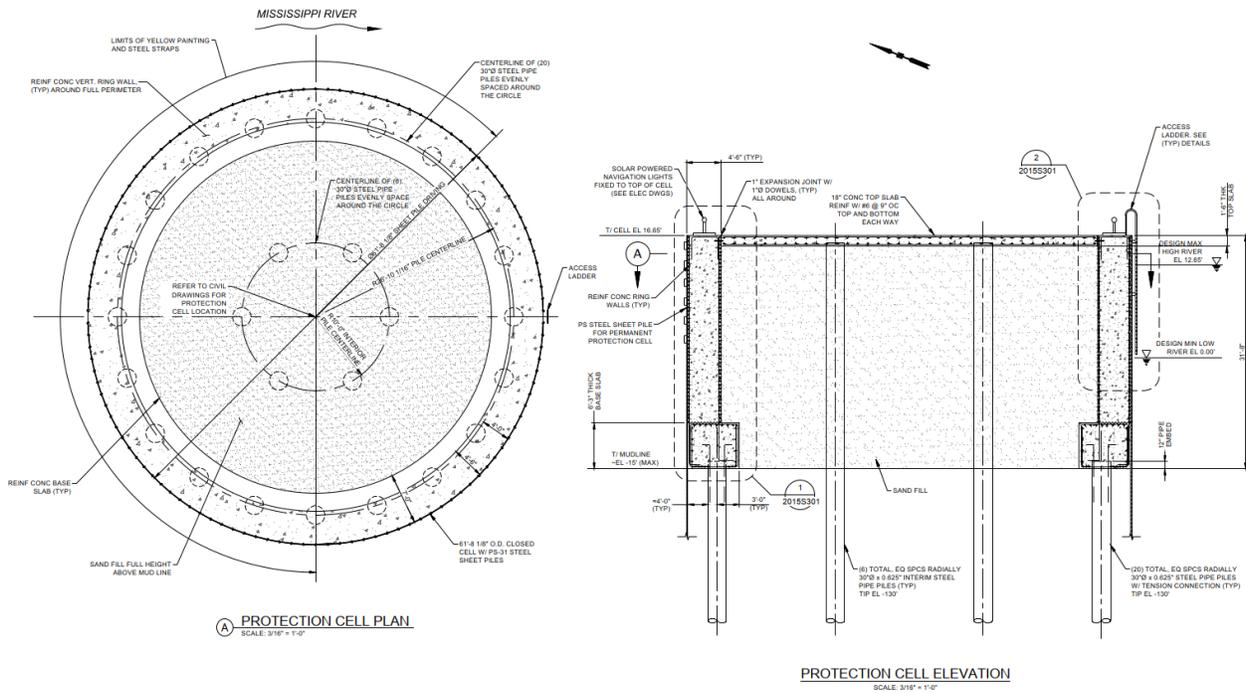
**Figure 5.3-3: Intake Protection Cell Plan and Elevation View**
