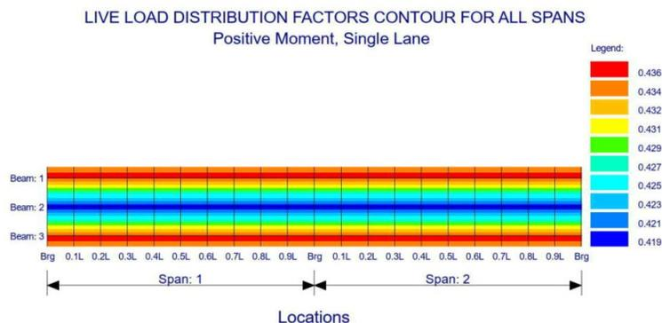
**Figure 5.4-16: An example of live load distribution factor for positive moment**
