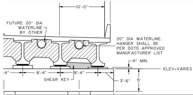
**Figure 6.8-6 – Water Line Detail**
