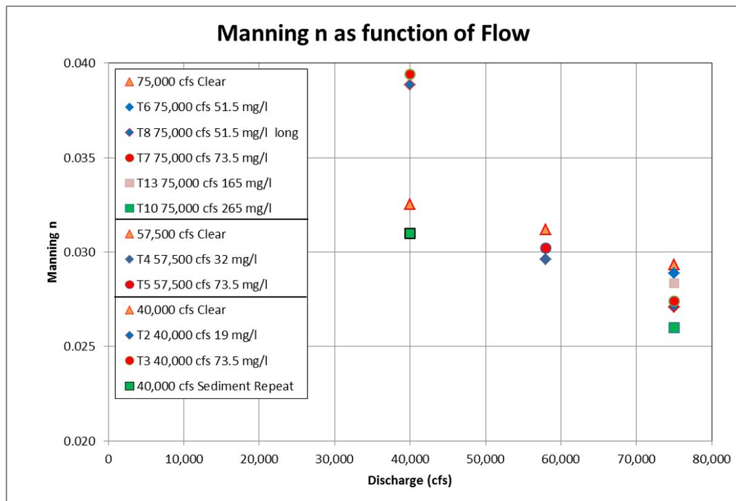
**Figure 3.3-12: Manning's  $n$  as a function of discharge with sediment.**
