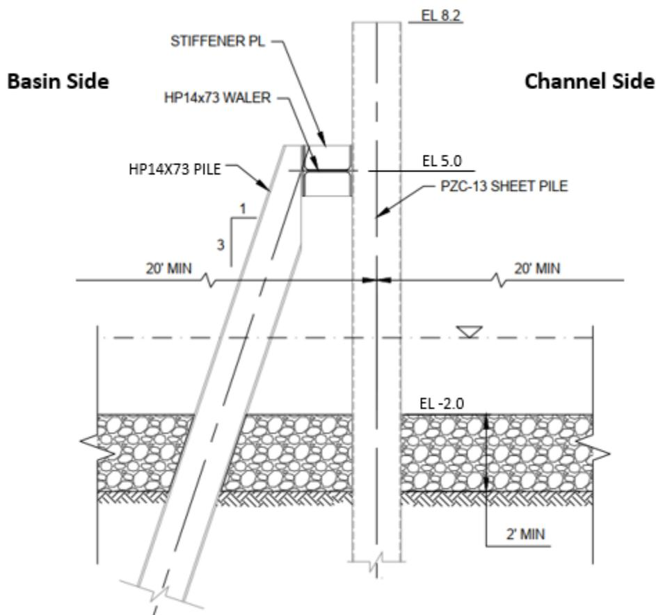
**Figure 5.10-1: OTF Braced Guide Wall Typical Section**
