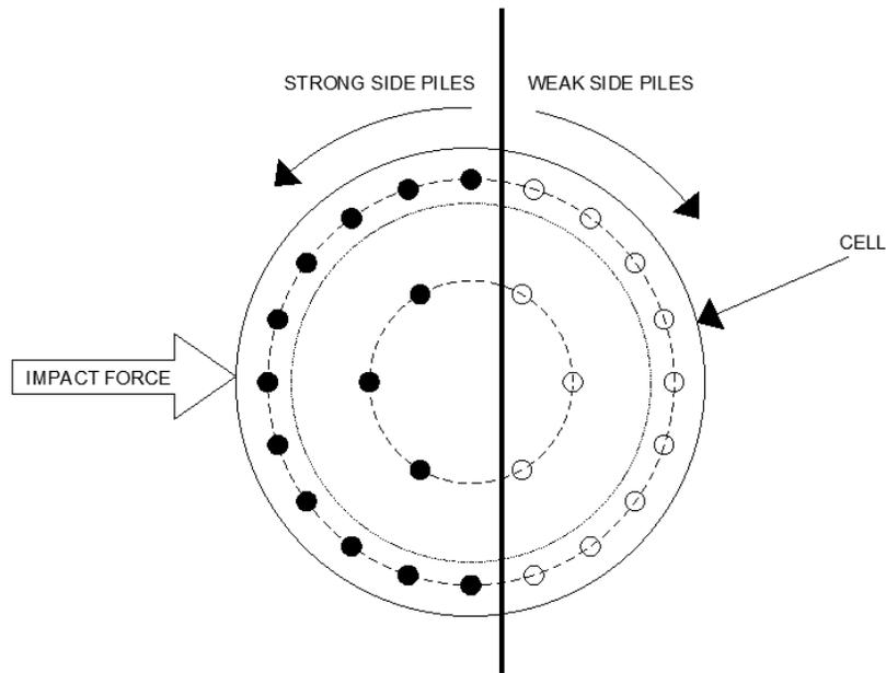
**Figure 5.3-4: Intake Protection Cell Pile Layout**
