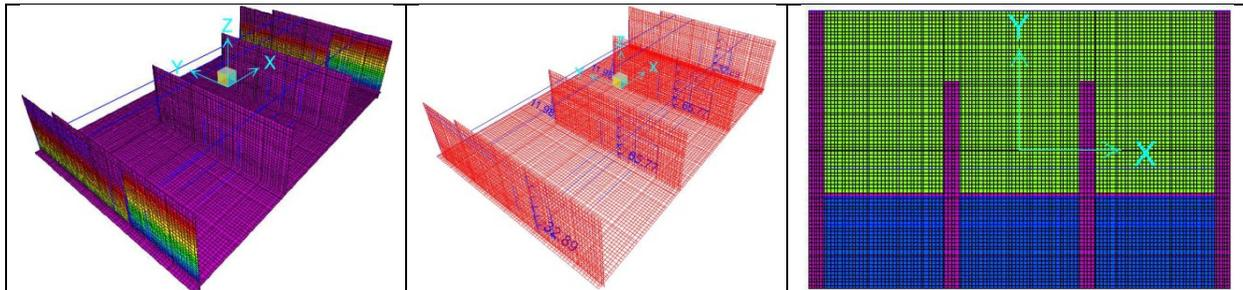
**Figure 5.4-2: An example of applying hydrostatic pressure on walls, gates and slab**
