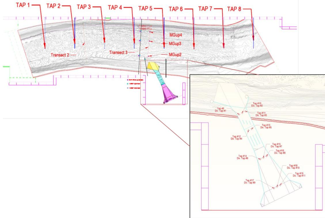
**Figure 3.3-1: Locations where model data was collected in the river model.**
