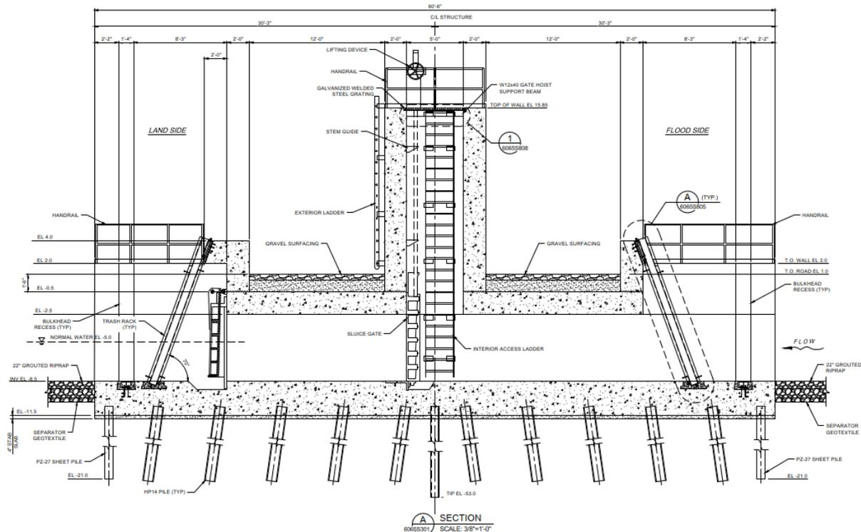
**Figure 5.12-2: Drainage Structure Cross Section**
