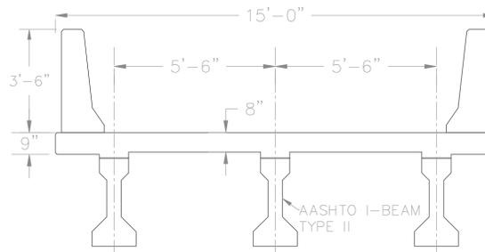
**Figure 5.4-11: Section with 15 ft. width**
