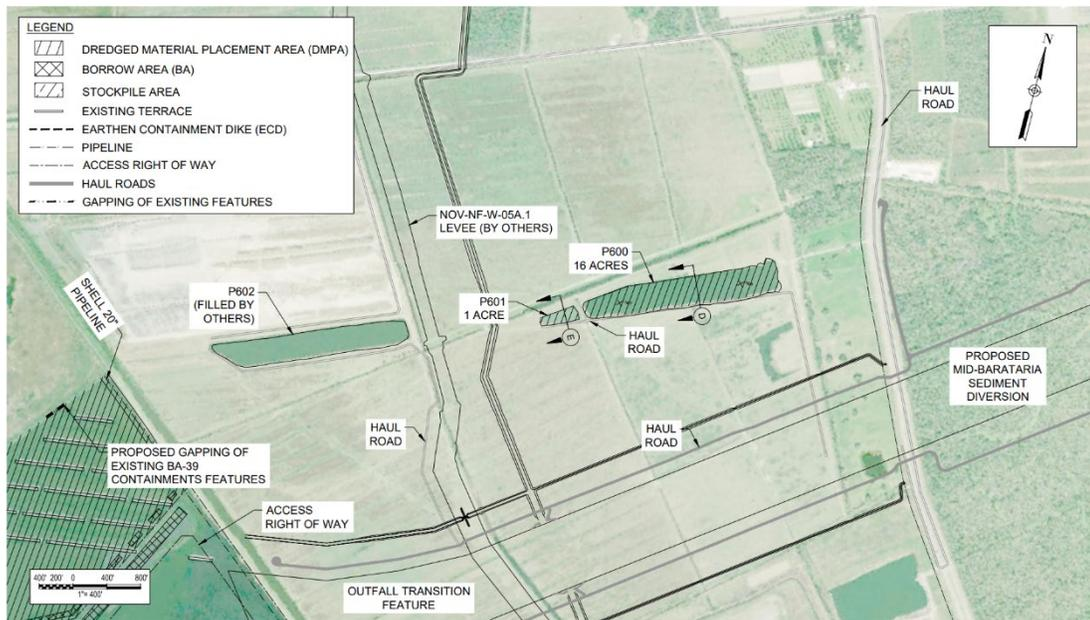
**Figure 6.7-8: Existing Borrow Pits Plan View**
