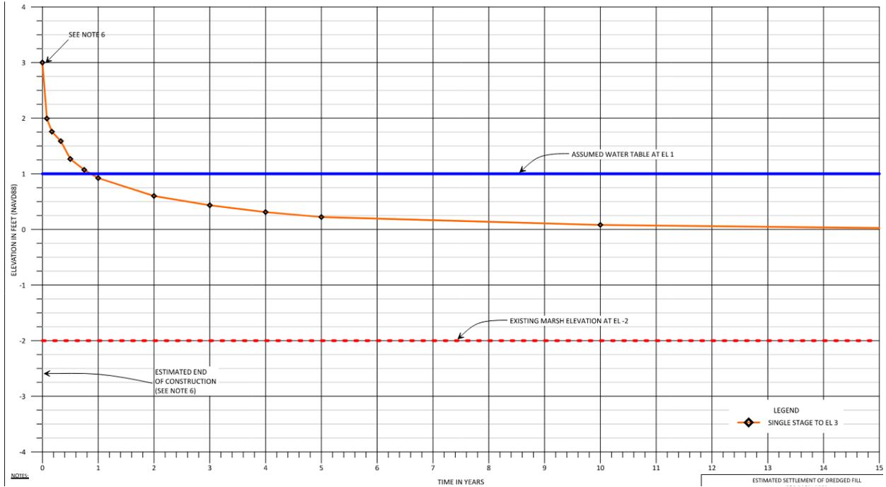
**Figure 6.7-11: Time settlement curve for material fill to +3.0 ft. NAVD88**
