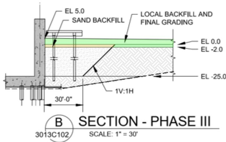
Figure 4.2-4: Compacted Local Backfill – Phase III (View at U-frame and Gated Structure Walls)
