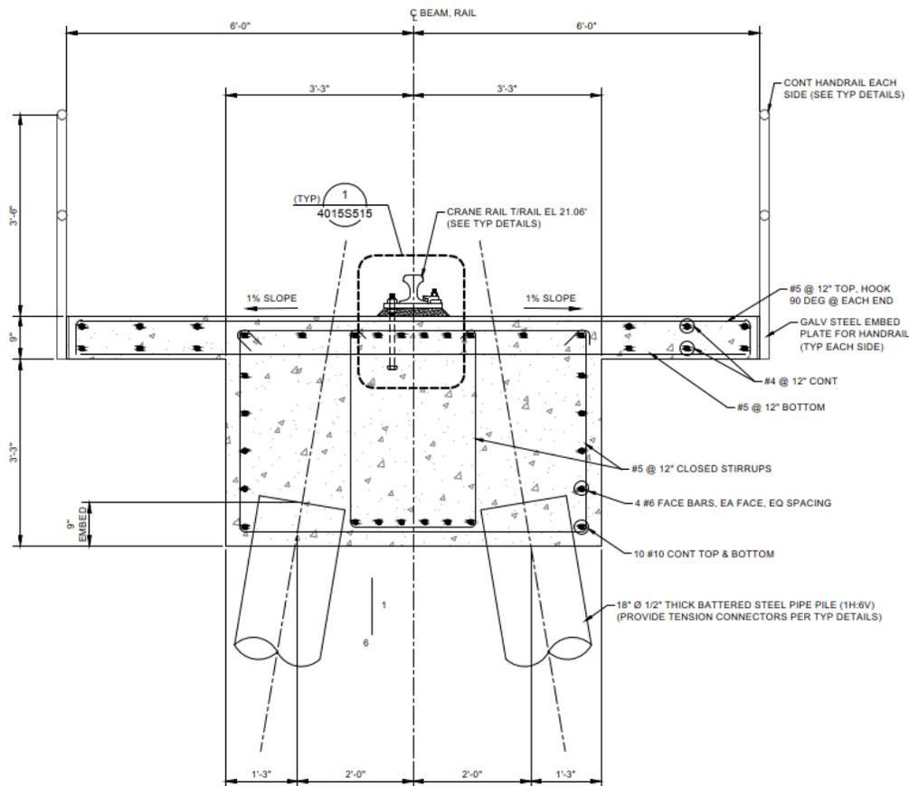
**Figure 5.5-2: Gantry Crane Platform Cross-Section**
