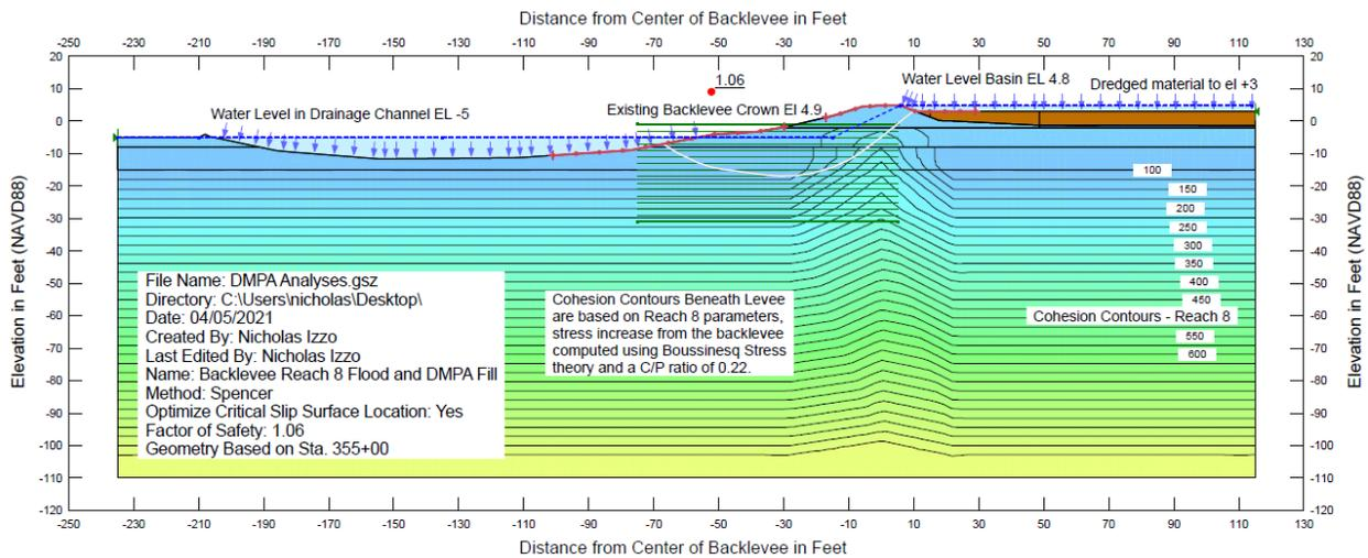
**Figure 6.7-13: Existing back levee slip surface analysis for existing conditions with DMPA fill placed to el 3.0 in the basin**
