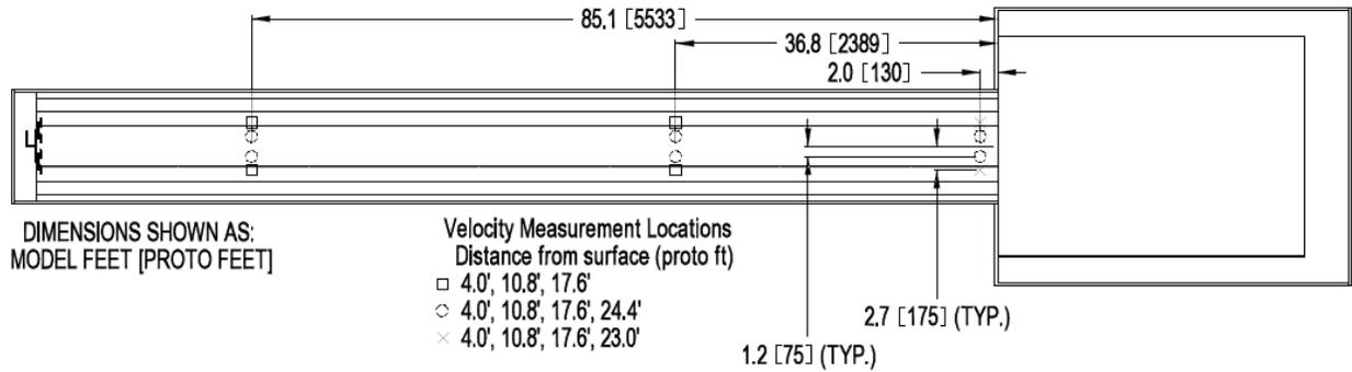
Figure 3.3-3: Location of velocity measurements in conveyance channel.
