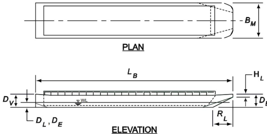
**Figure 5.3-1: Design Barge Tow Plan and Elevation View**
