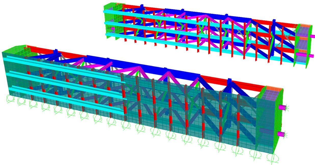
**Figure 5.4-6: 3-D SAP2000 Model of Bulkhead Gate**
