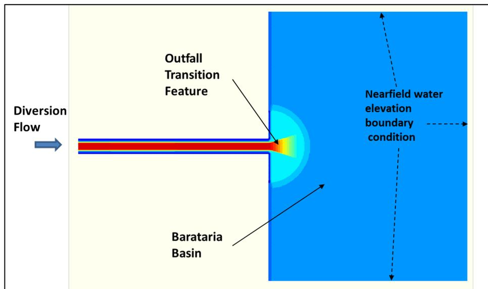
**Figure 3.2-4: Delft3D Model Domain for Conveyance Channel Analysis**
