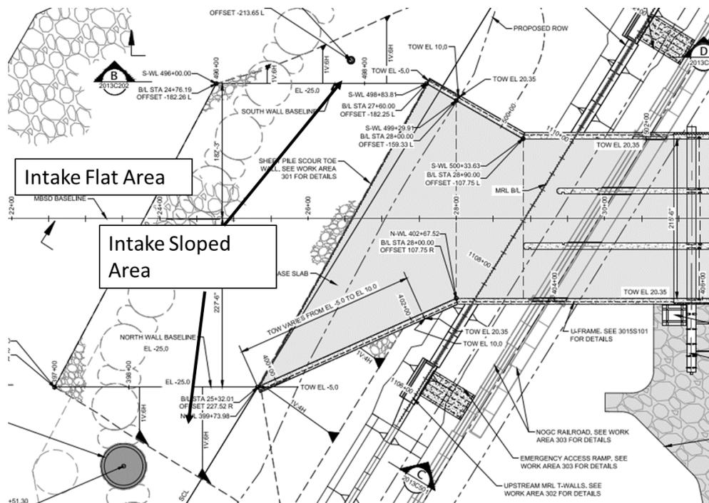
**Figure 6.6-4: Armored sections of the Diversion Intake**
