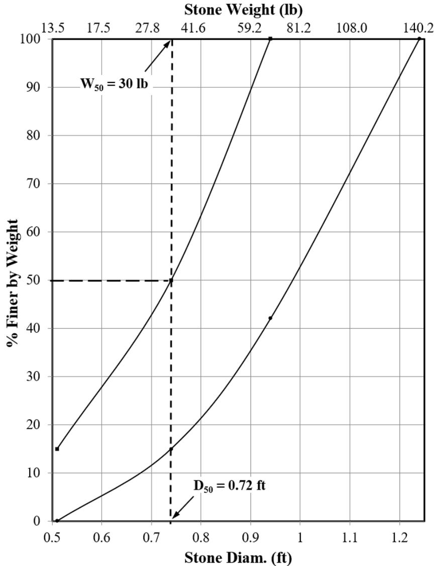
**Figure 6.6-11: Gradation Curves for LaDOTD 30 LB Class Riprap**
