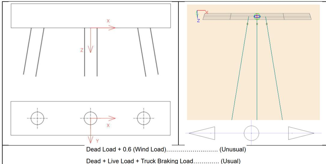
**Figure 5.4-18: Pile load combinations and CPGA model**
