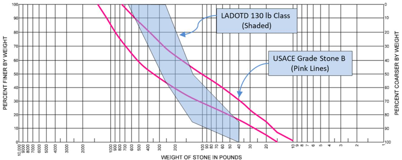
**Figure 6.6-1: LaDOTD 130 lb Class Riprap and USACE Grade Stone B Gradation Plots**
