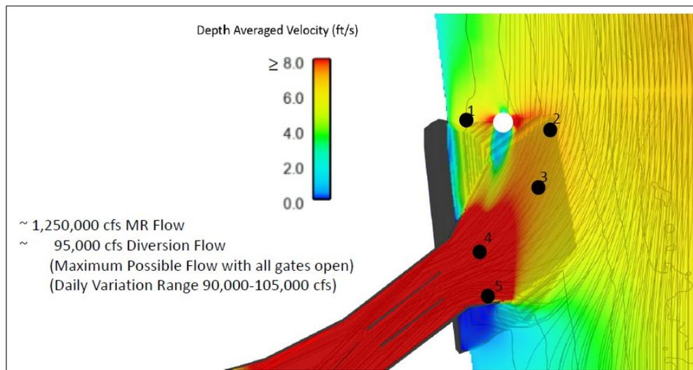
**Figure 6.6-2: Depth-Average Velocities, 95k cfs MBSD / 1.25M cfs MR, from April 2021 Model**
