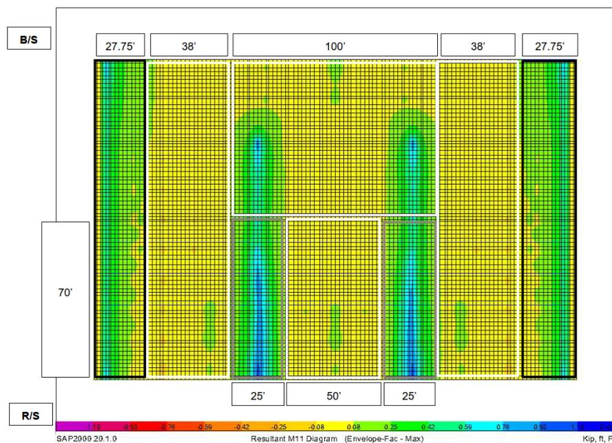
**Figure 5.4-5: Positive moment envelope in the direction perpendicular to the flow**
