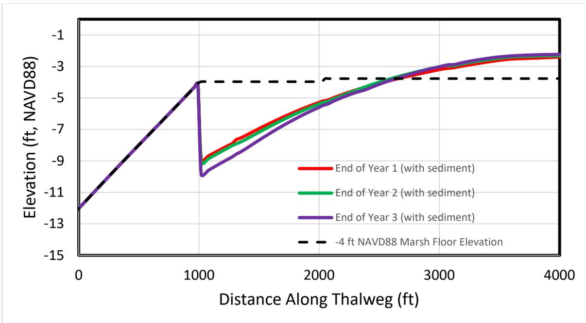
**Figure 3.2-5: Predicted scour bed elevations**
