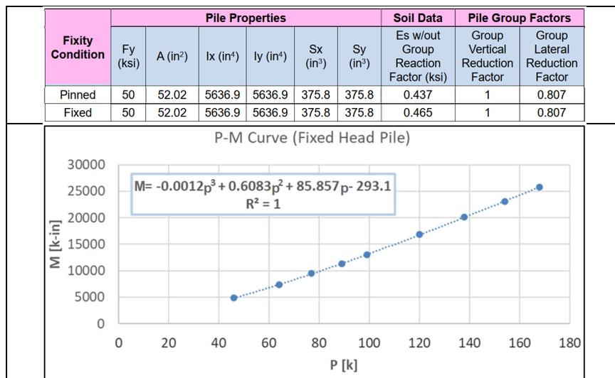
Figure 5.4-4: Pile properties and the P-M curve for the fixed head connection
