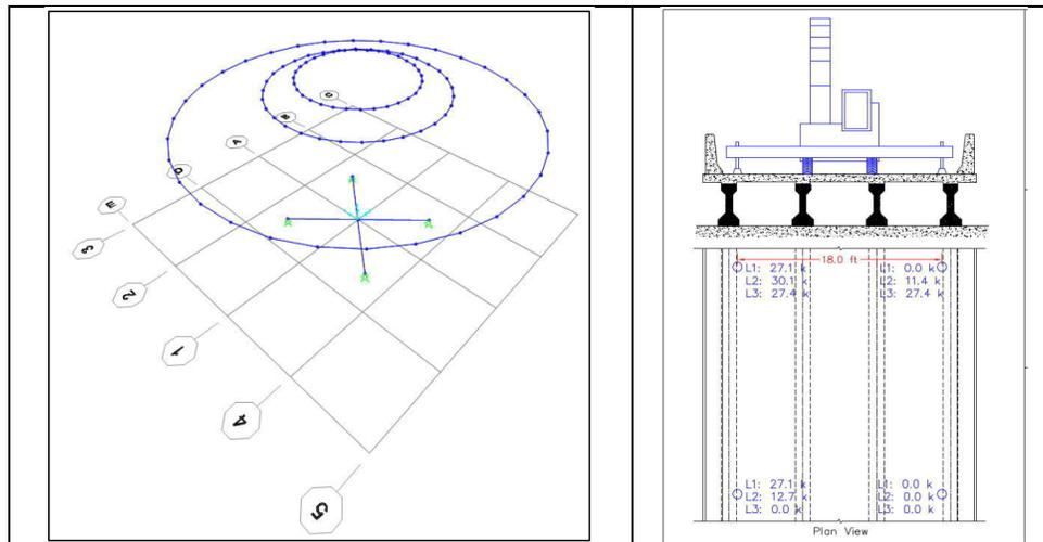
**Figure 5.4-15: Loaded crane modeled as a moving load in 3 different boom lengths and angles, and the worst reactions under the outriggers**
