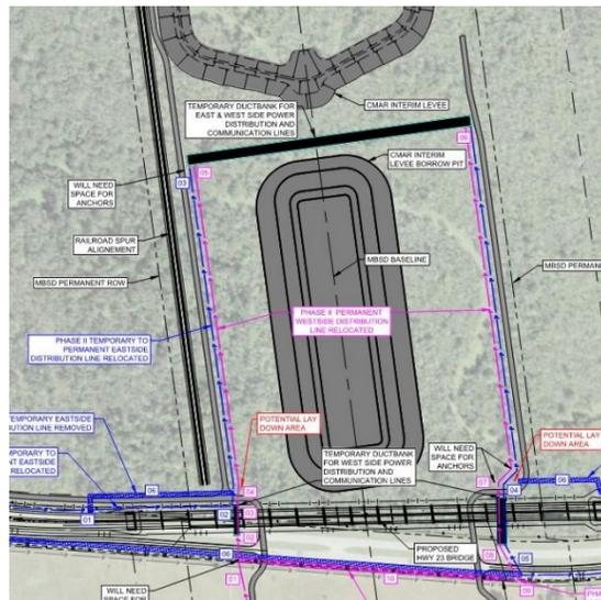
**Figure 6.8-4: Entergy Distribution Phase 2 Relocation**
