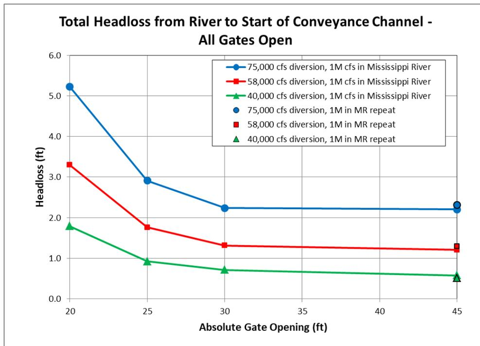
**Figure 3.3-7: Total head loss through the diversion with all gates open.**
