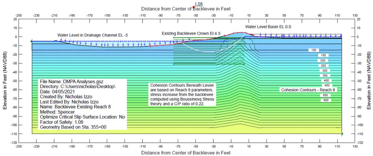
**Figure 6.7-12: Existing back levee slip surface analysis for existing conditions**
