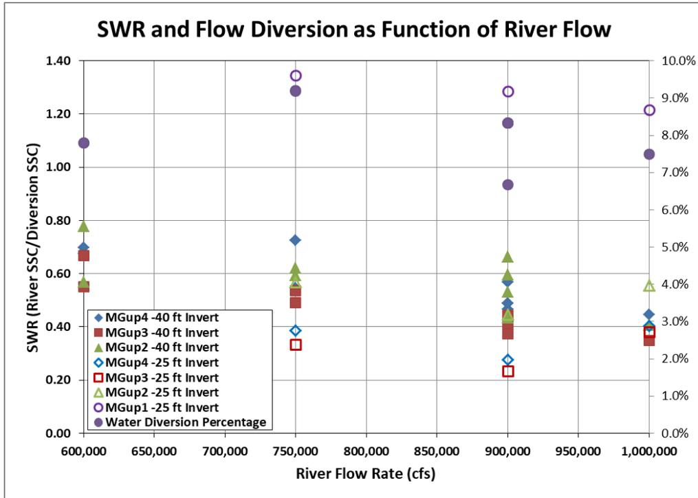
**Figure 3.3-10: SWR and flow diversion as a function of river flow.**
