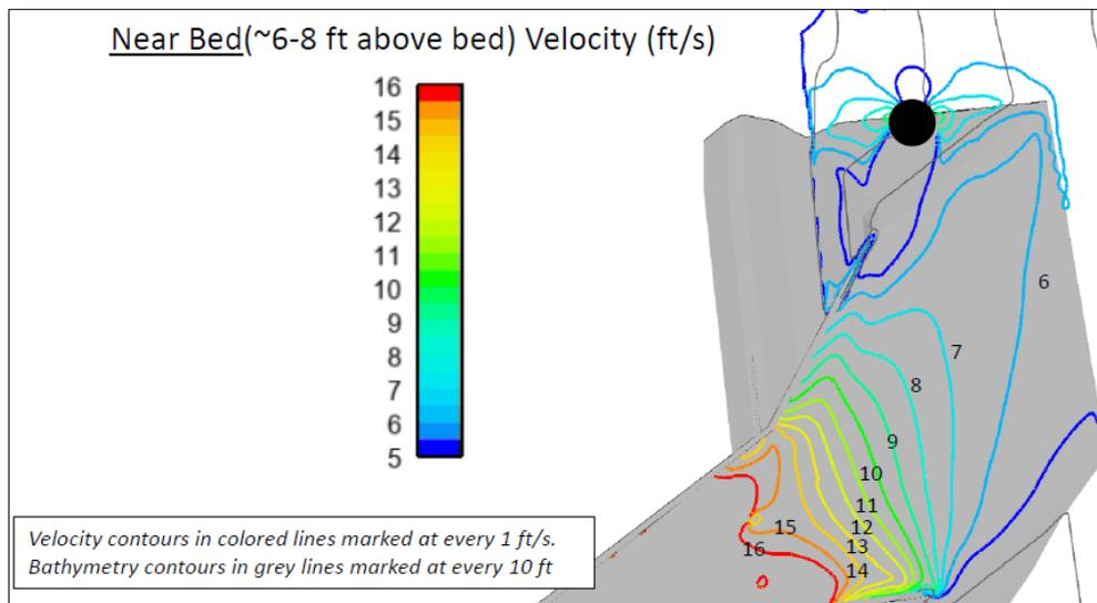
**Figure 6.6-3: Near-Bed Velocities, 95k cfs MBSD / 1.25M cfs MR, from April 2021 Model**
