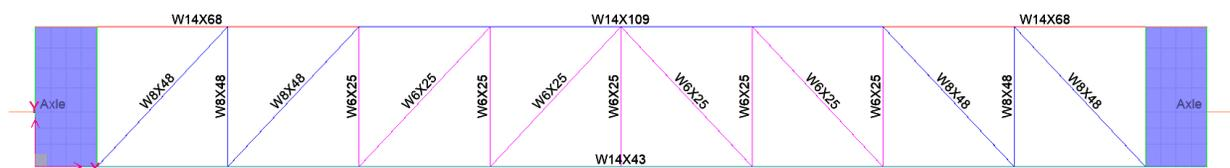
**Figure 5.4-7: Plan View of Typical Bulkhead Truss**
