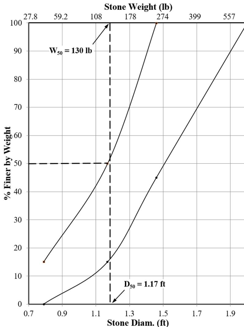
**Figure 6.6-9: Gradation Curves for LaDOTD 130 LB Class Riprap**
