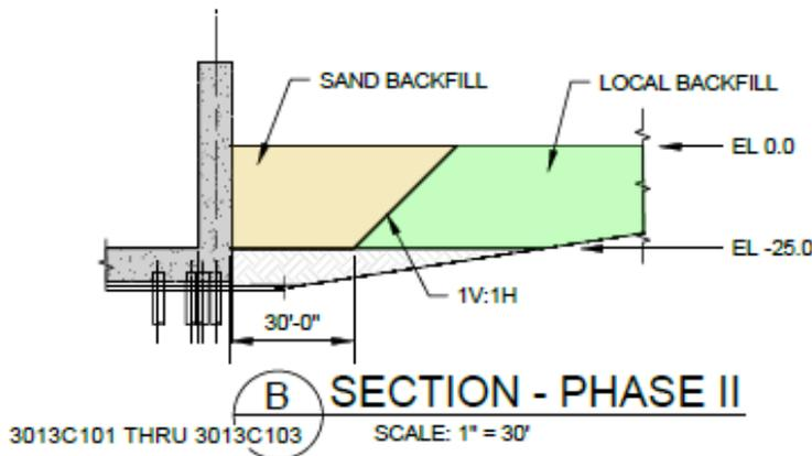
Figure 4.2-2: Sand Backfill Adjacent to U-frame and Gated structure Walls – Phase II (shown in yellow)
