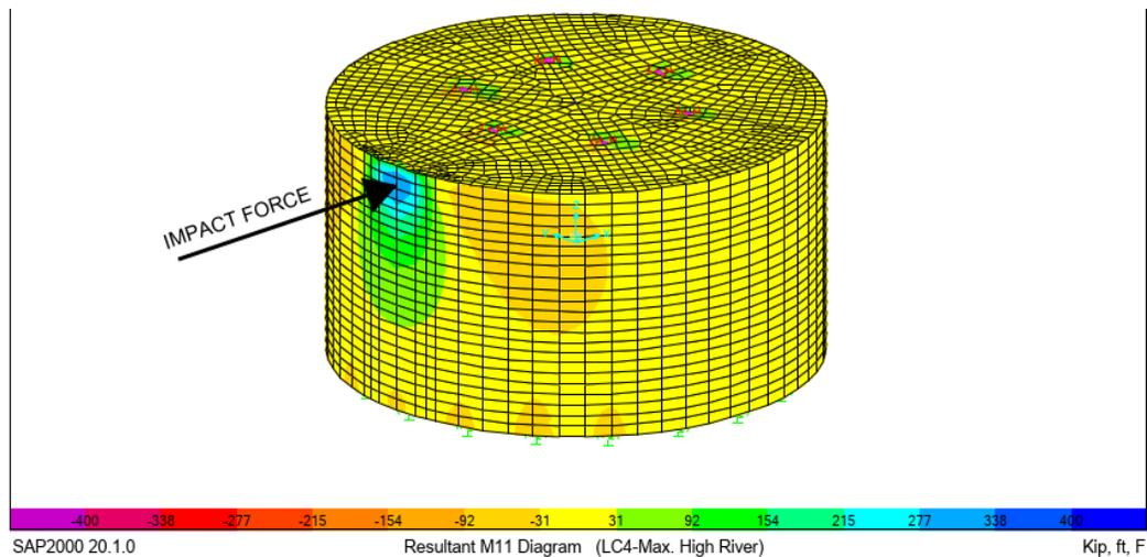
**Figure 5.3-5: SAP2000 Model for Worst-Case Bending**
