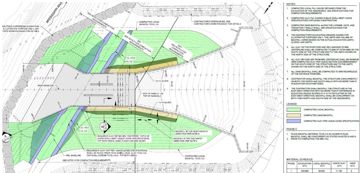
Figure 4.2-1: Sand Backfill Adjacent to U-frame and Gated structure Walls – Phase II (shown in yellow)
