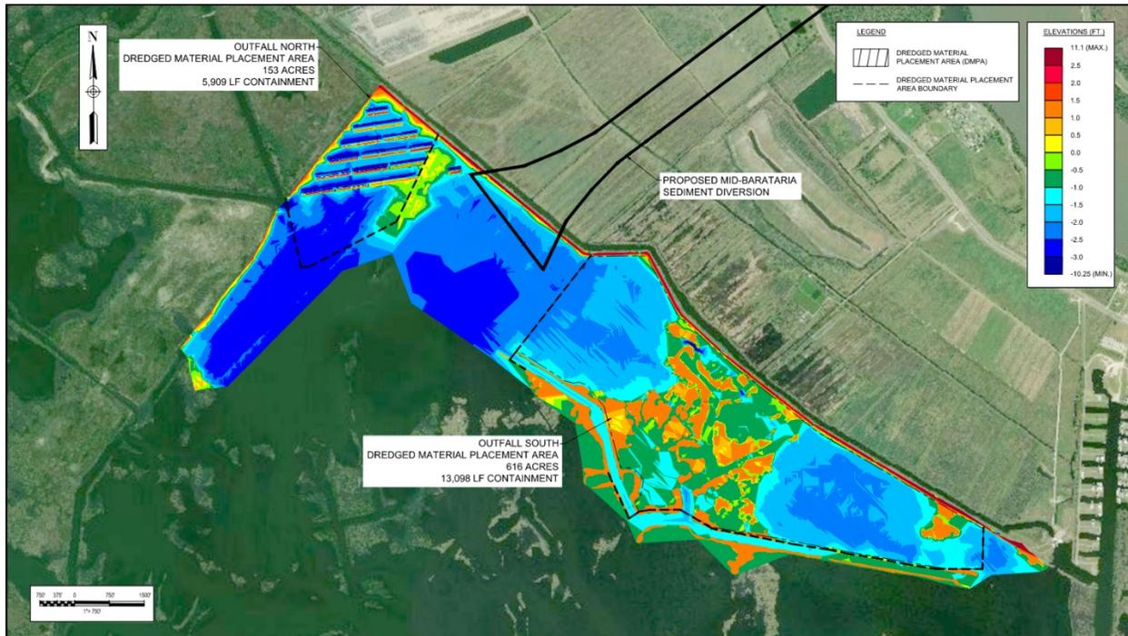
**Figure 6.7-16: Dredged material placement areas contour map**
