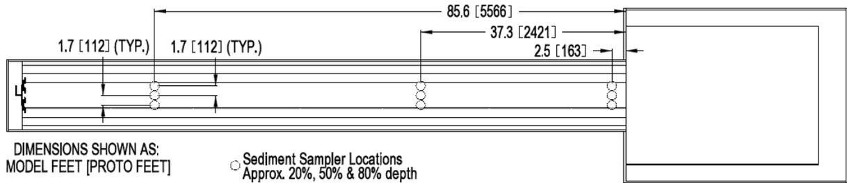
Figure 3.3-2: Location of suspended sediment sampling in conveyance channel.
