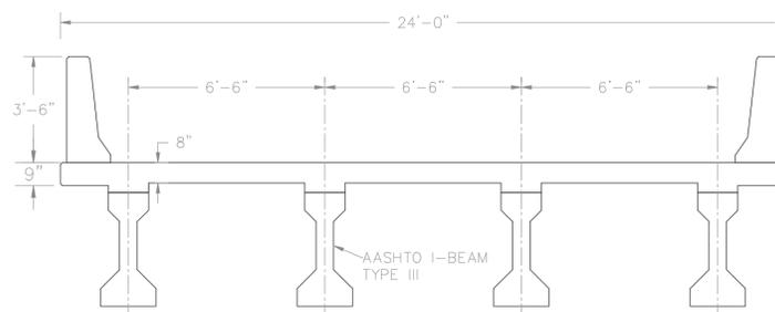
**Figure 5.4-12: Section with 24 ft. width (over the gated structure)**
