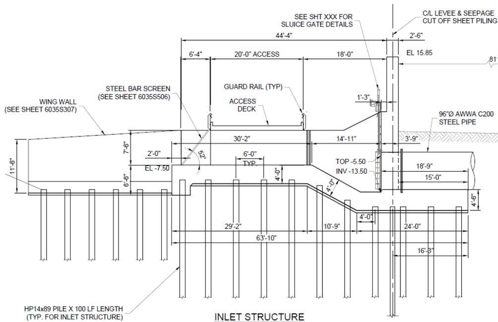
**Figure 5.11-1: Combined Inlet/Wingwall Structure**
