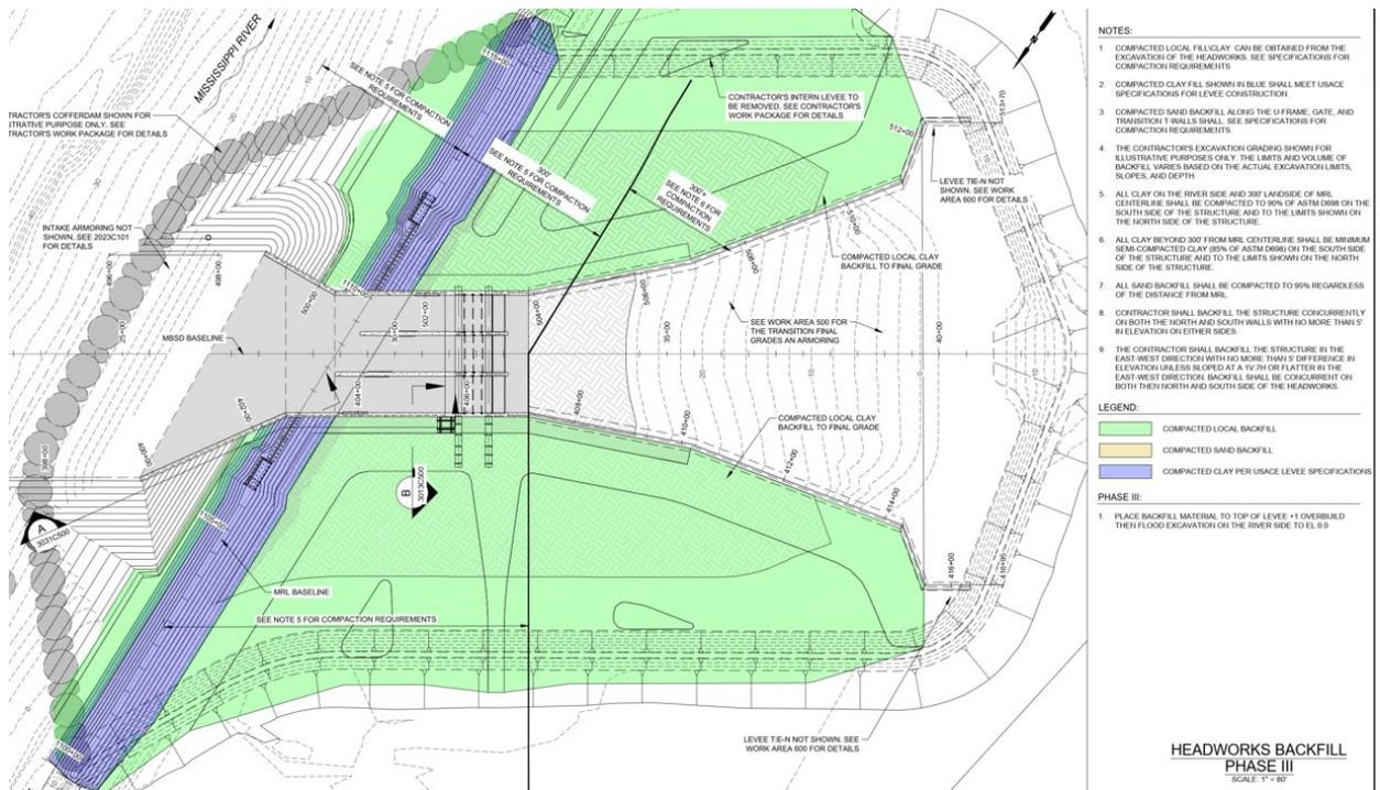
Figure 4.2-3: Compacted Local Backfill – Phase III (plan view)
