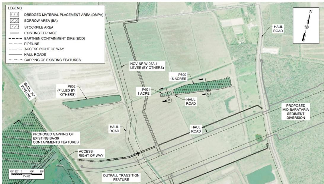
**Figure 6.7-8: Existing Borrow Pits Plan View**
