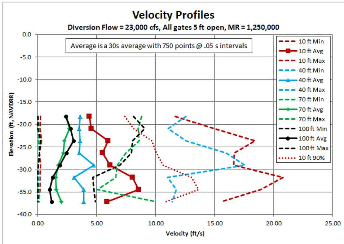
**Figure 6.6-10: Velocity Profiles in the Transition Section - All Gates Open 4-ft, River at 1.25 M cfs, and Diversion Flow of 23,000 cfs**
