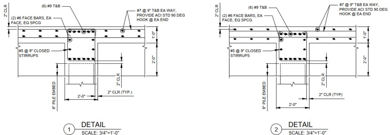
**Figure 5.7-1: Electric Building and Generator Platform Cross-Section**
