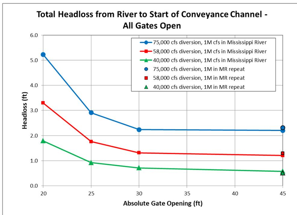
**Figure 3.3-7: Total head loss through the diversion with all gates open.**
