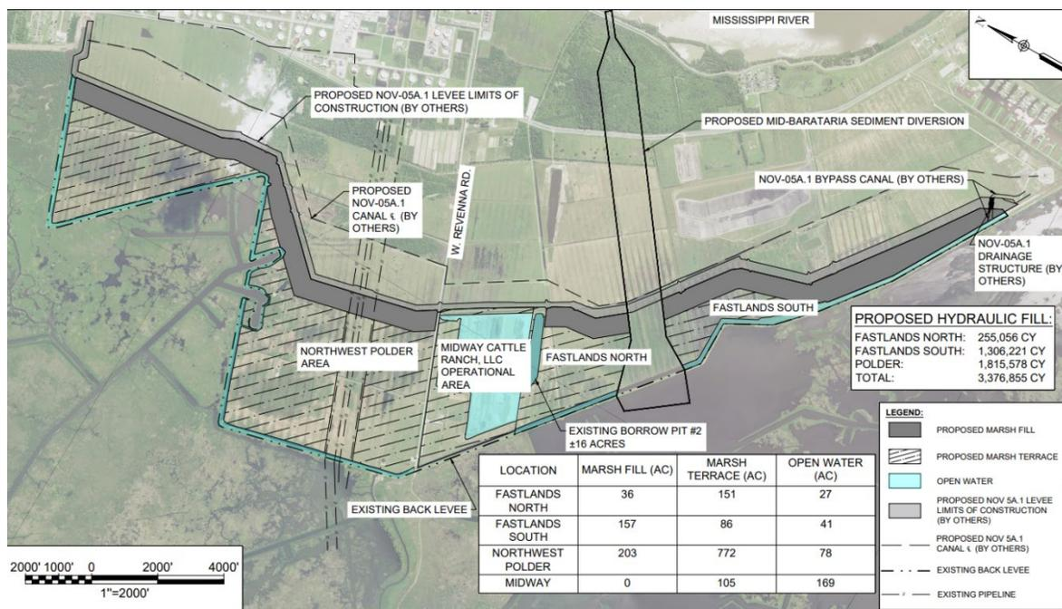
**Figure 6.7-7: NOV-NF-W-05a.1 Levee Vicinity Restoration Design Alternative**
