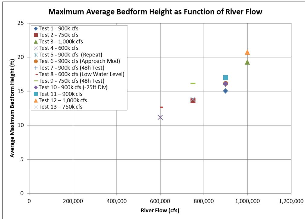
**Figure 3.3-11: River flow vs. average bedform height upstream of diversion.**
