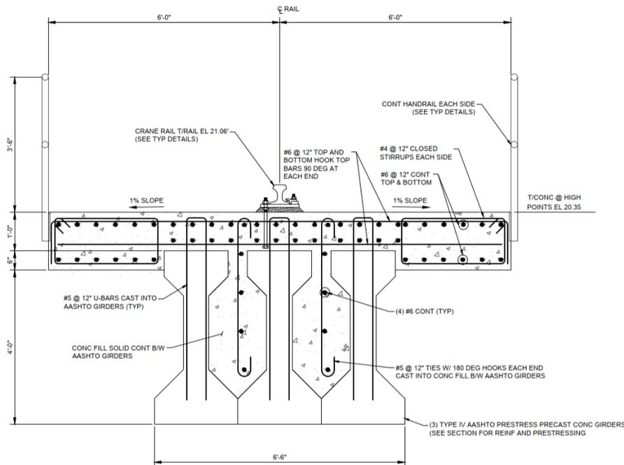
**Figure 5.5-1: Gantry Crane Rail Beam Cross-Section**
