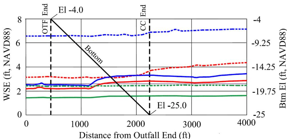
**Figure 6.6-16: Water Surface Elevations in the Outfall section for various model cases**
