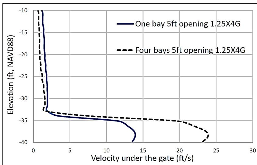
**Figure 6.6-7: Velocity Under a Partially Open Gate or Gates**
