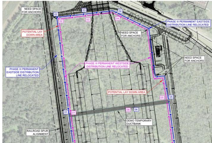
**Figure 6.8-5: Entergy Distribution Phase 3 Relocation**
