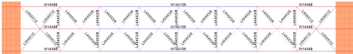
**Figure 5.4-8: Elevation View of Downstream (Basin) Side Framing**
