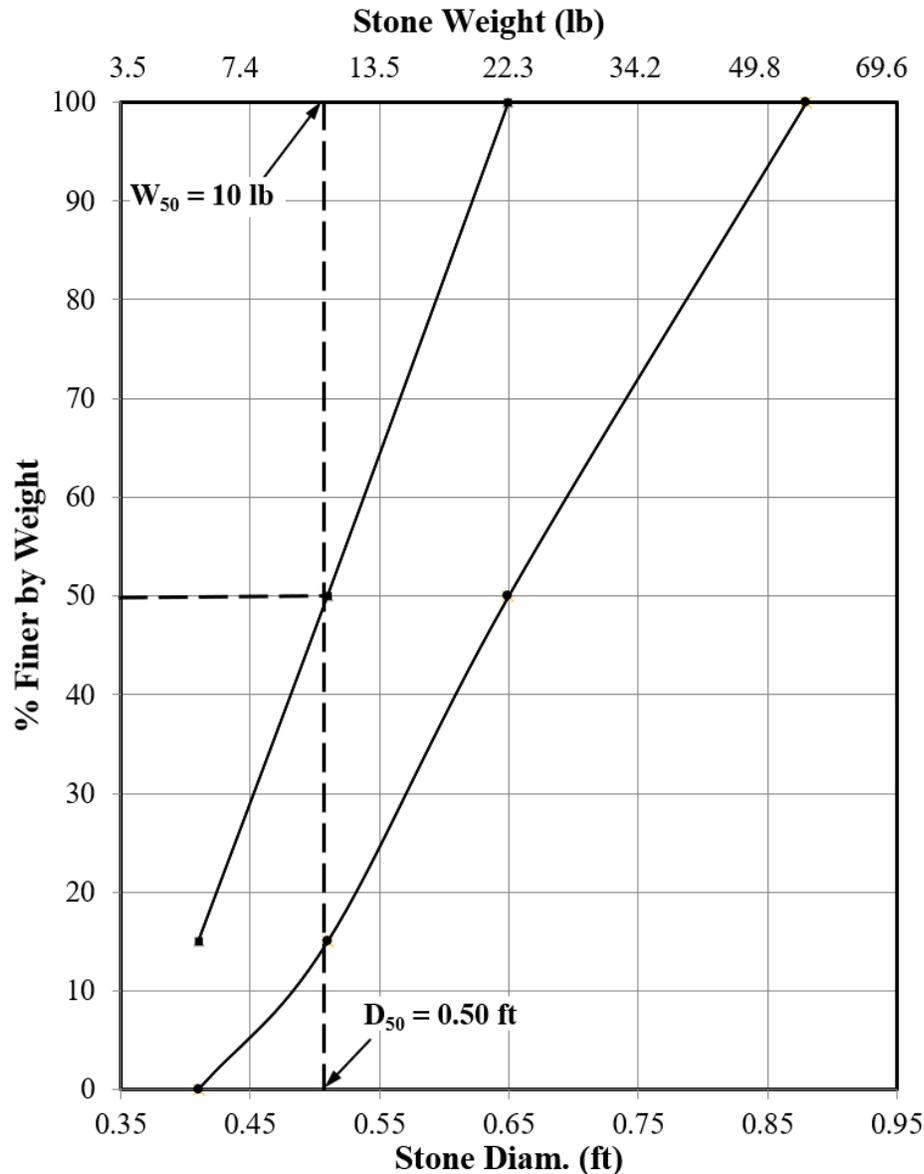
Figure 6.6-14: Gradation Curves for LaDOTD 10 LB Class Riprap
