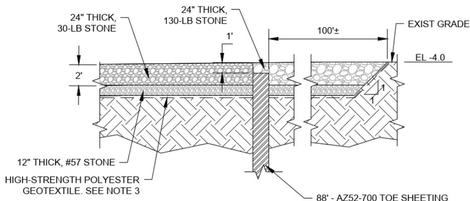
**Figure 5.10-2 OTF Sheet Pile End Wall Detail**
