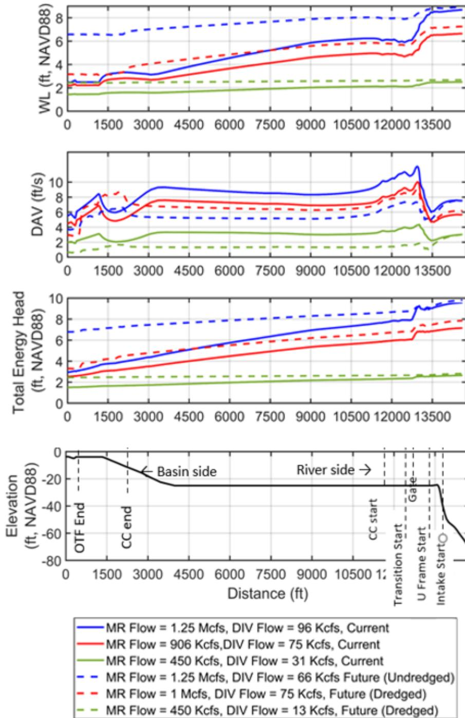
**Figure 3.2-1: Predicted Profiles of the Water Surface Elevation, the Depth-Averaged Velocity (DAV) and the Total Energy Head Along the Length of the Diversion System. Flow is from right (river end) to left (outfall end) in the above panels.**
