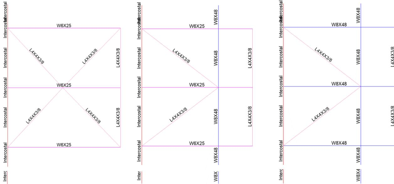
**Figure 5.4-9: Cross-Sections of Bulkhead Framing**
