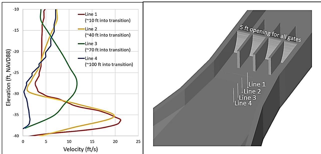
**Figure 6.6-8: Velocities at Various Locations for Partially Opened Gates**
