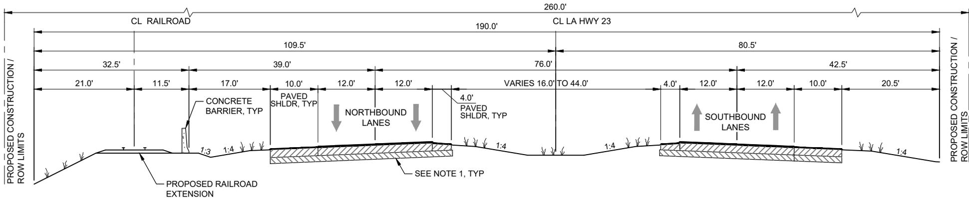
TYPICAL ROAD SECTION FOR REALIGNMENT AT GRADE RAIL (LOOKING SOUTH)
