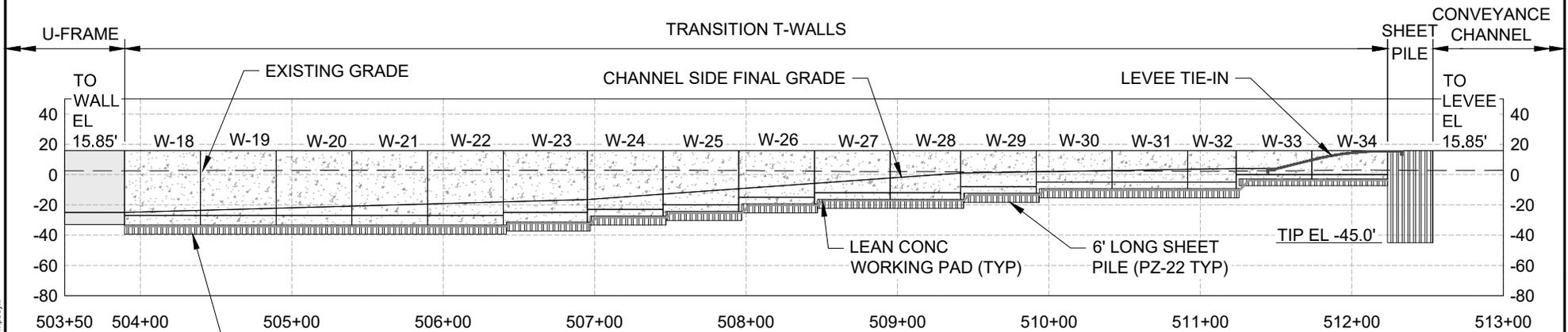
FOUNDATION PILES NOT SHOWN FOR CLARITY, PILES ARE 24"Ø WITH VARYING TIP ELEVATIONS FROM -100 TO -190
