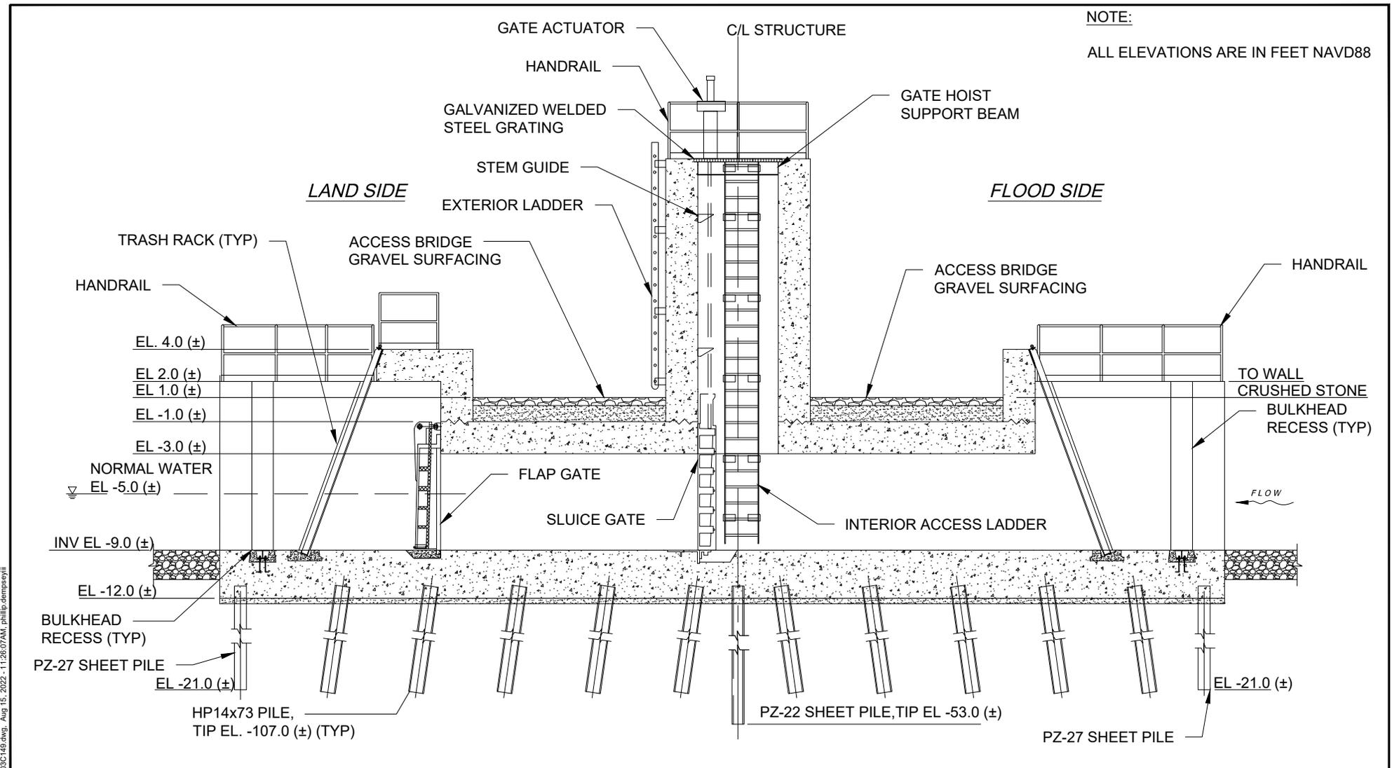
**A NOV-NF-W-05a.1 DRAINAGE STRUCTURE PROFILE**
