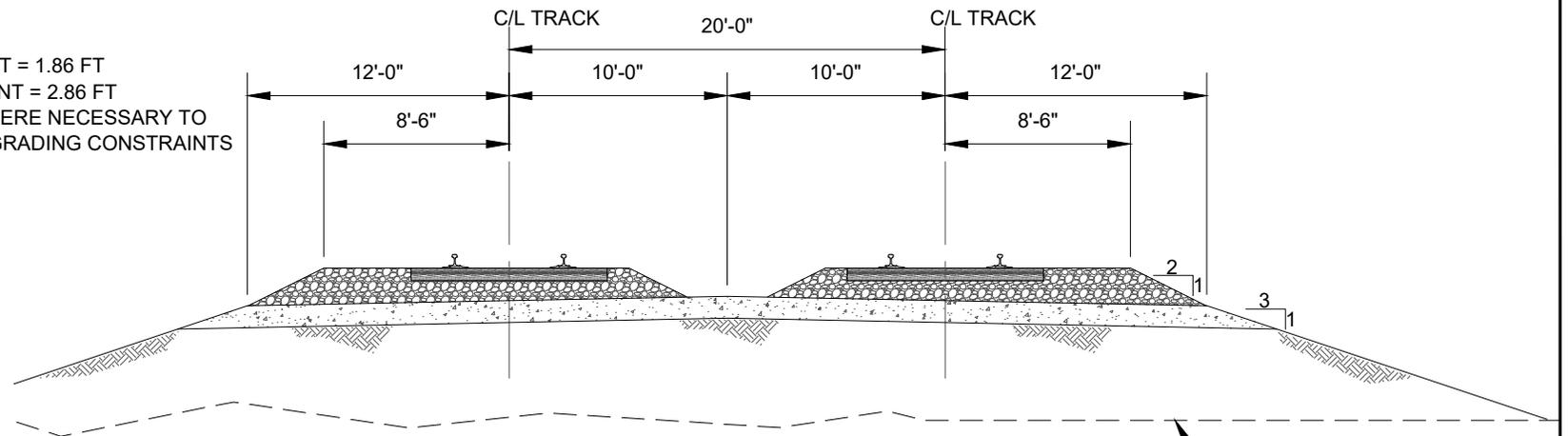
**B** TYPICAL SPUR TRACK SECTION - PARALLEL TRACKS
