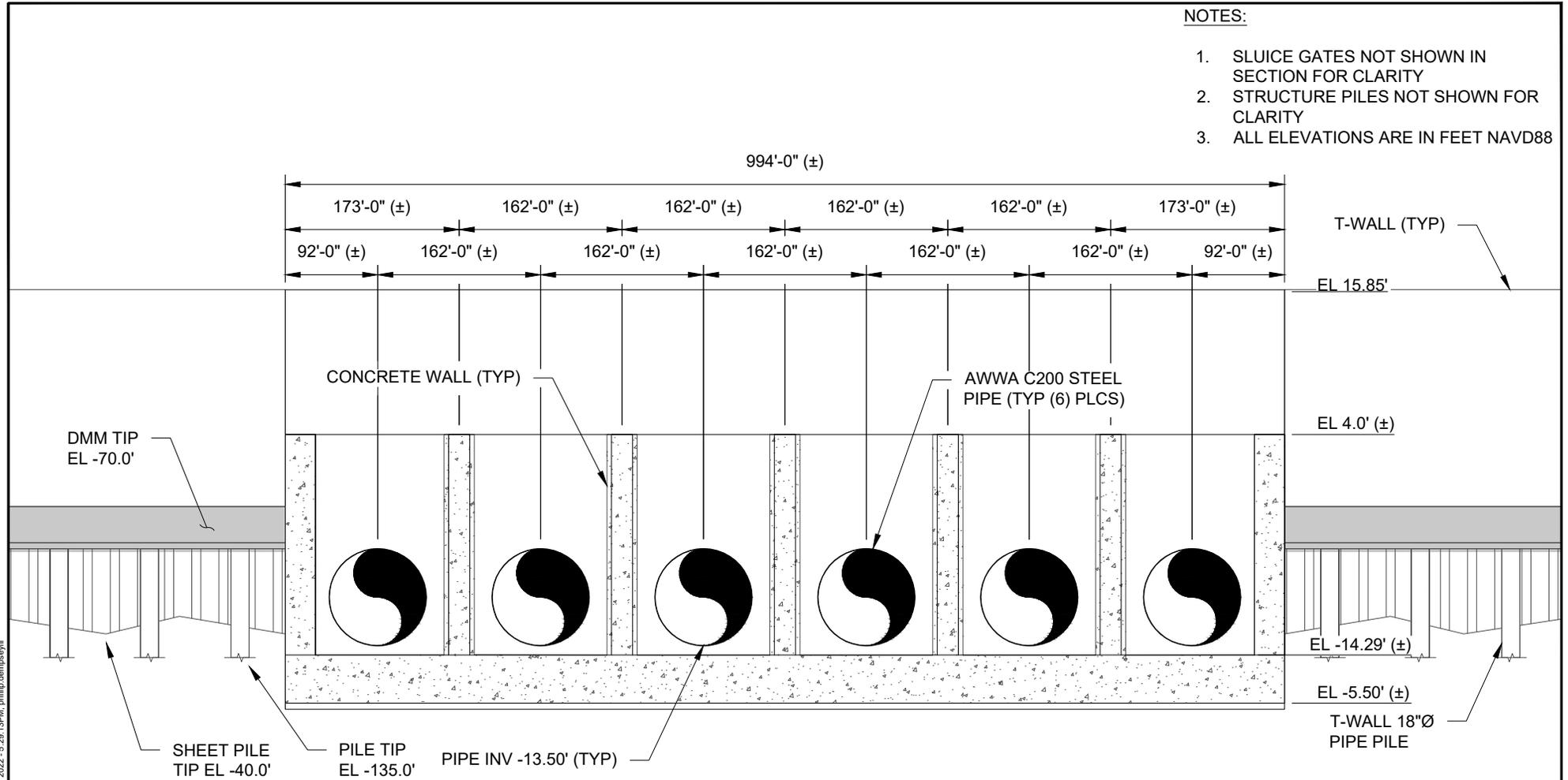
**A** INVERTED SIPHON INTAKE SECTION
