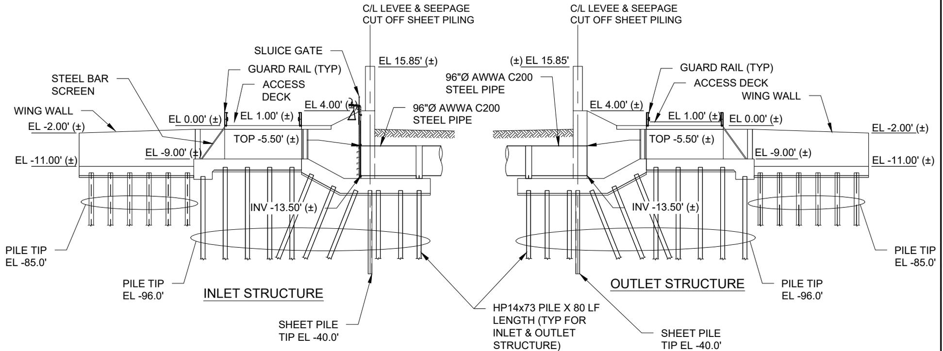
**B** **INVERTED SIPHON STRUCTURE SECTION**
