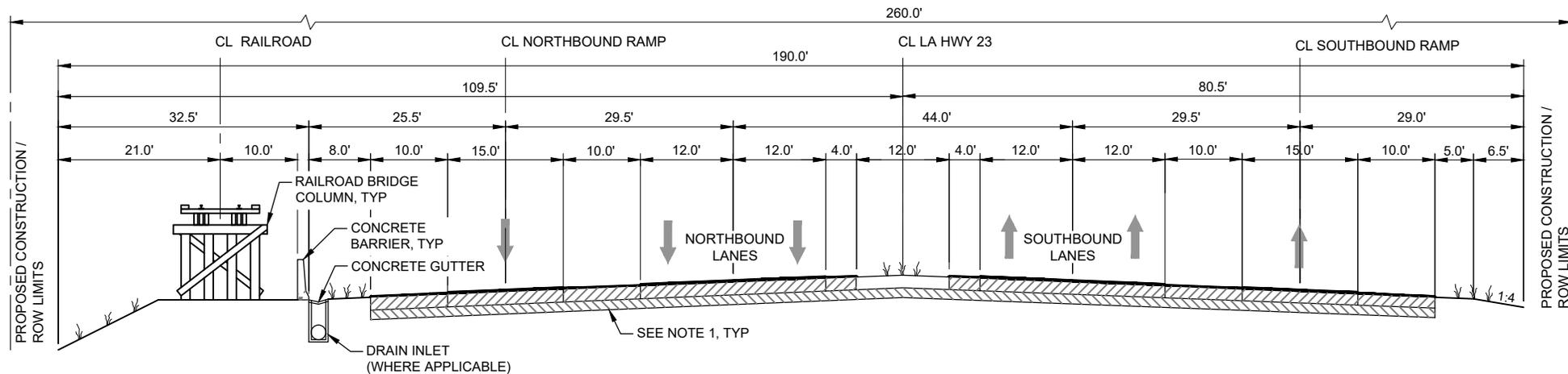
TYPICAL ROAD SECTION FOR REALIGNMENT WITH RAIL BRIDGE (LOOKING SOUTH)
