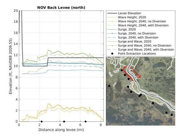
Figure 4.20-22. Comparison of 1 Percent AEP Storm Surge Elevation and Wave Height to Northern NOV-NFL Modeled Levee Height in Years 2020 and 2040 under the No Action Alternative and Applicant's Preferred Alternative.
