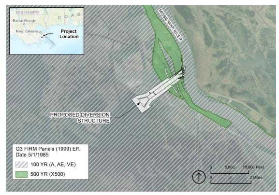
Figure 4.20-1. Construction Footprint in Relation to 100-year and 500-year Floodplains.
