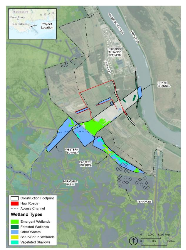
Figure 4.6-1. Wetlands within the Project Construction Footprint.
