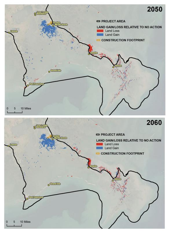
Figure 4.2-3.Model-projected Land Loss and Gain in the Project Area Relative to the No<br/>Action Alternative in 2050 and 2060 under the Applicant's Preferred Alternative.<br/>Map depicts all model results but results in Table 4.2-4 only tabulated within the<br/>Project area, depicted above.
