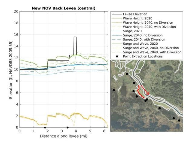
Figure 4.20-24. Comparison of 1 Percent AEP Storm Surge Elevation and Wave Heights to Central NOV-NFL Modeled Levee Height in Years 2020 and 2040 under the No Action Alternative and Applicant's Preferred Alternative.
