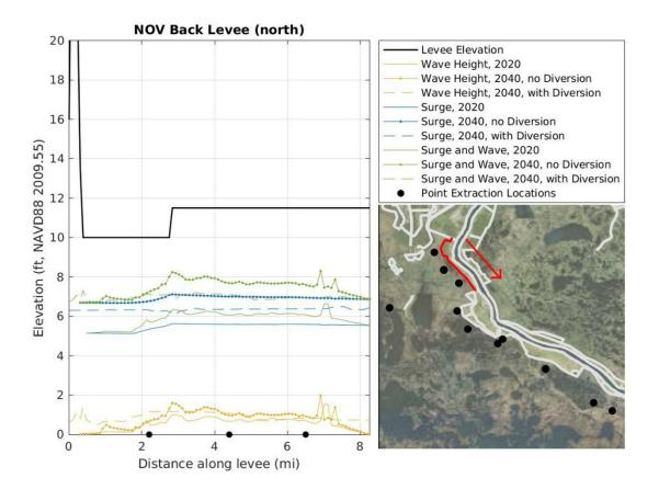
Figure 4.20-23. Comparison of 4 Percent AEP Storm Surge Elevation and Wave Height to Northern NOV-NFL Modeled Levee Height in Years 2020 and 2040 under the No Action Alternative and Applicant's Preferred Alternative.
