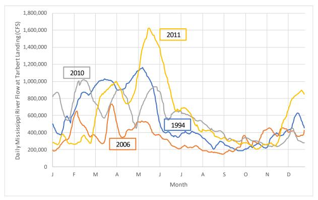
Figure 4.1-2. Mississippi River Hydrographs for Four Additional Flow Regime Years for Each Decade used in the Delft3D Basinwide Model.
