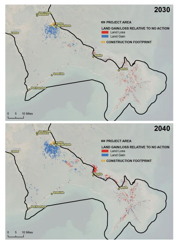
Figure 4.2-2.Model-projected Land Loss and Gain in the Project Area Relative to the No<br/>Action Alternative in 2030 and 2040 under the Applicant's Preferred Alternative.<br/>Map depicts all model results but results in Table 4.2-4 only tabulated within the<br/>Project area, depicted above.
