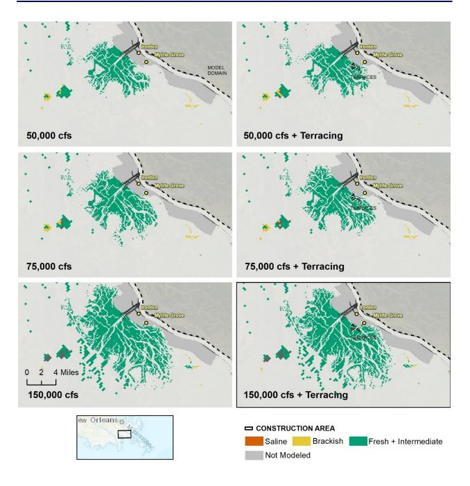
Figure 4.6-15. Wetland Extent Near the Delta Formation Area for Each Action Alternative in 2070.
