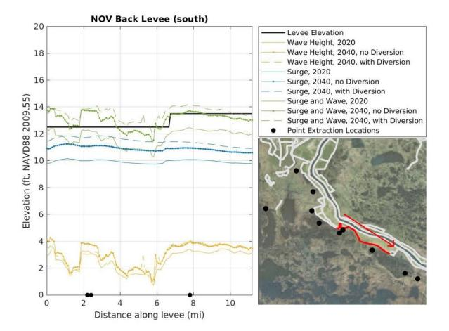
Figure 4.20-26. Comparison of 1 Percent AEP Storm Surge Elevation and Wave Heights to Southern NOV-NFL Modeled Levee Height in Years 2020 and 2040 under the No Action Alternative and Applicant's Preferred Alternative.
