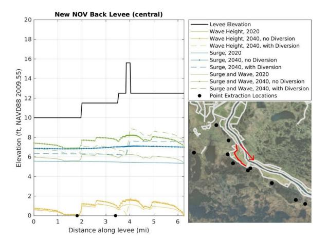
Figure 4.20-25. Comparison of 4 Percent AEP Storm Surge Elevation and Wave Heights to Central NOV-NFL Modeled Levee Height in Years 2020 and 2040 under the No Action Alternative and Applicant's Preferred Alternative.
