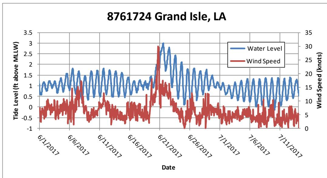
**Figure 3.4-3. Water Level and Wind Speed at the Grand Isle, LA Station.** USGS gages and CRMS stations throughout the Barataria Basin report daily or hourly water levels, most of which are referenced to the NAVD88 datum (USGS 2017d, CPRA 2017b). As shown in Table 3.4-1, average water levels within the Barataria Basin are generally about 1 foot.
