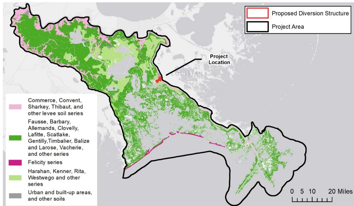
**Figure 3.2-3. Map of Primary Soil Units in Project Area.** Soils on the natural levees within the Project area that are protected from flooding or are rarely or occasionally flooded include Sharkey, Commerce, and Convent series. Soils on the natural levee at the location proposed for the Project diversion structure location belong to the Sharkey-Commerce unit.
