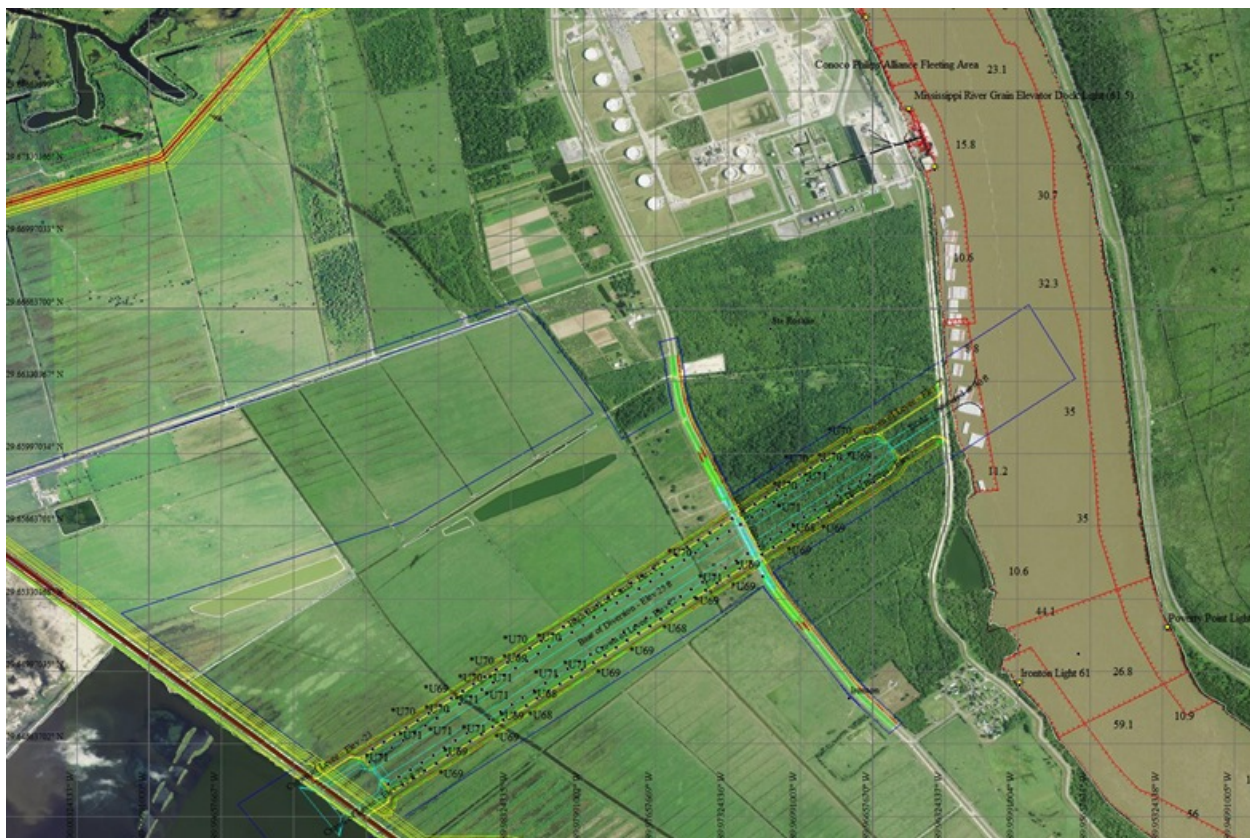
Figure 2: Conceptual Mid-Barataria Sediment Diversion Canal with Control Structures
