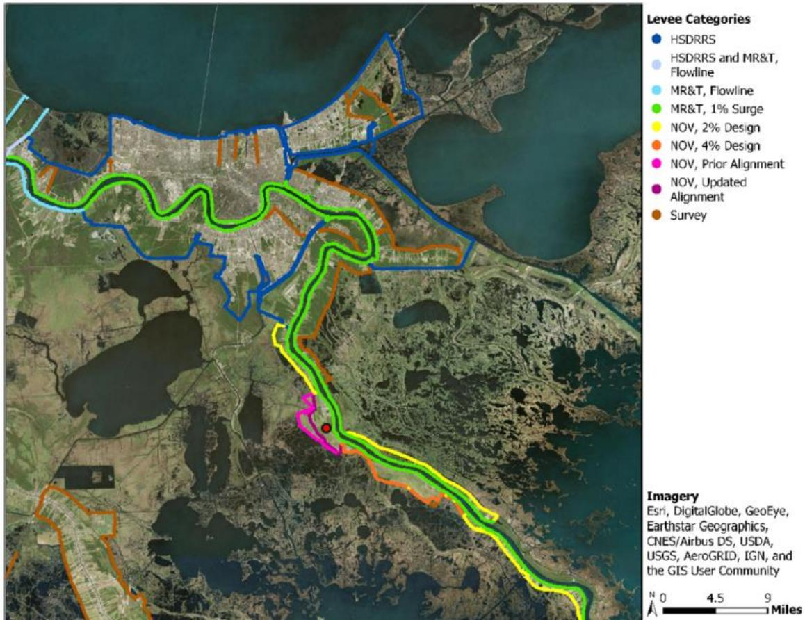
Figure 2-6. Levee Data Sources Used in ADCIRC+SWAN Model.
