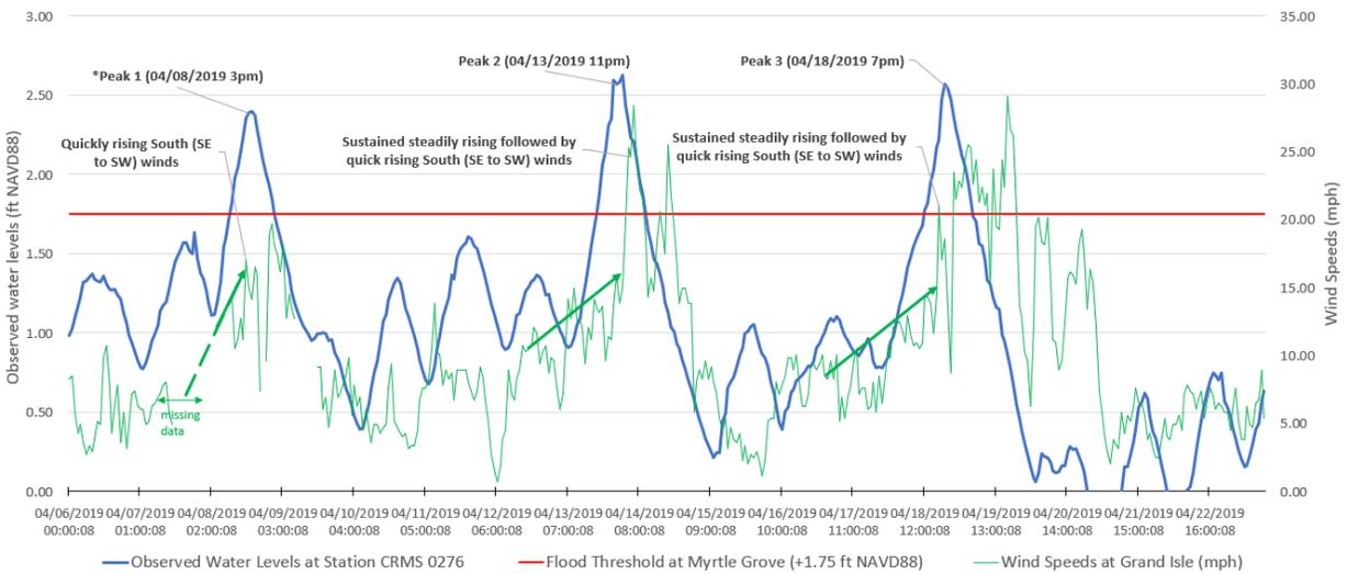
**Figure A 3.** Recent water level data at Myrtle Grove (Station CRMS0276) and wind speeds recorded at Grand Isle (Source NOAA) showing three wind tide peaks. \*The first peak (April 8<sup>th</sup>) was a verification event when water levels were reported by the surveyor and CPRA personnel on site confirming +1.8-2.0 ft NAVD88. Site observation confirmed that flood threshold at +1.75 ft NAVD88 is appropriate to indicate initial flood event in this area.
