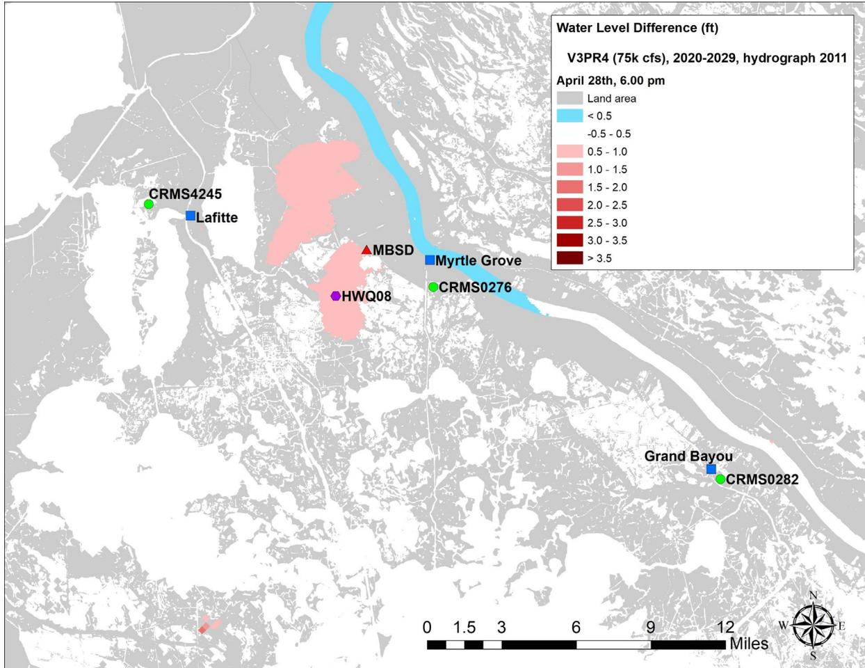
Figure 31: Difference in instantaneous WSEs for FWOP (V3PR1) and FWP (V3PR4, 75k cfs) during a wind driven peak event during the 2020s, 2011 hydrograph on April 28<sup>th</sup>, 2011 at 6 pm.
