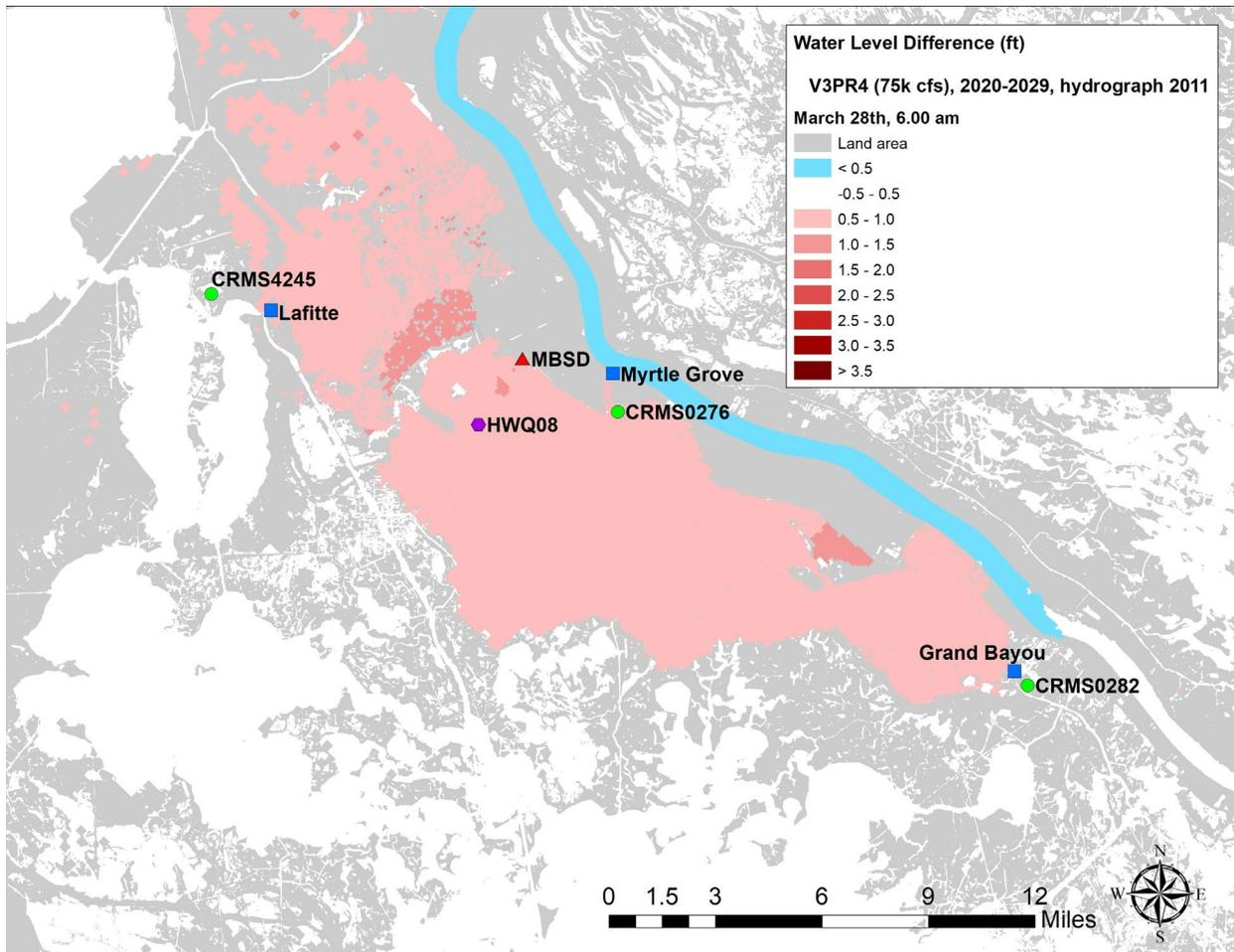
Figure 30: Difference in instantaneous WSEs for FWOP (V3PR1) and FWP (V3PR4, 75k cfs) during a wind driven peak event during the 2020s, on March 28<sup>th</sup>, 2011 at 6 am.
