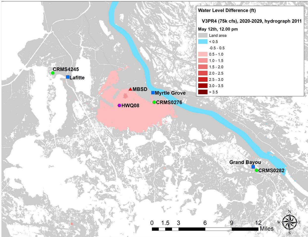
Figure 32: Difference in instantaneous WSEs for FWOP (V3PR1) and FWP (V3PR4, 75k cfs) during a wind driven peak event during the 2020s, on May 12<sup>th</sup>, 2011 at noon.
