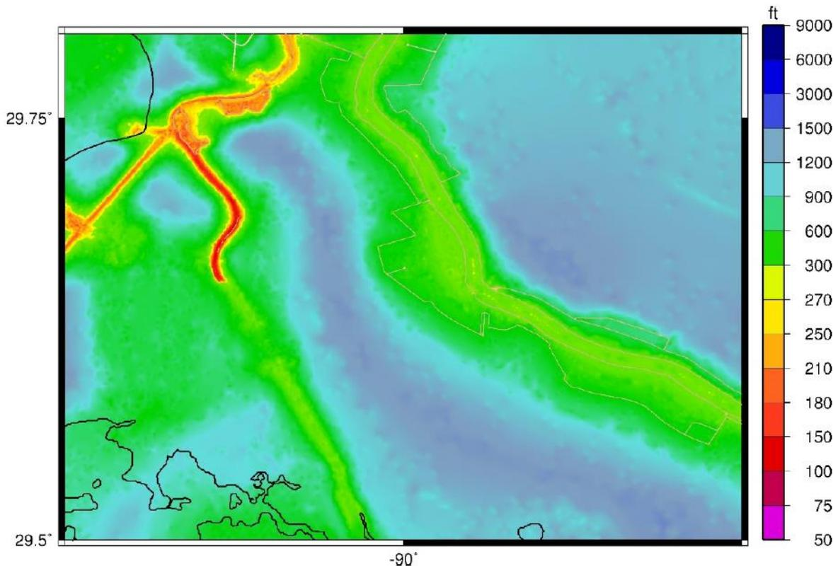
Figure 2-4. Mesh Resolution for the 2017 Master Plan Model.
