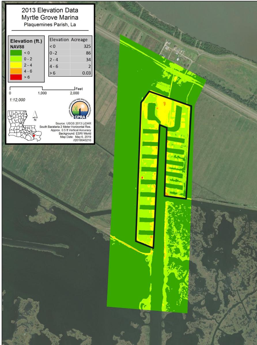
Figure A 2. USGS 2013 LiDAR (DEM) showing ground elevations at Myrtle Grove. The ground elevations within the area where the communities are located (black line) are largely in the range +0-2 ft NAVD88 (light green).
