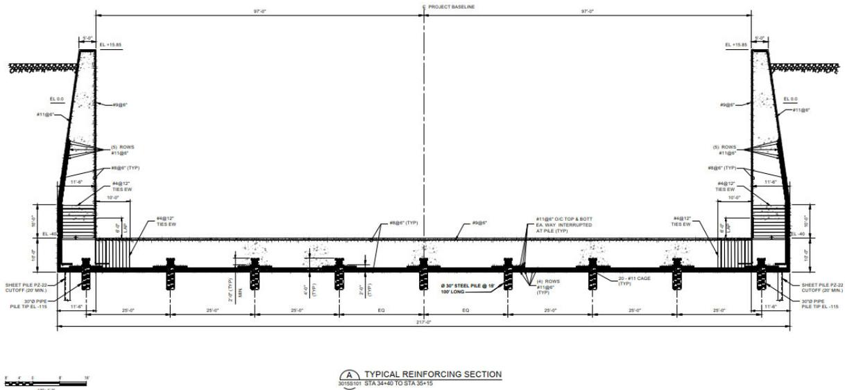
**Figure 5.2-2: Typical U-Boat Section**
