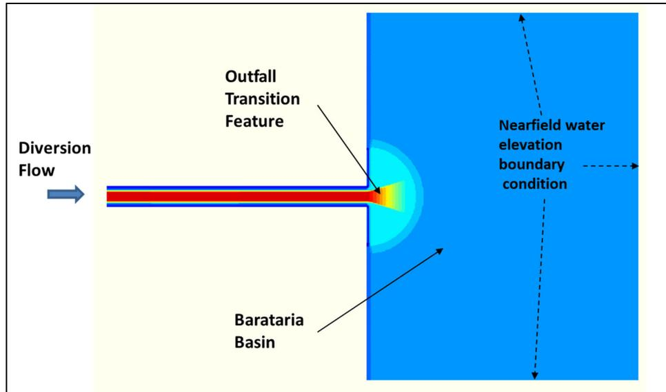
**Figure 3.2-4: Delft3D Model Domain for Conveyance Channel Analysis**
