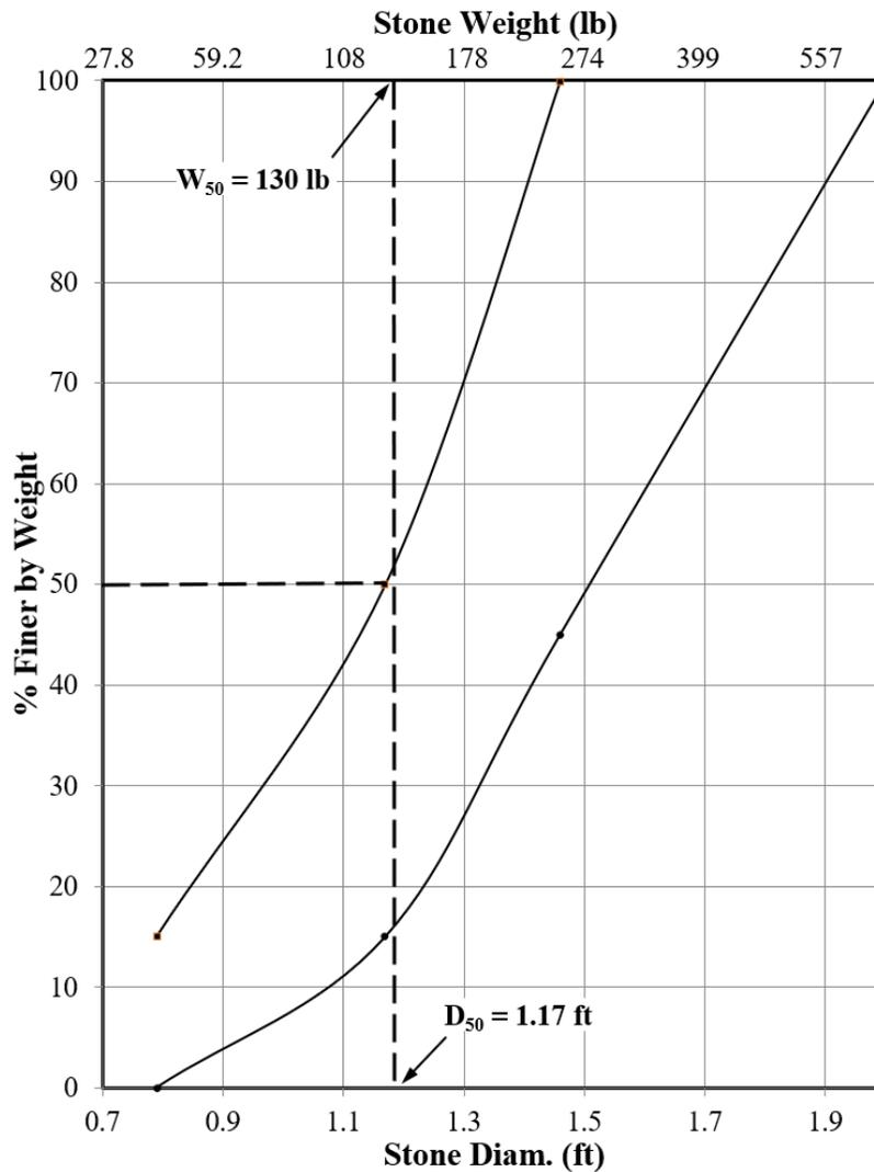
**Figure 6.6-7: Gradation Curves for LADOTD 130 LB Class Riprap**
