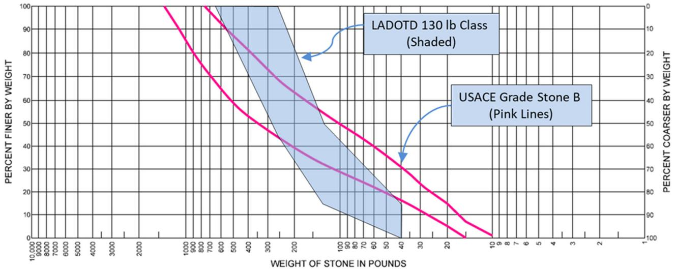
**Figure 6.6-1: LADOTD 130 lb Riprap and USACE Grade Stone B Gradation Plots**
