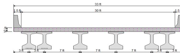
**Figure 3.5-6: Section with 33 ft. width (on the Gated Structure)**
