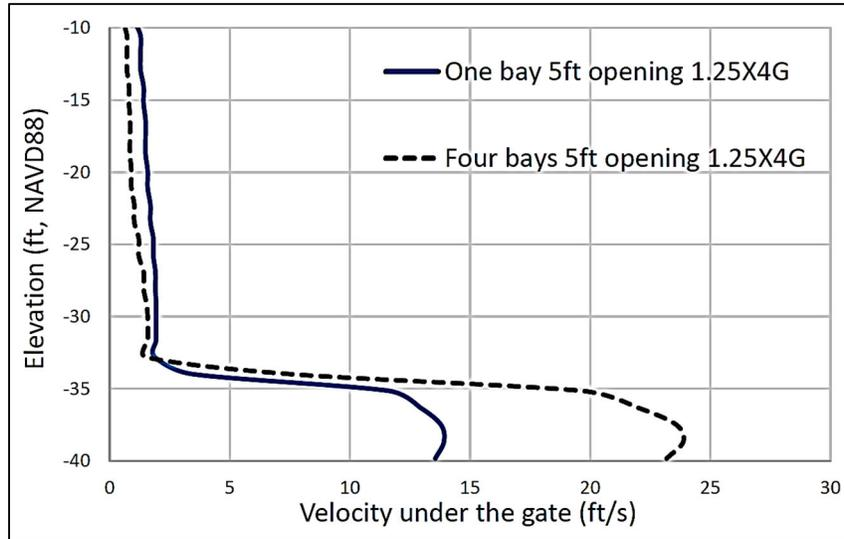
**Figure 6.6-5: Velocity Under a Partially Open Gate or Gates**
