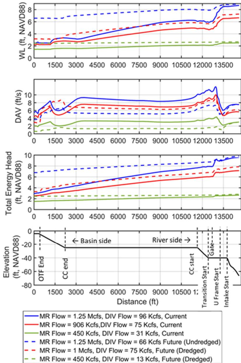
**Figure 3.2-1: The predicted profiles of the water surface elevation, the depth-averaged velocity (DAV) and the total energy head along the length of the diversion system. Flow is from right (river end) to left (outfall end) in the above panels.**
