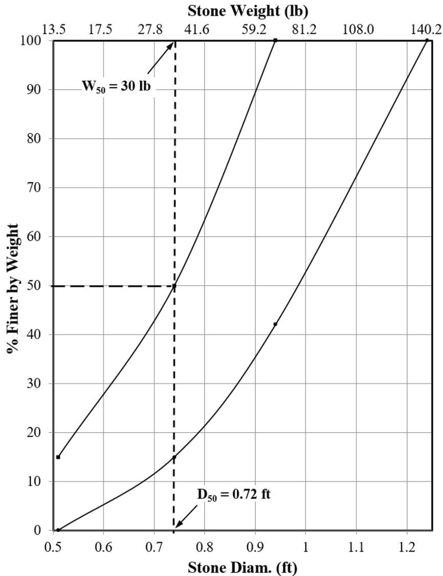
**Figure 6.6-9: Gradation Curves for LADOTD 30 LB Class Riprap**
