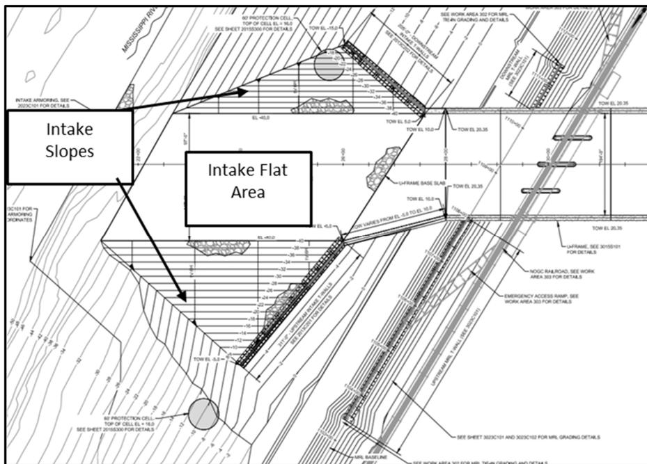
**Figure 6.6-3: Armored sections of the Diversion Intake**
