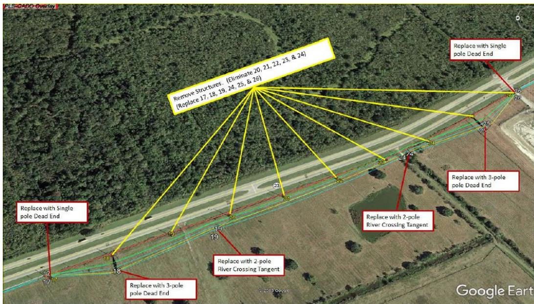
**Figure 6.8-3: Entergy Transmission Relocation Layout**
