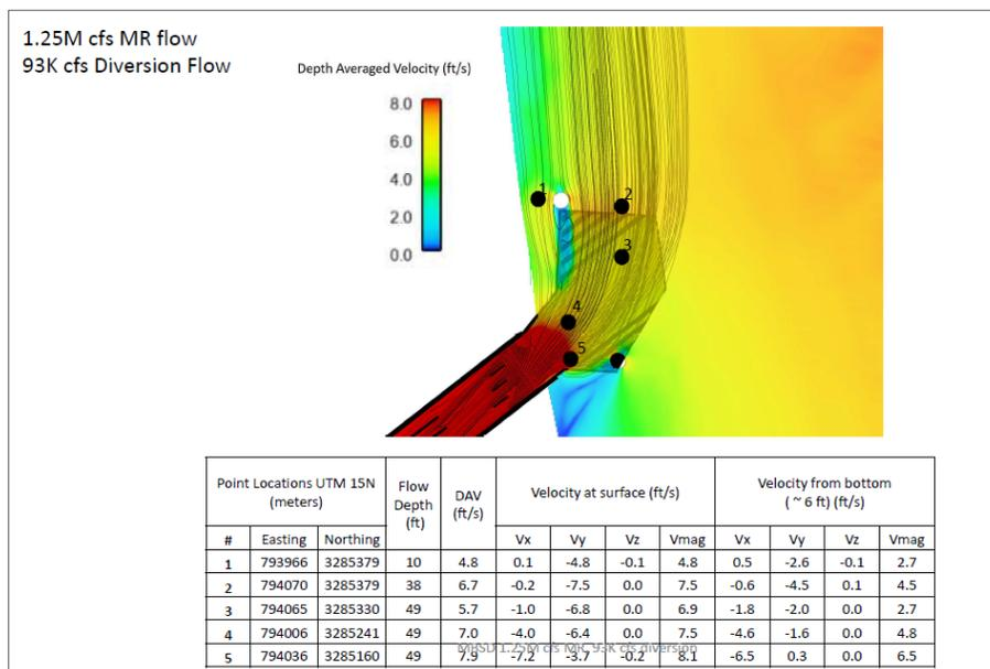
**Figure 6.6-2: Depth-Average Velocities, 93k cfs MBS / 1.25M cfs MR, from June 2019 Model**
