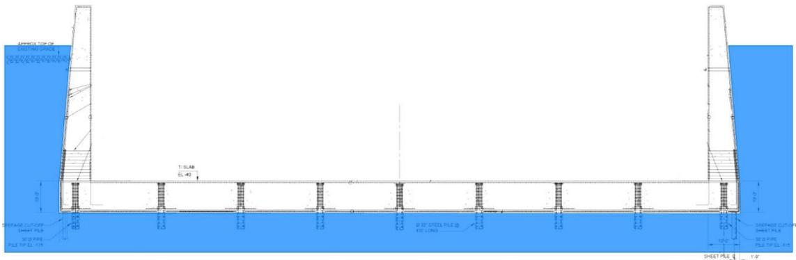
**Figure 5.2-3: Maintenance Dewatering Load Case Schematic**
