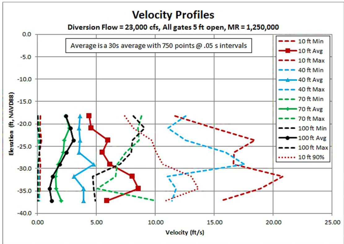
**Figure 6.6-8: Velocity Profiles in the Transition Section - All Gates Open 4-ft, River at 1.25 M cfs, and Diversion Flow of 23,000 cfs**
