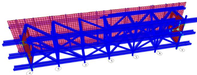
**Figure 5.3-2: 3D View of Bulkheads**
