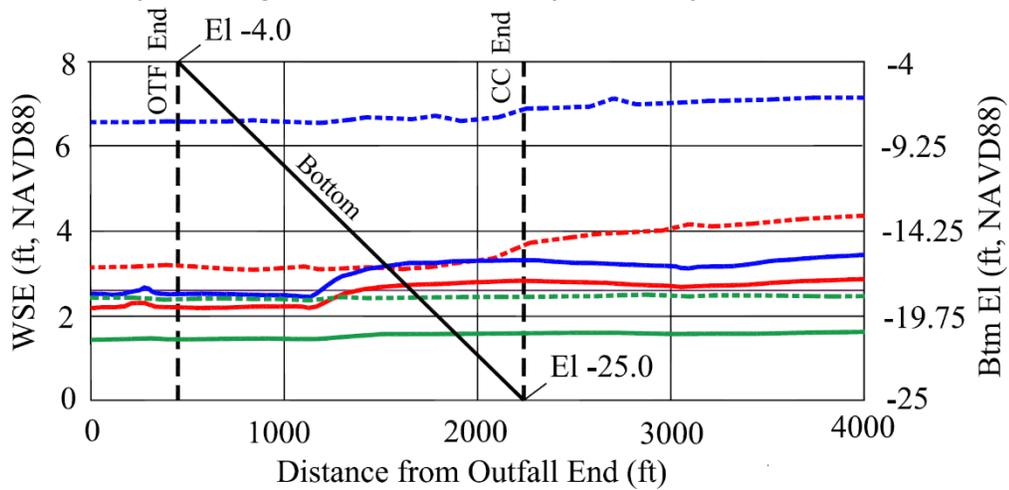
**Figure 6.6-14: Water Surface Elevations in the Outfall section for various model cases**
