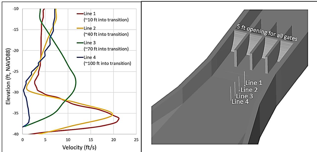
**Figure 6.6-6: Velocities at Various Locations for Partially Opened Gates**
