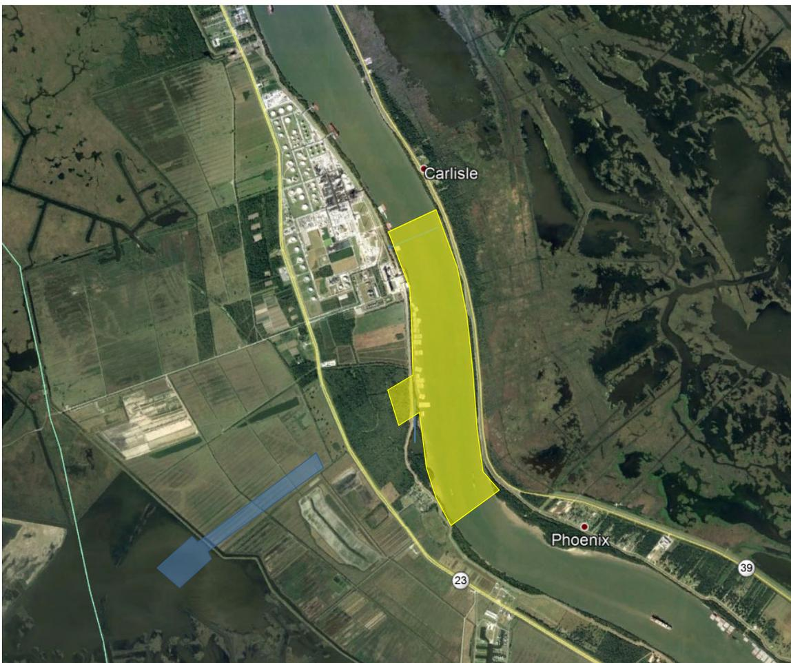
**Figure 3.3-1: Physical Model Domains (diversion intake & Mississippi River model yellow, conveyance model blue)**
