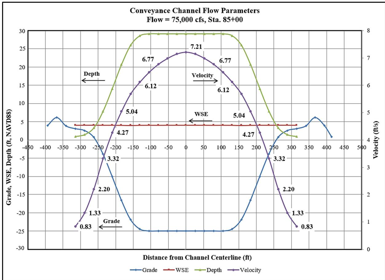
**Figure 6.6-10: Water Surface Elevation, Depth & Velocity at Mid-Channel (Sta 85+00) for Normal Flow Conditions (75,000 cfs) [Velocities are Depth-Averaged Velocities]**
