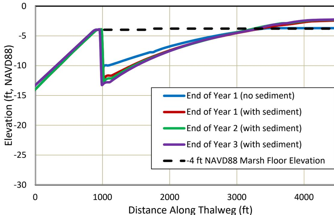
**Figure 3.2-5: Predicted scour bed elevations**
