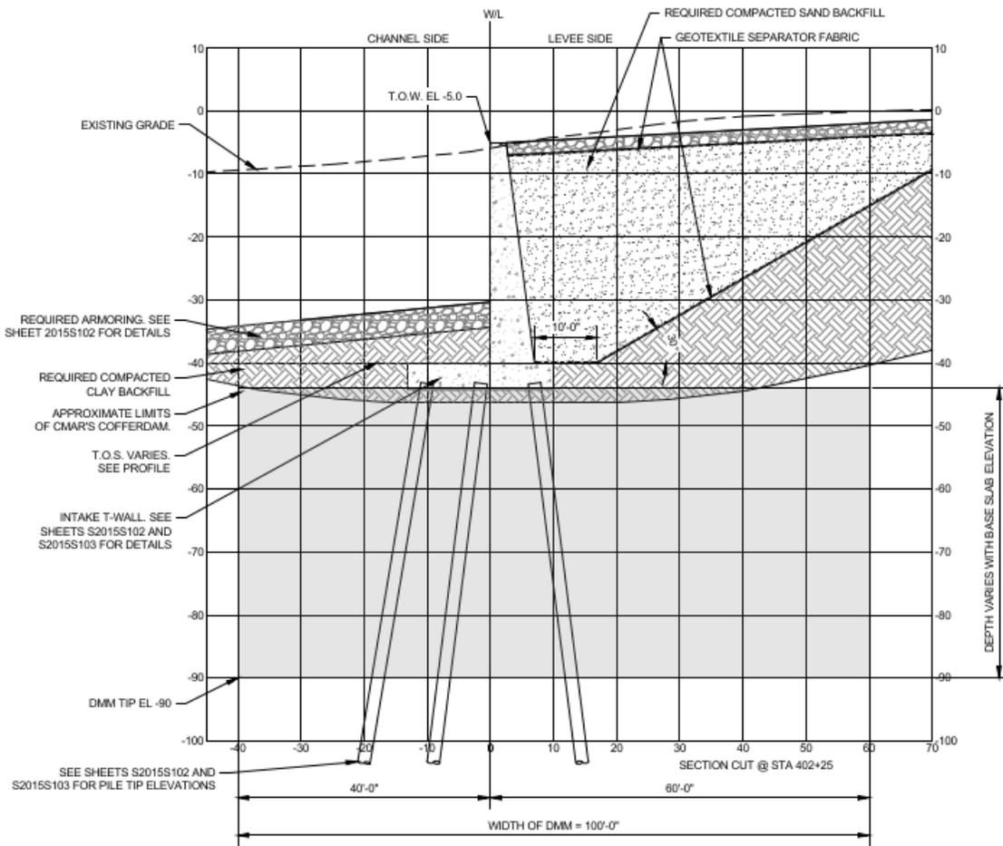
**Figure 5.10-1: Typical Section of T-Wall**
