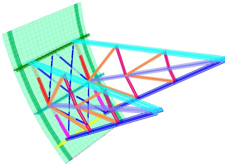
**Figure 5.3-3: 3-D SAP2000 Model of Tainter Gate**
