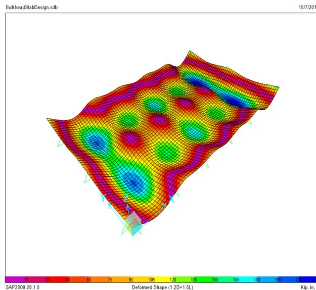
**Figure 3.5-6: Deformed Shape of Factored Live Load in SAP 2000**
