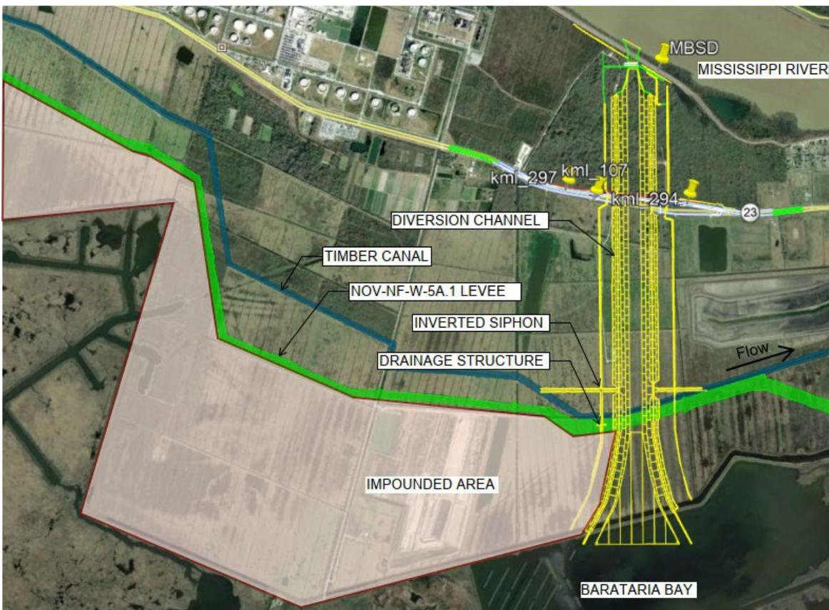
Figure 2.8-6. Proposed Project Drainage Structure and Location of Impounded Area (Polder).
