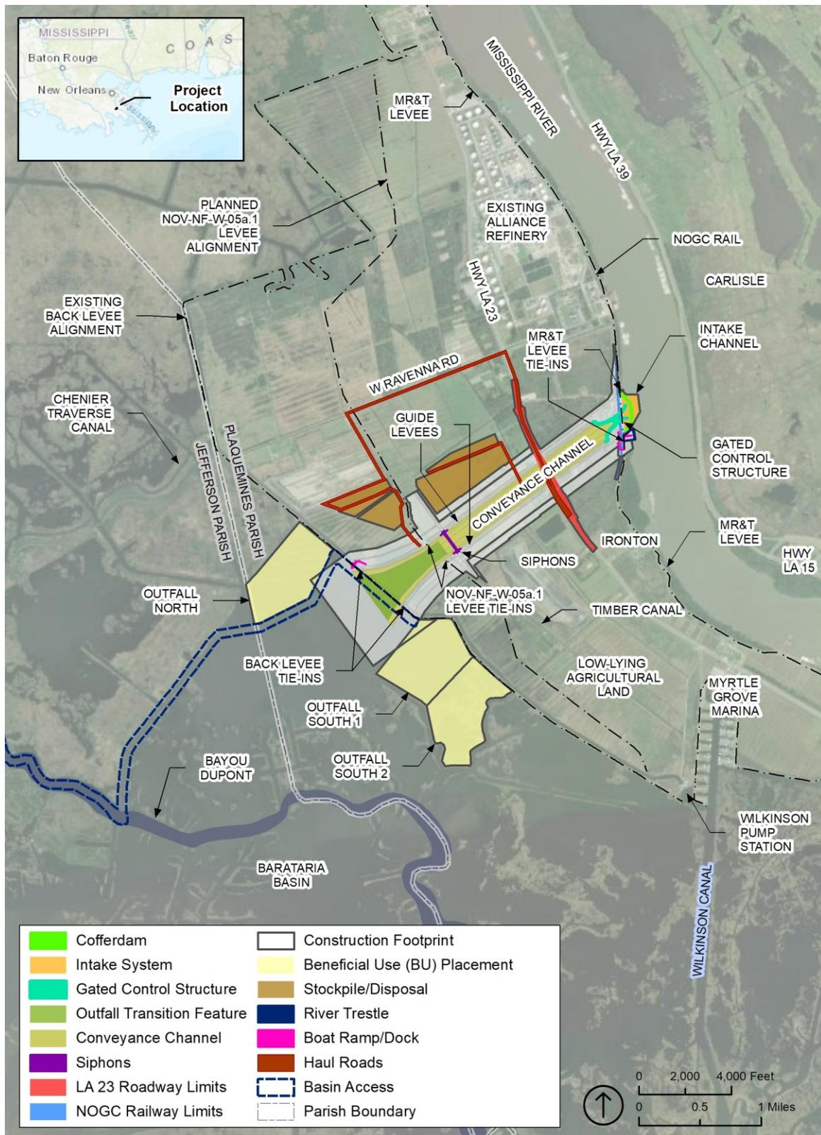
**Figure 2.8-1. Project Design Features and Construction Footprint.** Note that the terraces shown in the figure would only be constructed for the three terrace alternatives.
