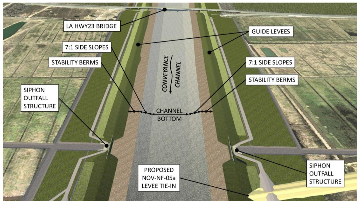
**Figure 2.8-3. Upstream View of the Proposed Conveyance Channel, Guide Levees, Stability Berms, and Siphon.**
