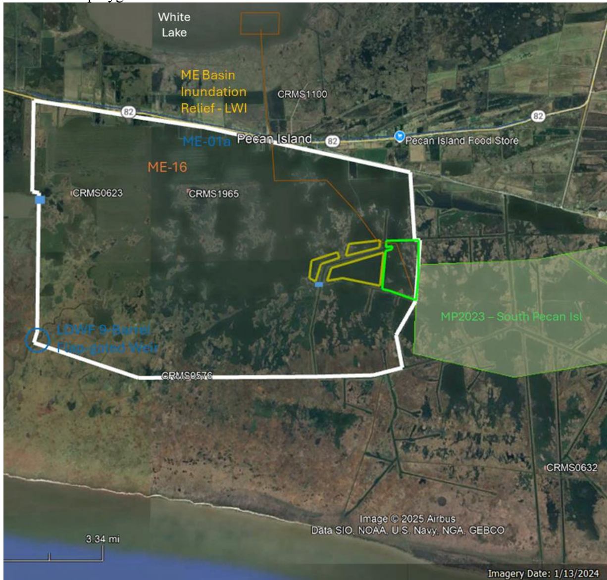
Figure 3 - Site Map with Synergistic Projects. Project Features are a marsh creation unit (green polygon), terraces (gold polygon), and a water control structures (small blue lines). Also included are the synergistic, infrastructure, and landscape features along with the MP 2023 South Pecan Island polygon.
