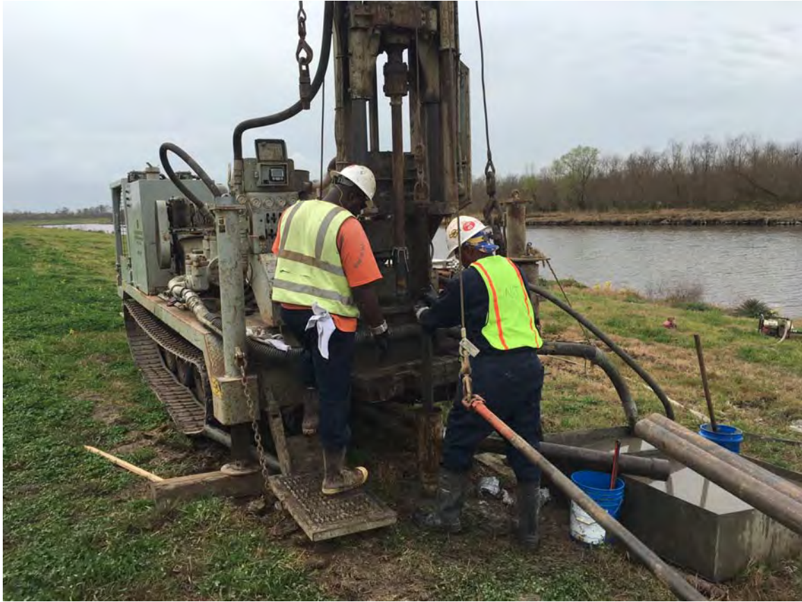
Figure 1: Typical land-based set up during drilling and sampling (track-mounted rig)
