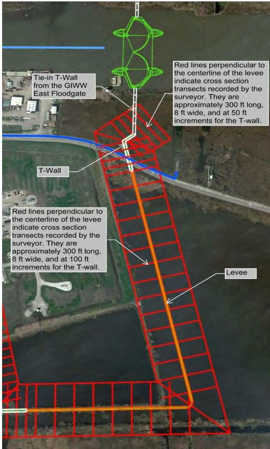
Figure 2.2 – Details of Survey Work Zone for Levee and Short T-wall
