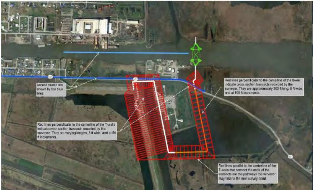
**Figure 4.** Overview of GIWW East Floodgate Proposed Floodwall and Levee Alignment Survey Work Zone
