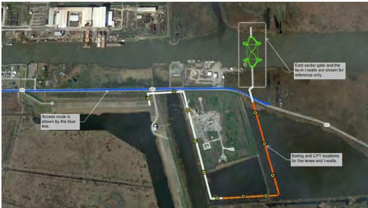
**Figure 5.** Overview of GIWW East Floodgate Proposed Floodwall and Levee Alignment Boring Locations
