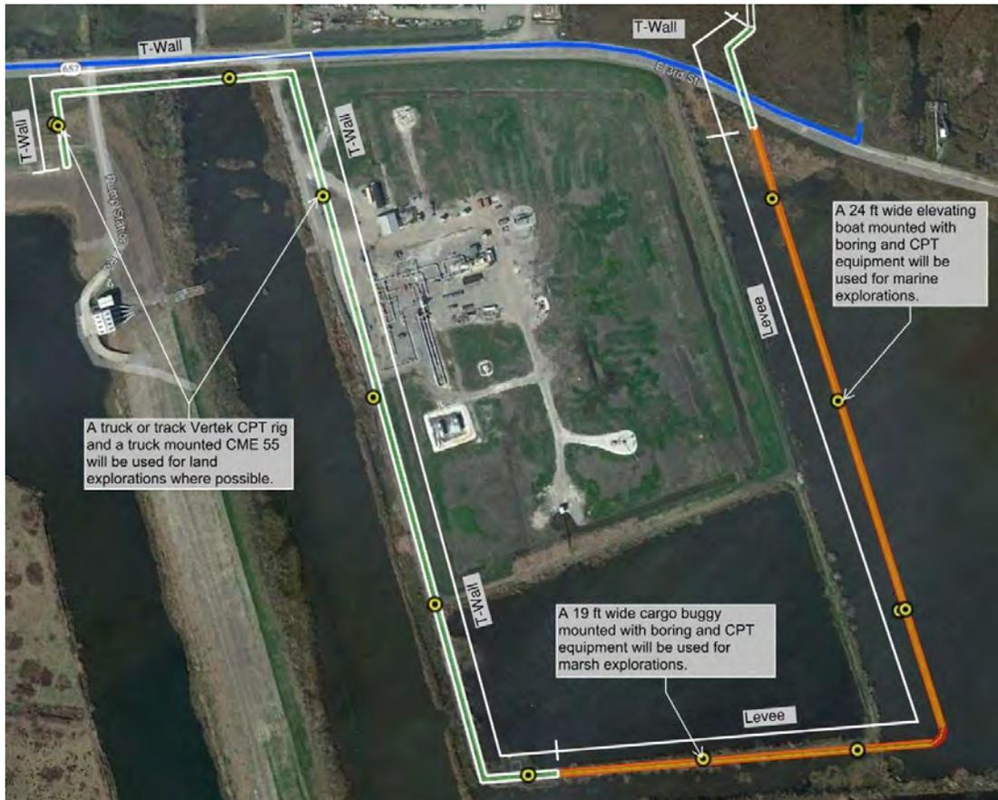
Figure 2.5 – Details of Boring Work Zone
