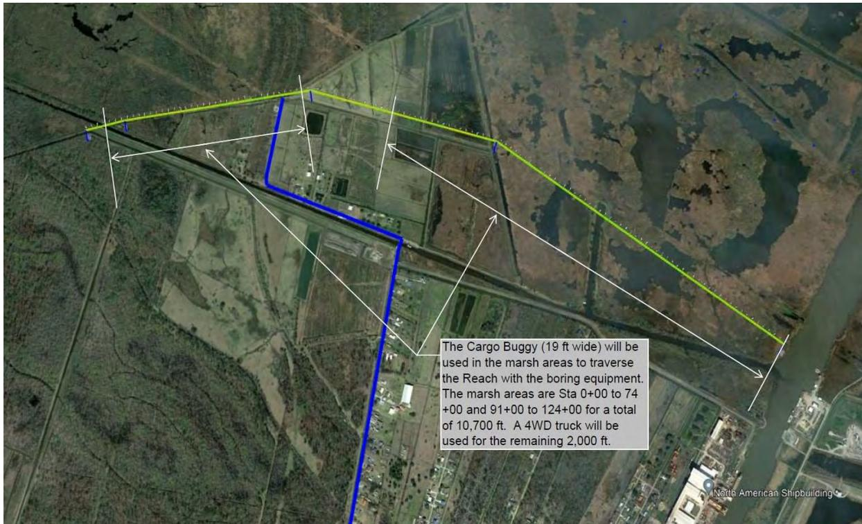
Figure 11.4 – Overview of Boring Locations by Equipment Type
