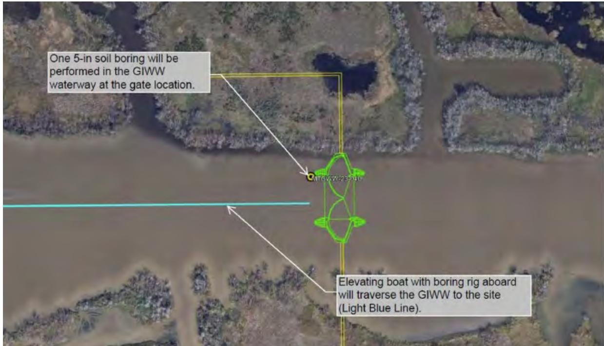
**Figure 7.** Overview of GIWW West Floodgate Boring Locations
