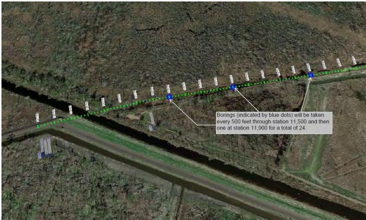
Figure 11.5 – Details of Boring Work Zone
