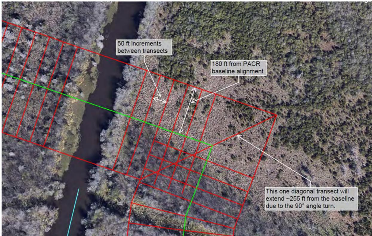
Figure 6.2 – Details of Survey Area
