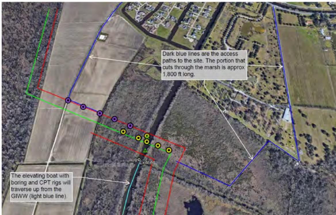
**Figure 13.** Overview of Minors Canal Floodgate (PACR Alignment) Boring Locations
