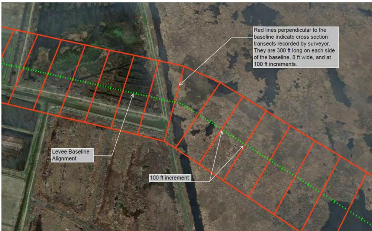
Figure 11.2 – Details of Survey Work Zone
