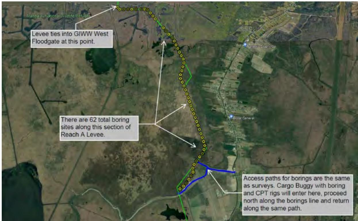
**Figure 9.** Overview of Reach A Levee – South of the GIWW (PACR Alignment) Boring Locations
