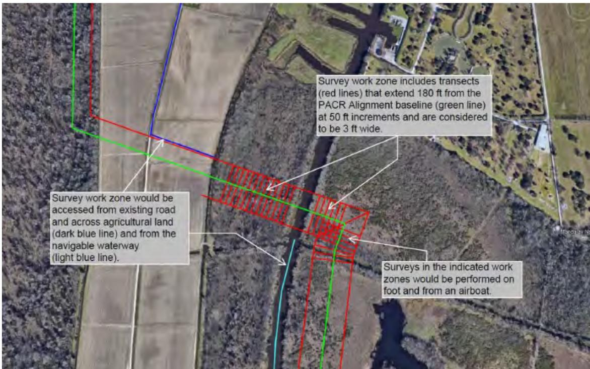
**Figure 12.** Overview of Minors Canal Floodgate (PACR Alignment) Survey Work Zone
