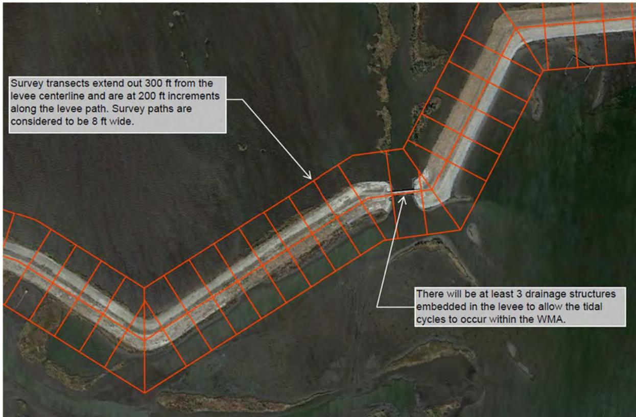
Figure 10.2 – Details of Survey Area
