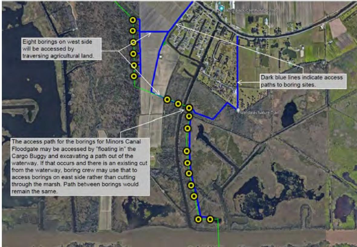
**Figure 11.** Overview of Reach A Levee – North of the GIWW (PACR Alignment) Boring Locations
