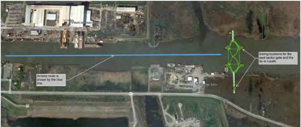
**Figure 3.** Overview of GIWW East Floodgate Boring Locations
