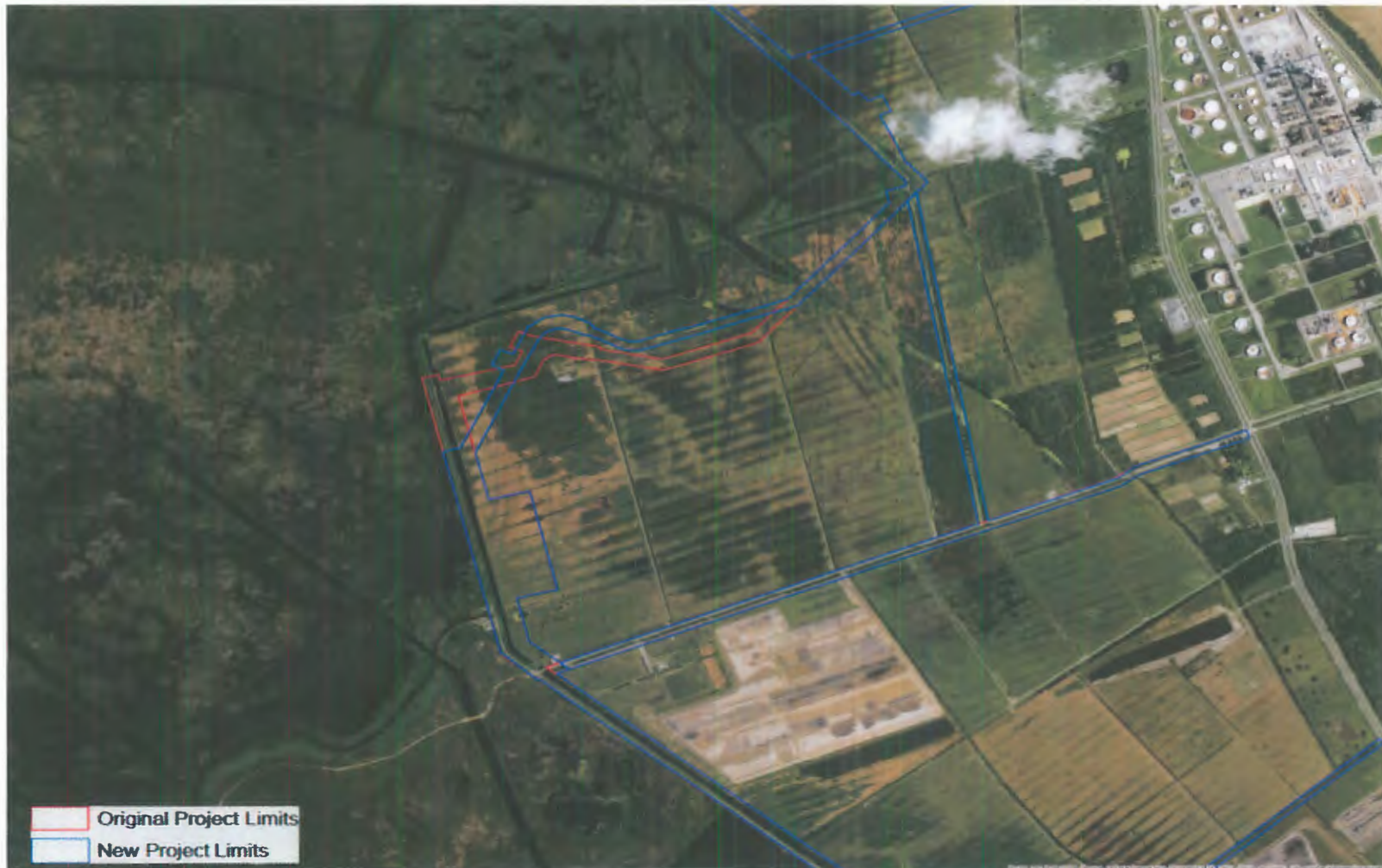
Figure 3. NOV-NF-W-05a.1 in the NFL Section 2, redlines depict the original levee alignment, blue lines depict new ROW for levee and floodwall alignment.
