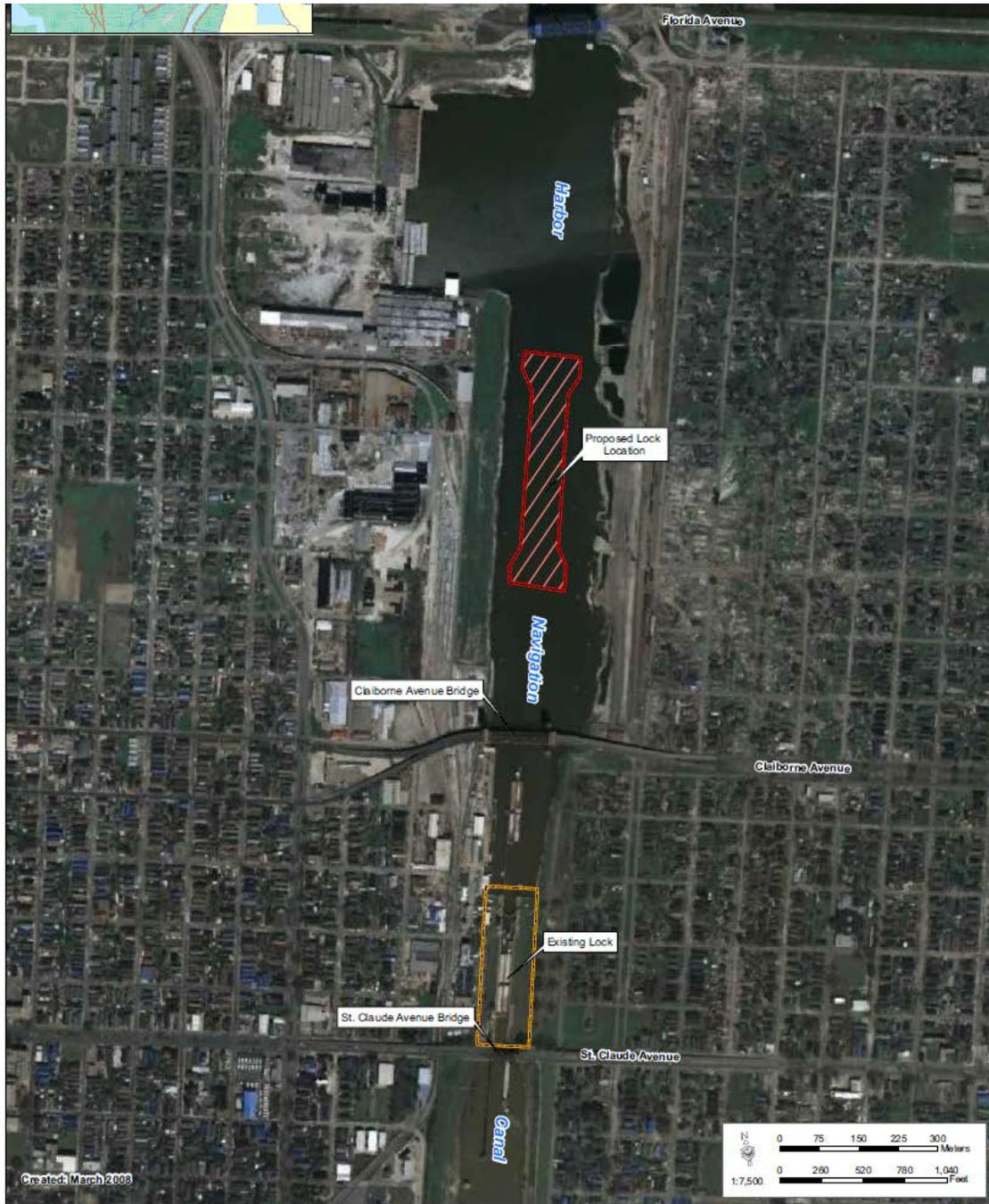
Figure 3 below shows proposed lock location – cofferdam (red) and bypass channel (yellow).
