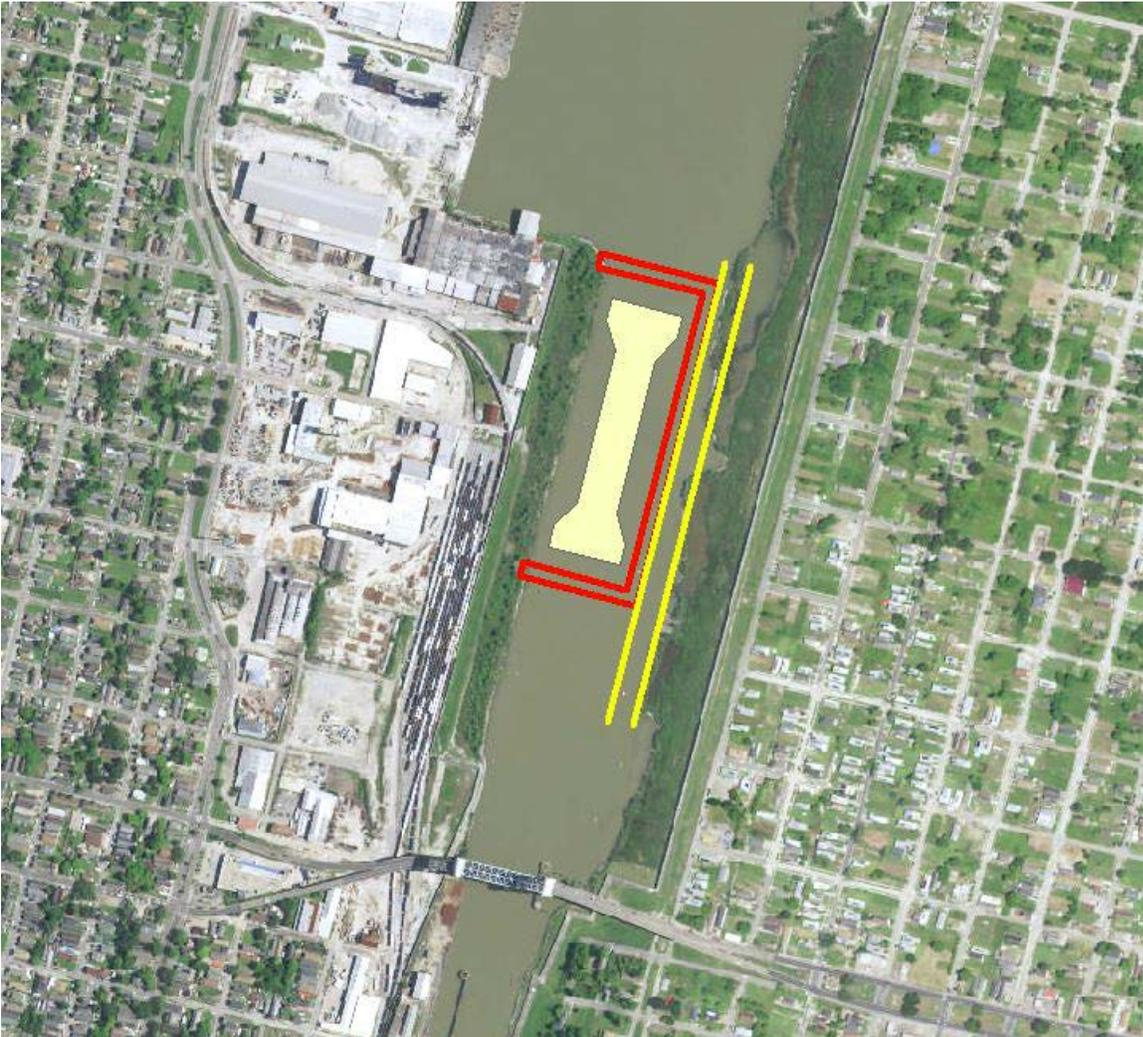
Figure 4 below shows existing lock location – temporary bridge (red), new flood risk reduction measures (green) and bypass channel (yellow).
