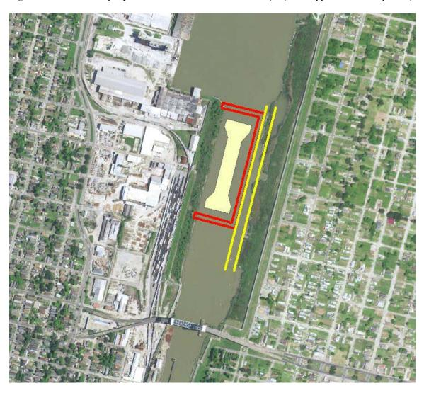
Figure 3 below shows proposed lock location - cofferdam (red) and bypass channel (yellow).
