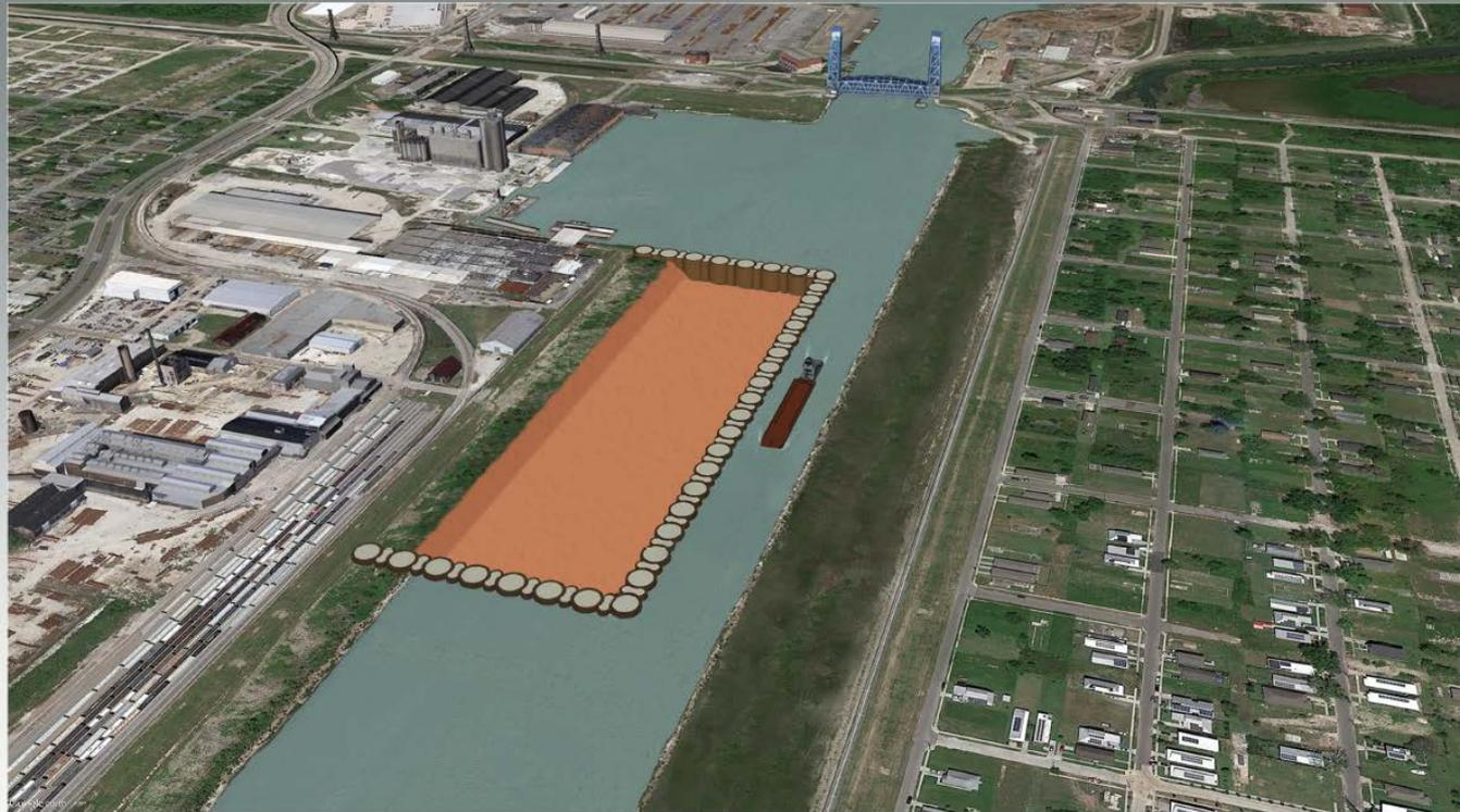
Temporary bypass channel with cofferdam dewatered and excavated.
