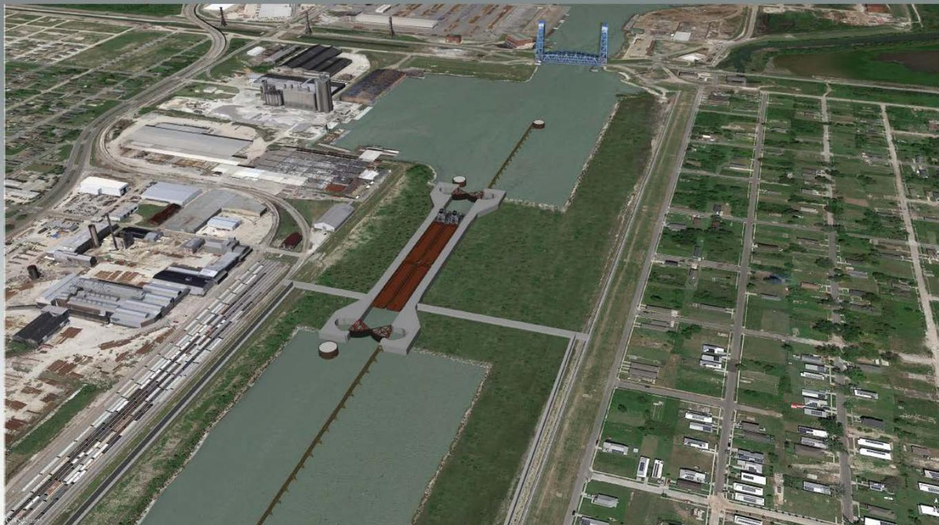
New 900 feet long by 110 feet wide IHNC Lock, with a sill elevation of -22.0 feet NAVD88.
