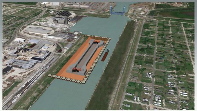
Cofferdam with sector gate and lock constructed.
