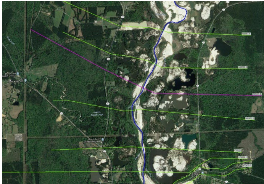
Figure H-14 Lateral Inflow Location Representing Flow from Bluff Creek into the Amite River
