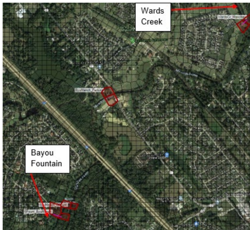
Figure H-23 Cross Sections where Ward Creek and Bayou Fountain EBR Flows Were Applied
