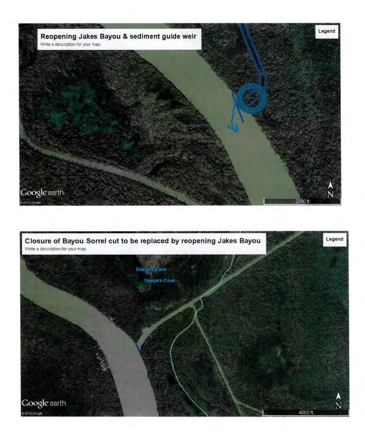
Bayou Chene restoration. Bayou Chene cut closure, restoring old Bayou Chene, sediment guide weir and sediment trap.
