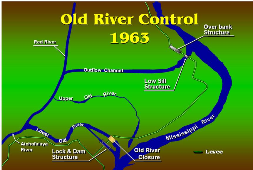
The Old River control structures were to be operated so as to maintain the distribution of flow and sediments between the lower Mississippi River and the Atchafalaya River in approximately the same proportions as occurred naturally in 1950. That distribution was determined to be approximately 30 percent of the total latitude flow (combined flow in the Red River and Mississippi above the control structures) passing down the Atchafalaya River on an annual basis.
