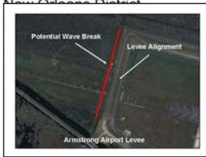
Here is the Armstrong Airport Levee. The problem here is that there are airplane lights, and we're trying to fit a levee in between the lights and not interfere with the lights. We're looking at different options and we're working with the airport.
