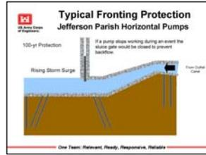
controlled at its head by a gate).
