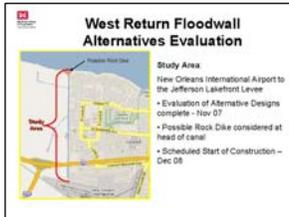
This is the West Return floodwall, and it's about 3.5 miles long. Eighty percent of it is an inverted T-wall. There are sections of it that have just a sheet pile wall. It extends from the airport to Lake Pontchartrain. It ranges from 12 1/2 to 15 feet in height. We've done evaluations on the different alternatives and we're looking at the possibility of putting a rock dyke there
