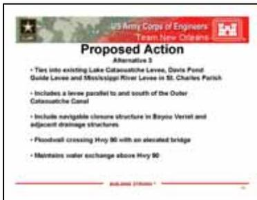
This is a written explanation of what I discussed in the last slide. The proposed alternative ties into the Mississippi River levees. It maintains the water exchange above Highway 90 to make sure we are avoiding some impacts. This navigable closure structure in Bayou Verret would stay open most of the time. The size would be wide enough and will maintain the same water flow. There will be additional openings to the structure because we are not restricting or reducing the area.
