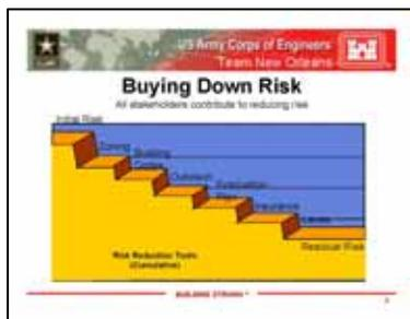
We like to use this slide to tell the public how risk is bought down in the greater New Orleans area. We have identified an initial risk for the area, but by taking these steps we can buy down risk. Constructing levees and floodwalls are the last step on this staircase but in the end there is still residual risk. We can not eliminate risk but we can buy it down.
