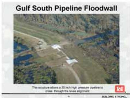
At the Gulf South Pipeline, which is a 30 inch high pressure line that goes in this direction right here, perpendicularly through this floodwall. At this location we are just going to be replacing the existing floodwall.
