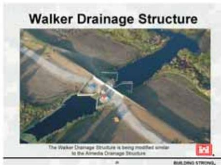
This is the Walker Drainage Structure. It looks a lot like Almedia Structure. We are going to do the exact same thing here. We are modifying the existing structure and you can see they are not quite as far along with this one yet. They have torn out the existing tie-in walls and they are driving new sheet piles cutoffs to keep water from
