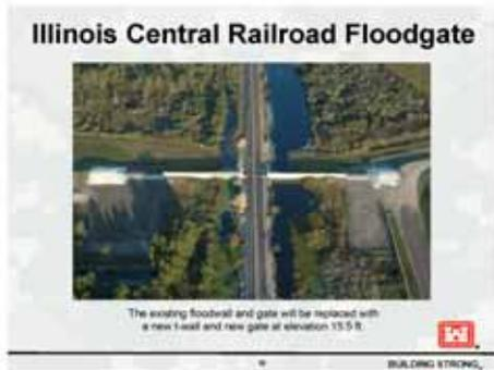
Our last structure here is going to be the Illinois Central Railroad Floodgate. This is just a floodwall that has gate in it that allows Illinois Central's main line here to pass through all hurricane protection alignment. We are going to be tearing out the existing floodwall and building a higher and stronger T-wall to an elevation of 15.5 feet.
