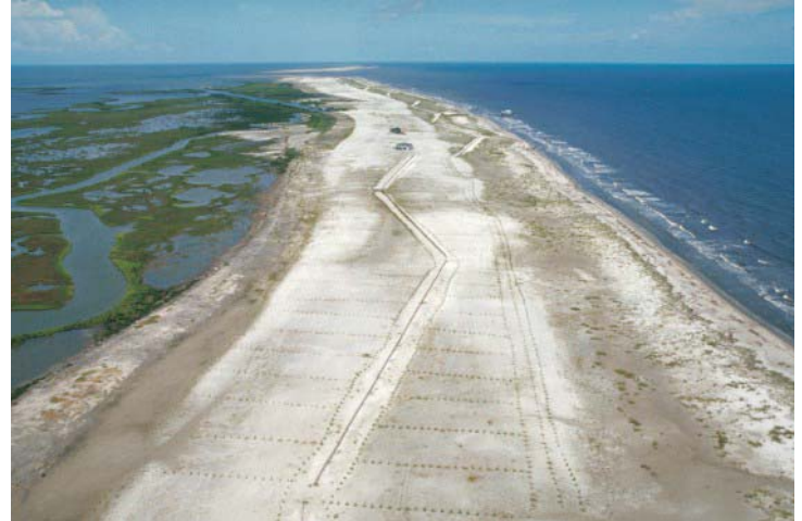
Sediment was pumped to restore 3.2 miles of the island, which was then revegetated. Sand fencing was later added to aid sediment retention.
