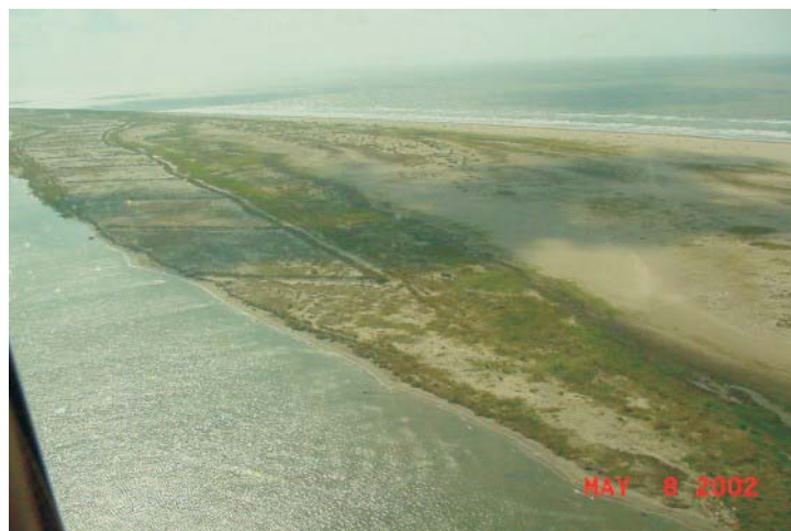
Aerial view of sand fencing and vegetative plantings on East Island.
