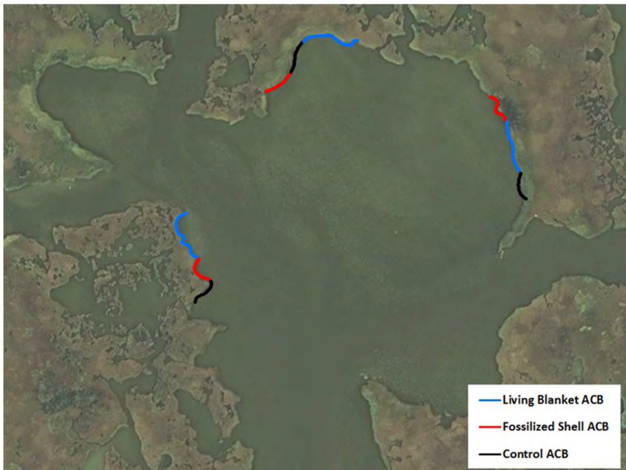
Figure 1: Not-to-scale example of Living Blanket demonstration layout. Each of three articulated concrete block (ACB) mat treatments (Living Blanket ACB, Fossilized Shell ACB, and Control ACB) has three replicates.
