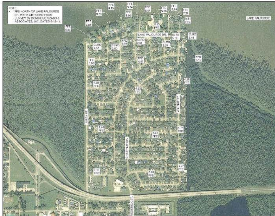
Figure B:3-21. Map Showing Ground Surface Elevations along Lakeshore Area
