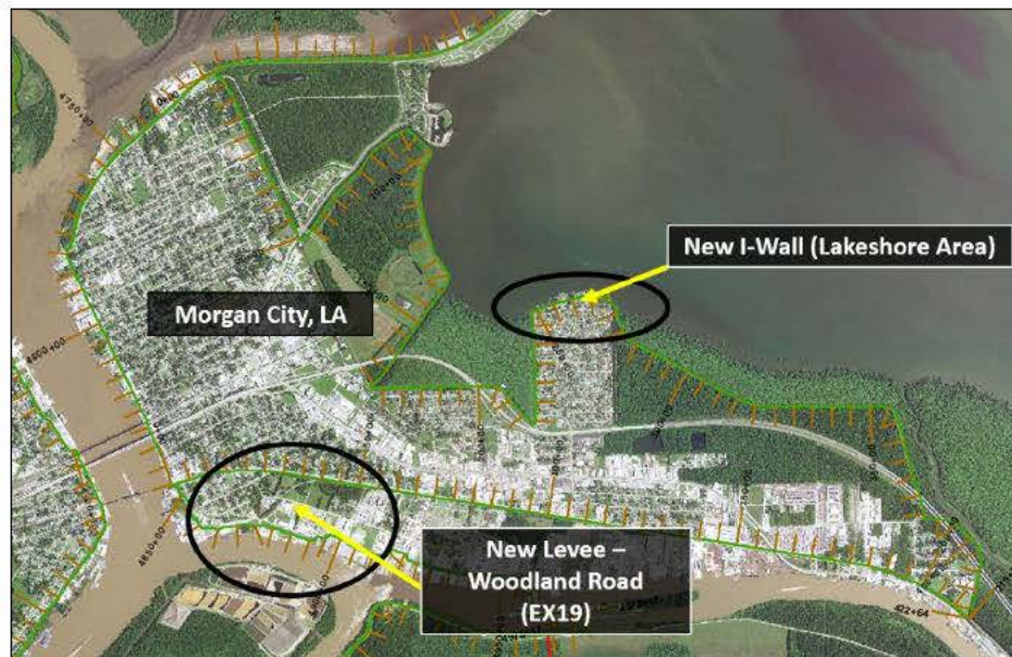
Figure B:3-19. Map Showing Proposed Work Areas for Measure 6 Alternative
