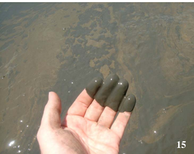
Pictures 14-16. Dredged material within the upper boundary of Placement Area #2 was predominantly fine-grained sediments mixed with organic material.
