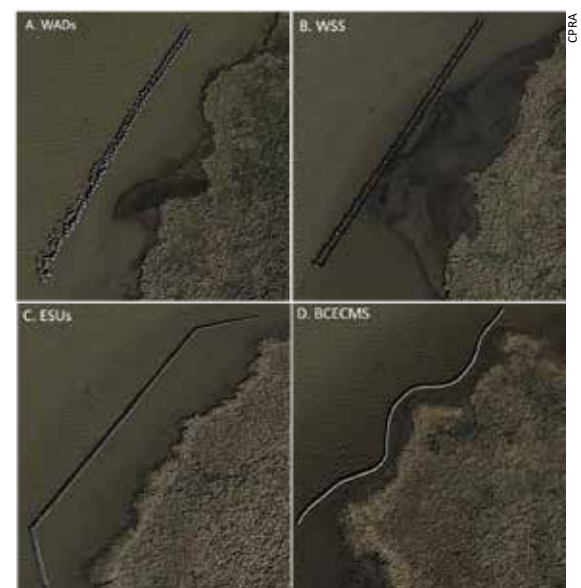
Figure 24. A close up image of each section of structures shows a better view of mudflat formation behind the WADs and WSS.
