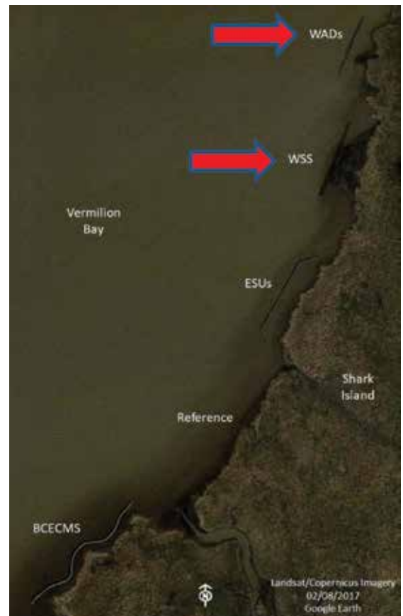
Figure 23. Aerial imagery during low water levels about 3 years after installation of LA-16 structures. Note mudflat formation behind the porous WADs and WSS.
