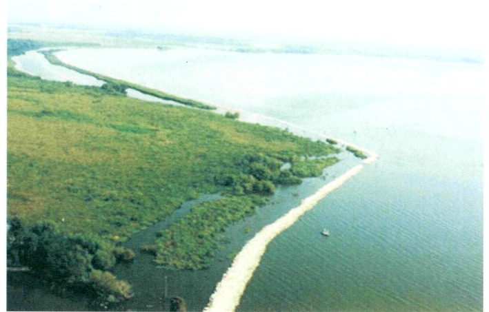
A foreshore rock dike, such as the one shown above, may provide an alternative type of shoreline protection to the eastern shoreline of East Cote Blanche Bay.
