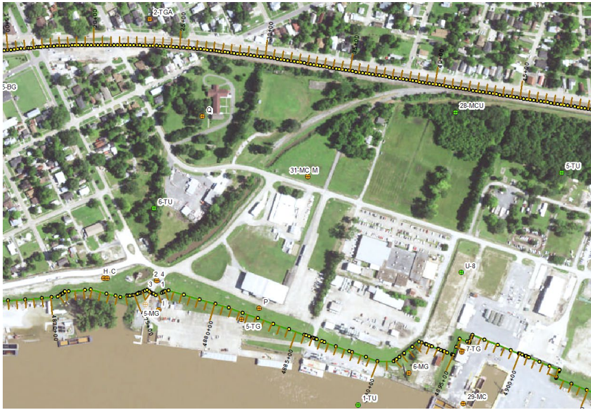
Figure 26. Map showing BNSF Railway embankment and Atchafalaya Basin levee alignments. Nearby boring locations are also shown.
