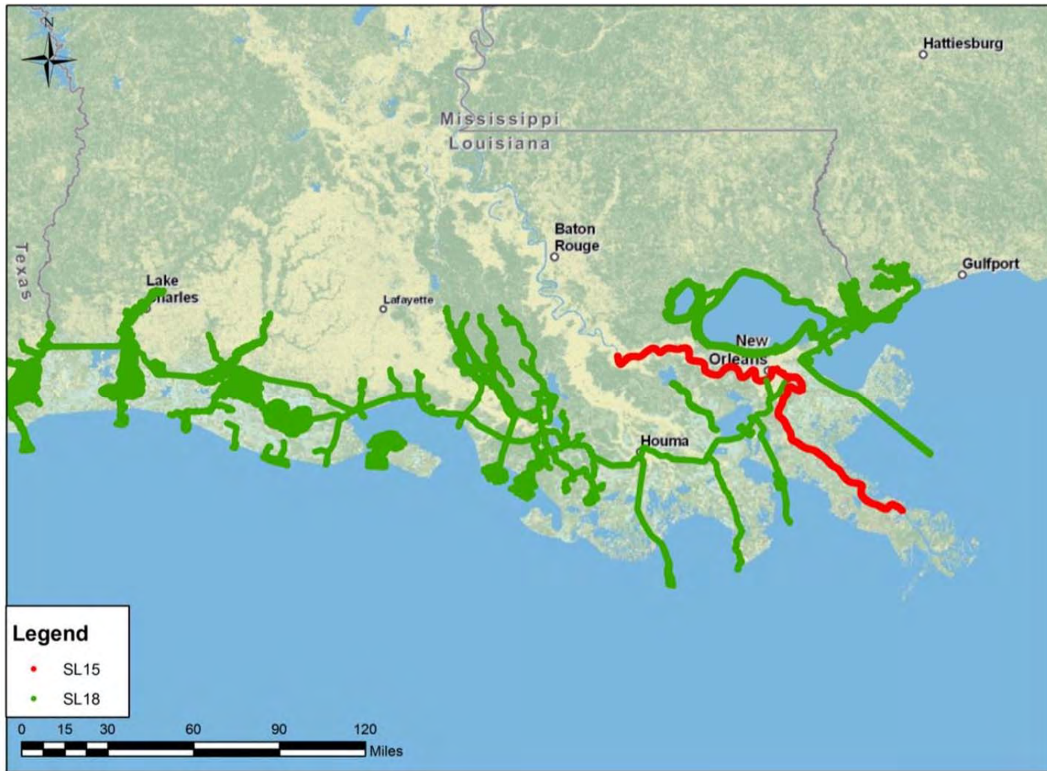
Figure 12: Bathymetric features, including channels, dredged channels, and other inland water bodies, defined using SL18 and SL15 nodal locations and elevations.
