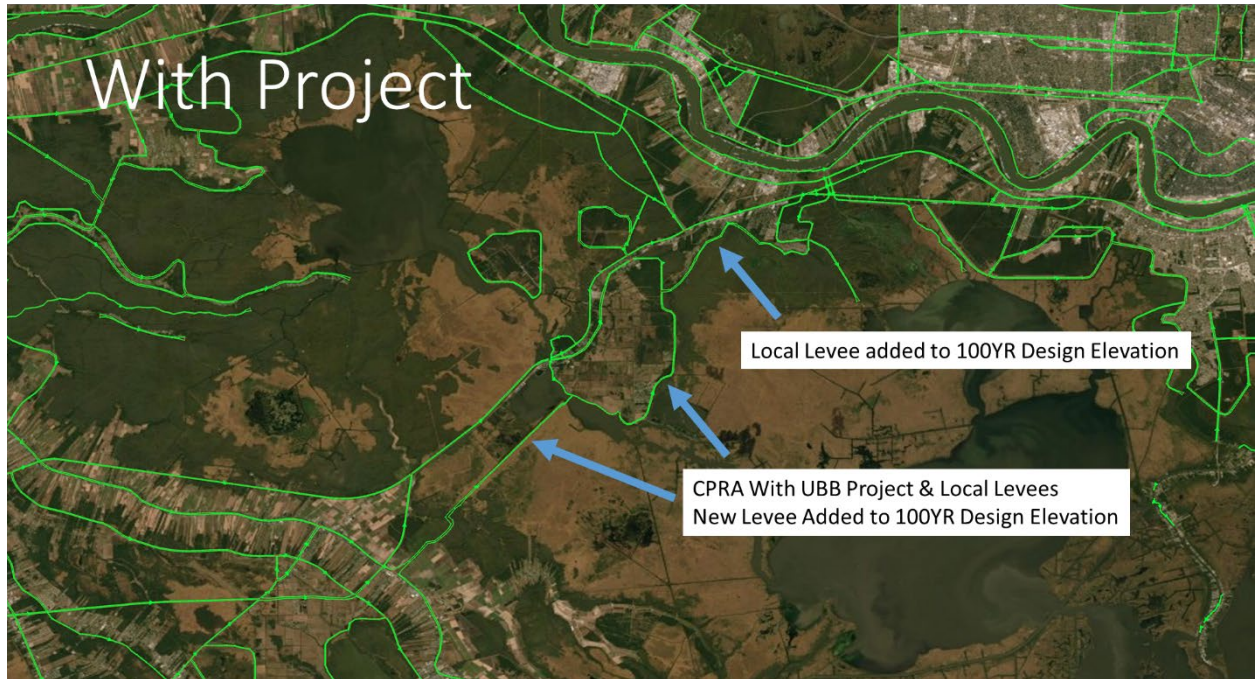
Figure 3 With project - levees and raised feature alignments
