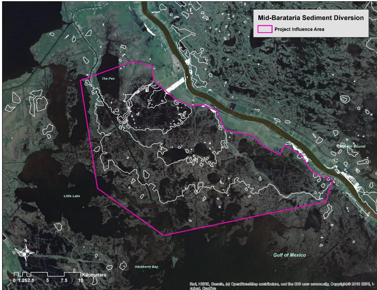
Fig. 3.3-3. A Project Influence Area (magenta polygon) was defined around the Project outfall as the maximum extent of the area where the Delft Basin-wide Model projected water level differences of at least 0.5 meters (white lines) between the Future without Project and the 75,000-cfs Applicant’s Preferred Alternative without terraces. The water level differences shown are specifically for the third week of May during the first decade modeled, using a 2011 Mississippi River hydrograph.
