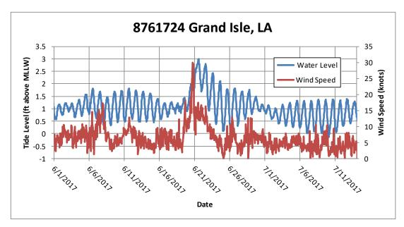
**Figure 3.4-3. Water Level and Wind Speed at the Grand Isle, LA Station.** USGS gages and CRMS stations throughout the Barataria Basin report daily or hourly water levels, most of which are referenced to the NAVD88 datum (USGS 2017d, CPRA 2017b). As shown in Table 3.4-1, average water levels within the Barataria Basin are generally about 1 foot.
