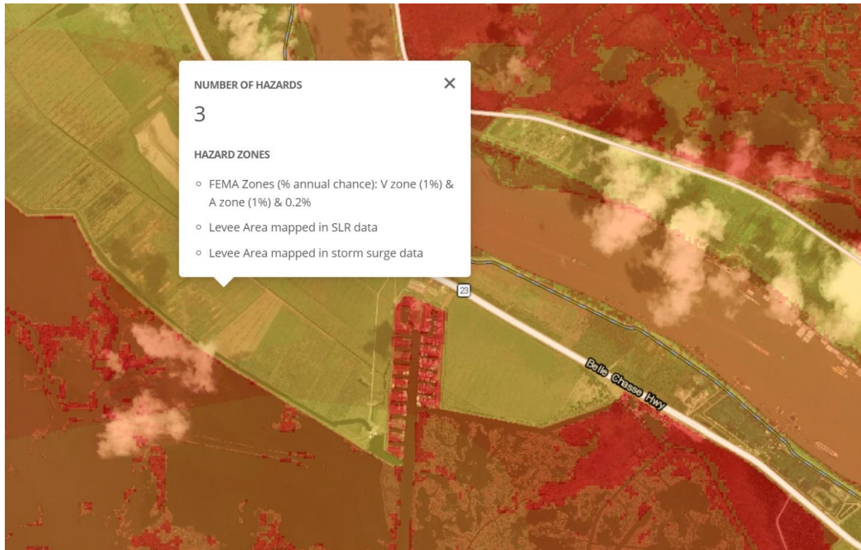
Figure 6d. An example of agricultural polderlands that may be inundated with the Project, located within the Plaquemines Parish back levee. Under current conditions, the back levee is subject to breaching and overtopping and subsequent inundation of the polder when low intensity tropical storms with onshore winds that produce water levels > 3.5 ft. Image and data from the NOAA Coastal Flood Exposure Mapper.
