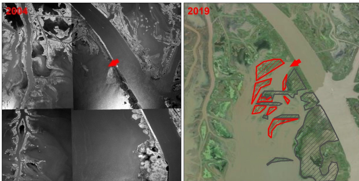
Figure 4.2-10. Google Earth Imagery Depicting Progression of Landform Development in the Vicinity of the West Bay Diversion between 2004 (left) and 2019 (right). Diversion opened in 2003. Red arrow indicates diversion mouth. Note development of small deltaic crevasse splay systems as identified within the red hatching on right. Some material visible in 2019 identified by gray hatching was deposited as beneficial use placement from dredging and not by processes associated with diversion (Google Earth Imagery 2004 and 2019) (Plitsch 2017).
