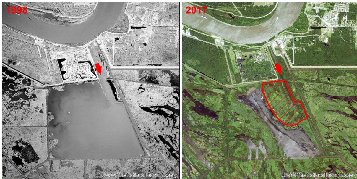
Figure 4.2-9. Google Earth Imagery Depicting Progression of Landform Development in the Vicinity of Caernarvon Diversion, in the Big Mar Receiving Basin between 1998 (left) and 2017 (right). Diversion opened in 1991. Red arrow indicates diversion mouth. Note development of small deltaic system as identified within the red hatching on right. Some material to the southwest in Big Mar was deposited as a result of Hurricane Katrina in 2005, and not by diversion operations.
