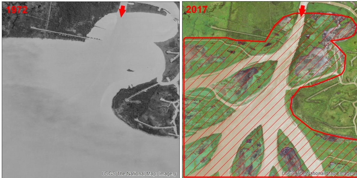
Figure 4.2-8. Google Earth Imagery Depicting Progression of Landform Development in the Wax Lake Outlet Delta between 1972 (left) and 2017 (right). Outlet opened in 1942. Red arrow indicates outlet mouth. Note extensive development of bifurcating channels, deltaic crevasse splay systems, and emergent marshes between 1972 and 2017, as identified within the red hatching on the right panel.
