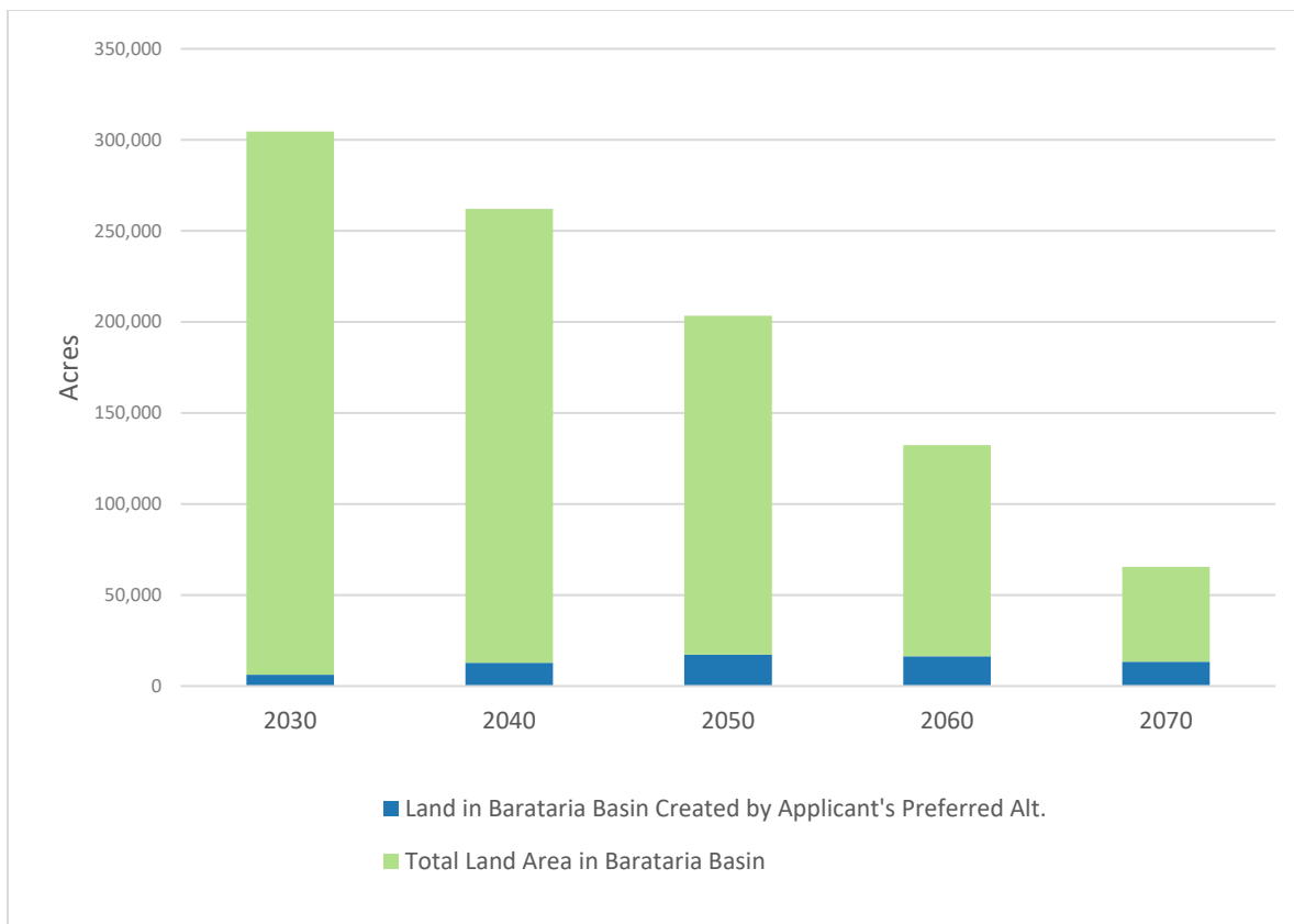
Figure 4.2-6. Model-projected Land Area in the Project Area in the Barataria Basin under the Applicant’s Preferred Alternative, and Fraction of the Remaining Area due to the Proposed Project.
