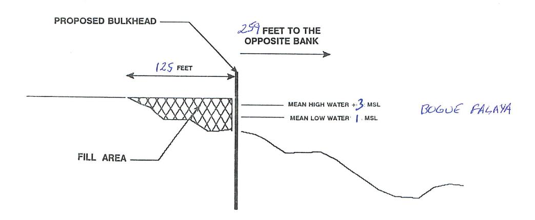
APPROXIMATELY % CUBIC YARDS OF SAND WILL BE HAULED IN FROM A COMMERCIAL SOURCE TO BE USED AS FILL BEHIND THE PROPOSED BULKHEAD
