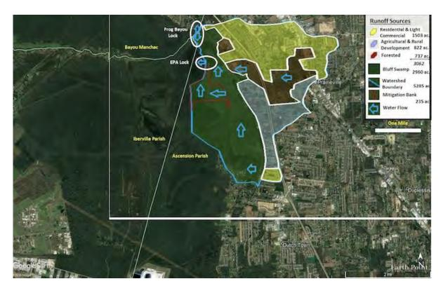
Figure C7. Current hydrologic conditions. An estimated 3,062 acres of Pleistocene terrace drain into a similar area (2960 acres) of Bluff Swamp. The Bluff Swamp watershed westwardly drains into Alligator Bayou through the EPA Locks. Exchange with Bayou Manchac takes place at the Frog Bayou Lock.
