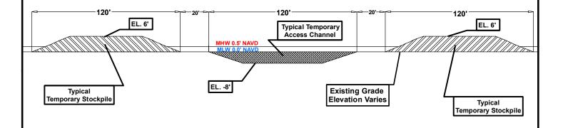
Phase I Stockpile Existing Grade Elevation Varies ~(-1)' to ~(-7)' Phase II Stockpile Existing Grade Elevation Varies ~(-3)' to ~(-10)'
