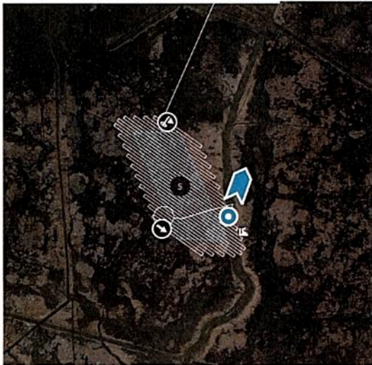
Figure 4: Flight path of fixed wing UAS aerial data collections in Terrebonne Basin that produced 2.5cm visible light and near infrared imagery. (Image credit: Jesco Environmental)
