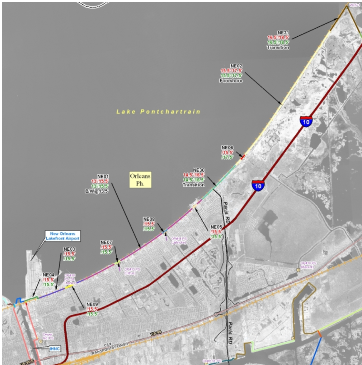
Figure 32 – Levee and floodwall sections in Orleans Parish Lakefront East. The numbers represent existing/future conditions and are without (red) and with (green) structural superiority.
