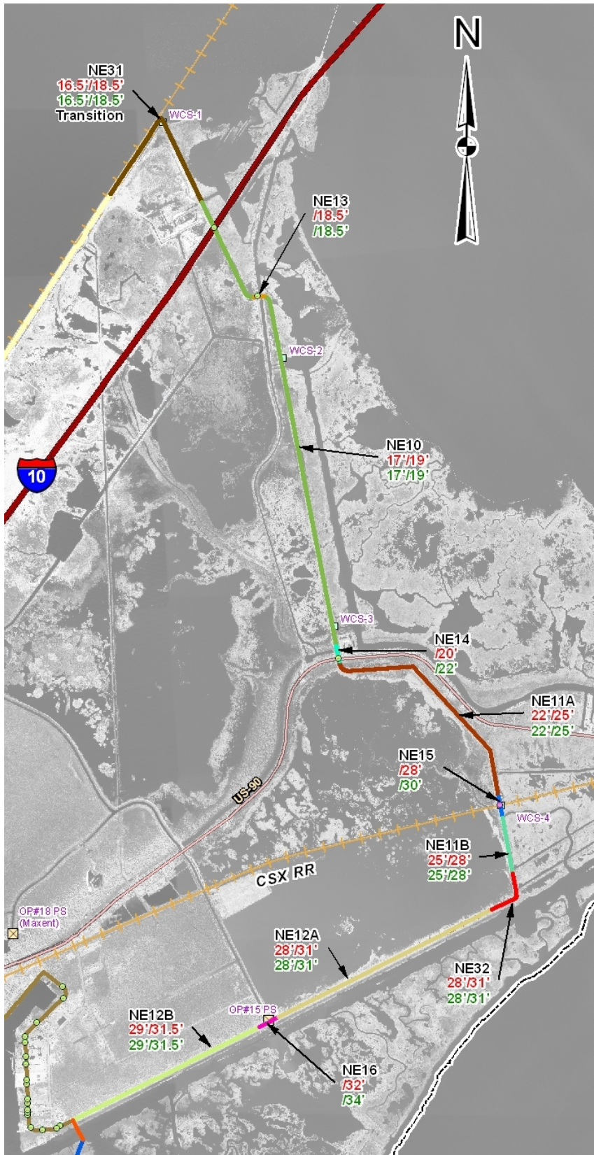
Figure 39 – Levee and floodwall sections in GIWW area. The numbers represent existing/future conditions and are without (red) and with (green) structural superiority.
