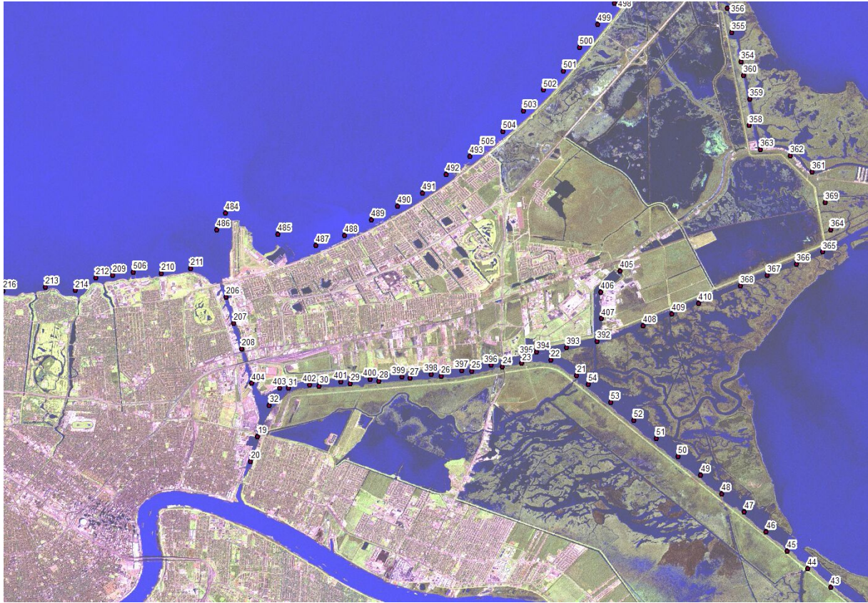
Figure 17 – MRGO levee with output points from ADCIRC and STWAVE (point 35 – 54 and 21 - 22)
