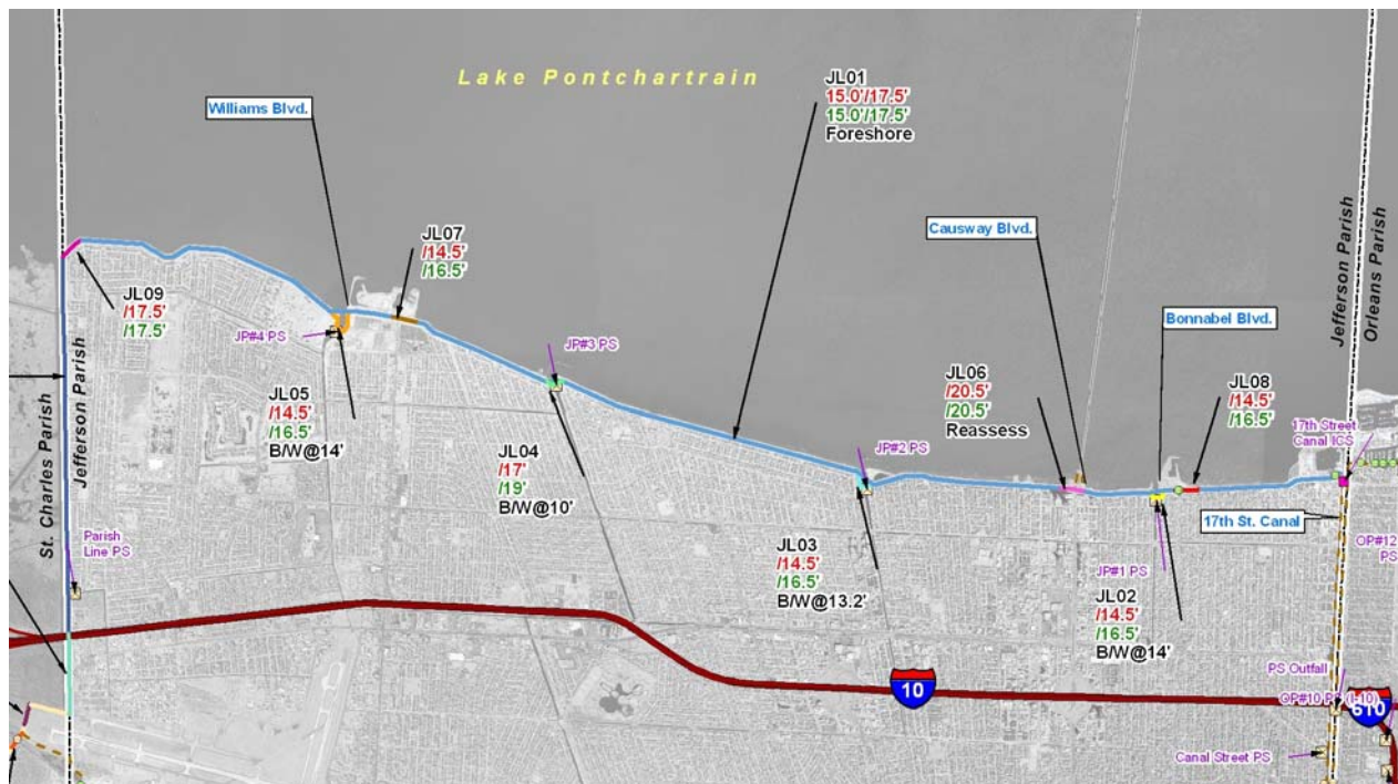
Figure 26 – Levee and floodwall sections in Jefferson Parish lakefront. The numbers represent existing/future conditions and are without (red) and with (green) structural superiority.
