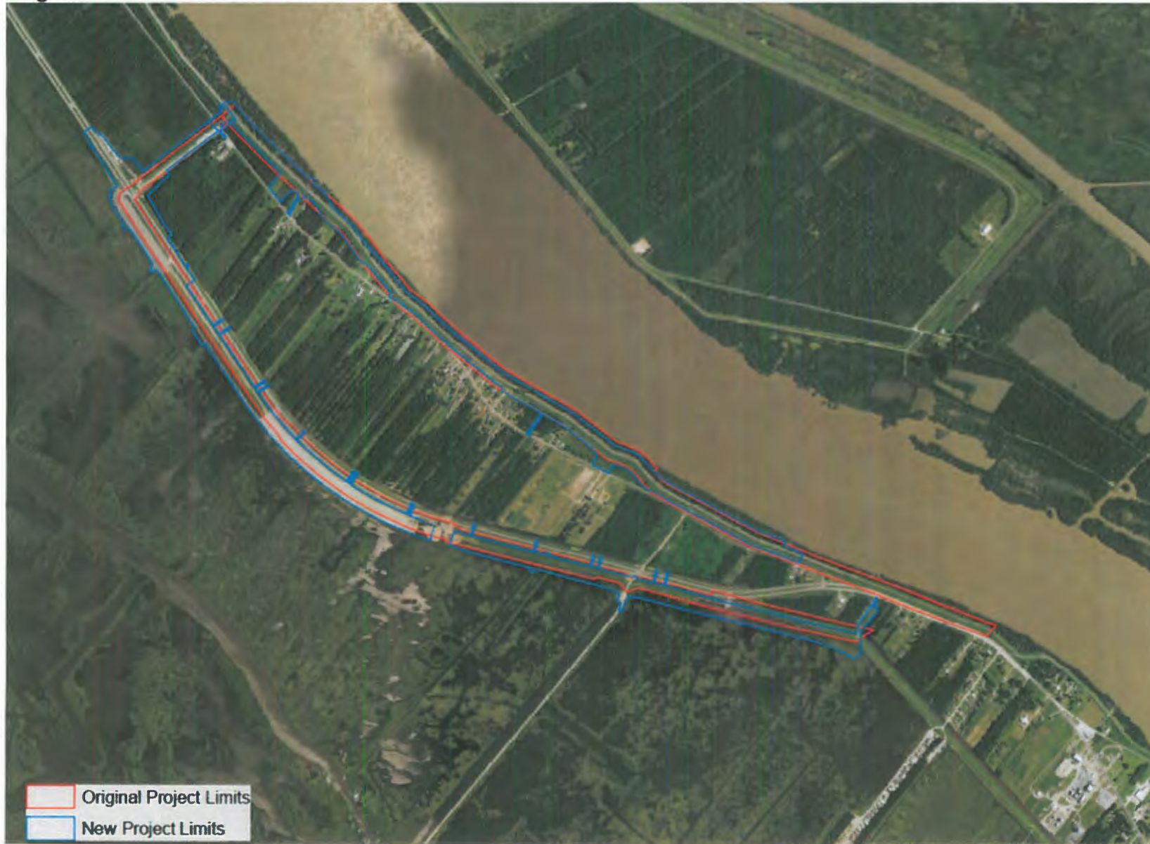
Figure 2. NOV-09 is the northern section of levee; NOV-05A is the southern section of levee. Red lines depict original ROW and blue lines new ROW.
