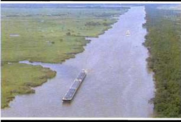
An alternate connection from the Mississippi River to the Gulf Intracoastal Waterway is provided by an improved 12- by 125-foot channel from Port Allen to Morgan City. At Port Allen, opposite Baton Rouge, a navigation lock 1,200 feet long and 84 feet wide provides passage through the west bank levee system to the Intracoastal Waterway.
