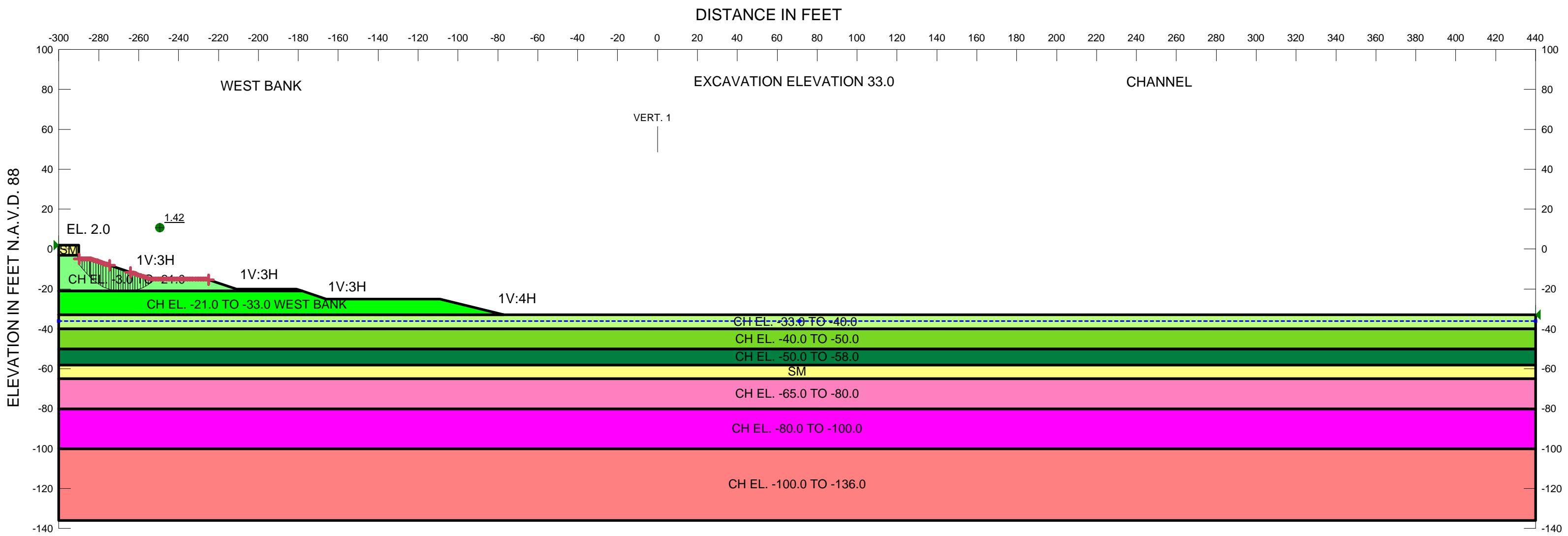
Name: CH EL. -21.0 TO -33.0 WEST BANK Model: Mohr-Coulomb Unit Weight: 100 pcf Cohesion: 400 psf Phi: 0° Piezometric Line: 1
