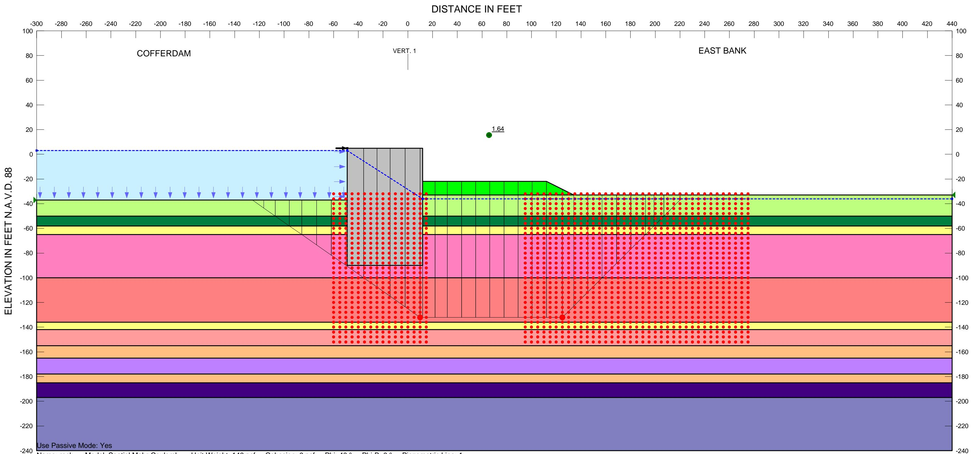
Name: rock Model: Spatial Mohr-Coulomb Unit Weight: 140 pcf Cohesion: 0 psf Phi: 40° Phi-B: 0° Piezometric Line: 1
