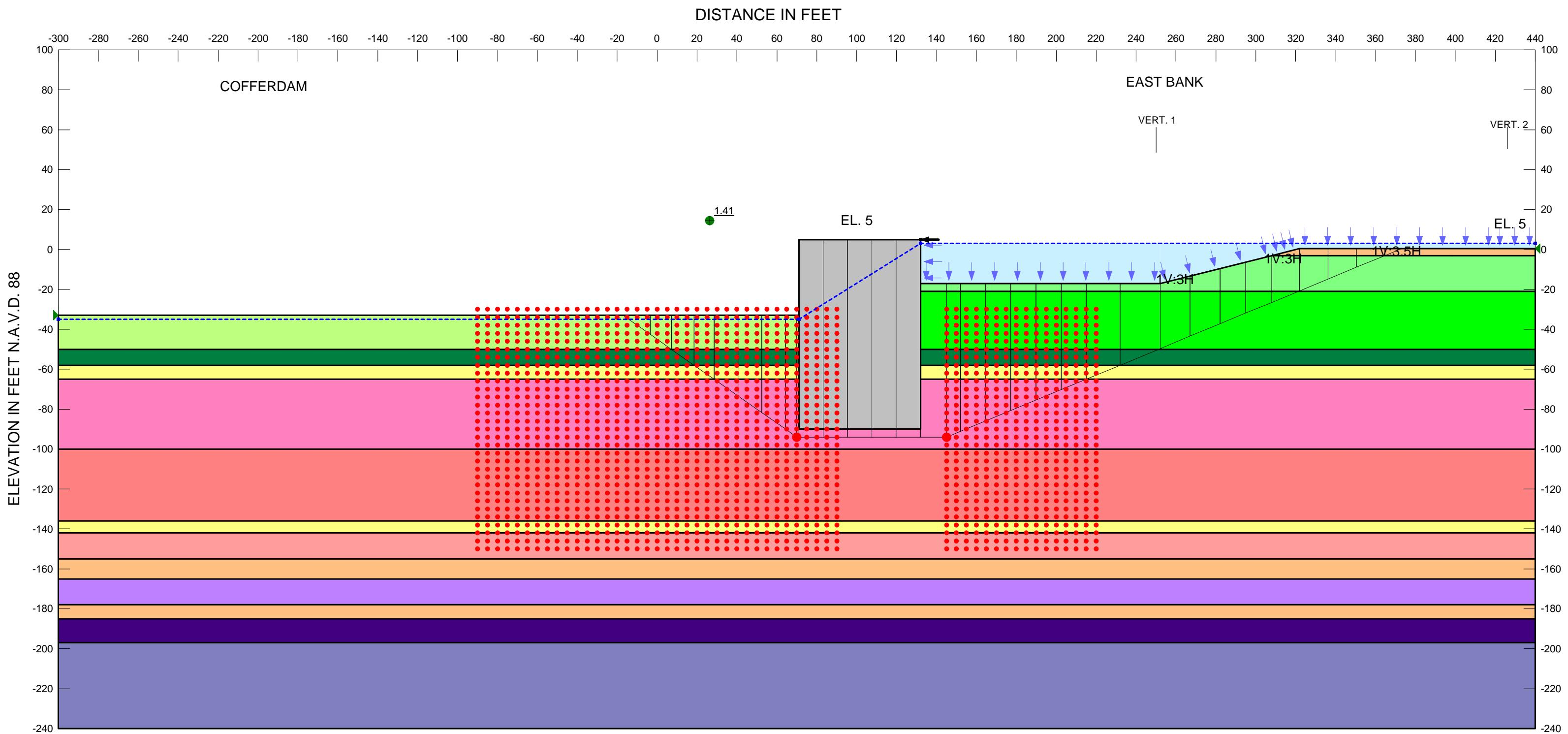
Name: CH EL. -21.0 TO -50.0 EAST BANK Model: Spatial Mohr-Coulomb Unit Weight: 100 pcf Cohesion Spatial Fn: CH EL. -21.0 TO -50.0 Phi: 0° Piezometric Line: 1
