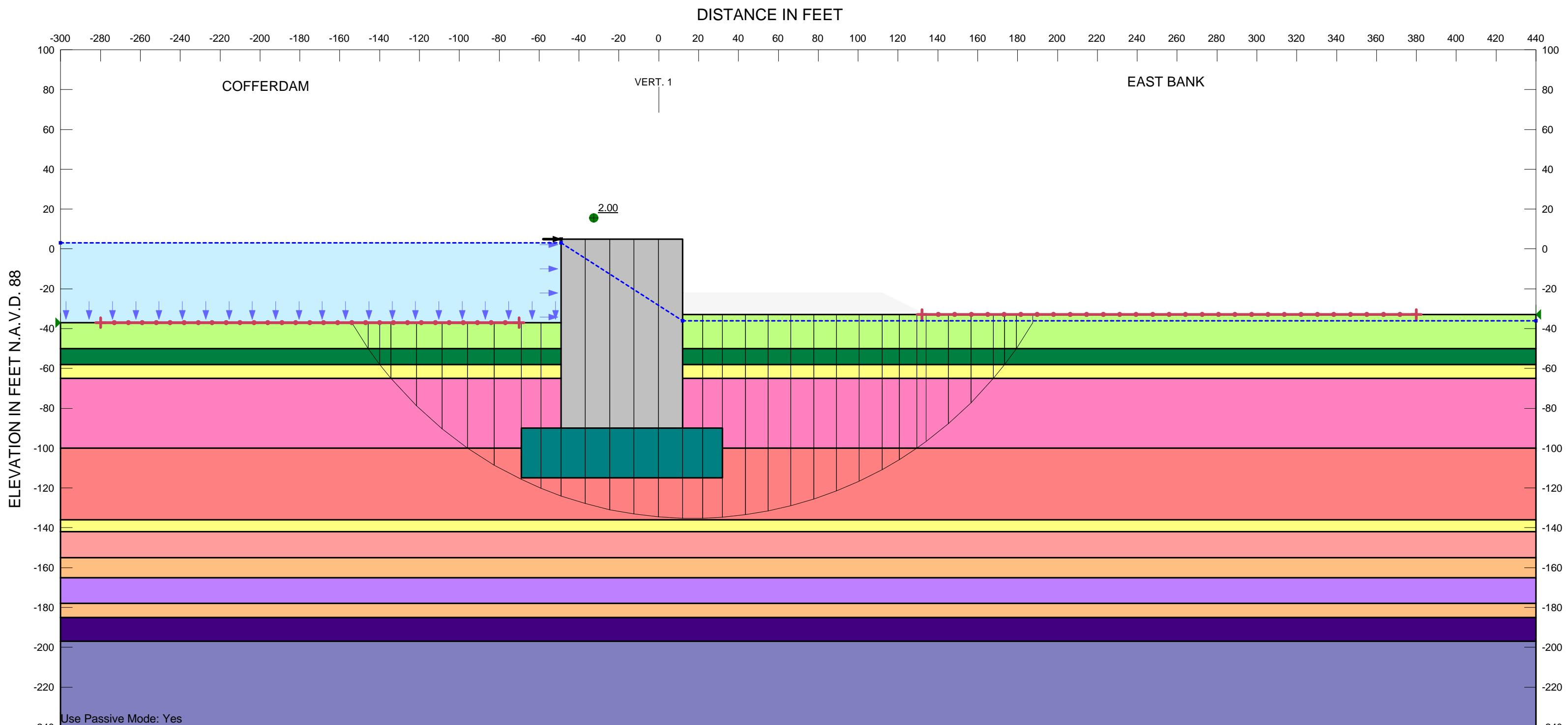
Name: CH EL. -100 TO -136 Model: Spatial Mohr-Coulomb Unit Weight: 115 pcf Cohesion: 1200 psf Phi: 0° Phi-B: 0° Piezometric Line: 1
